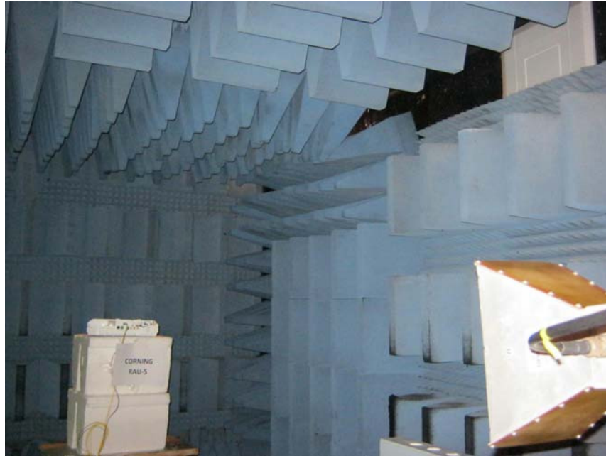
Figure 7. Radiated Emission Test
