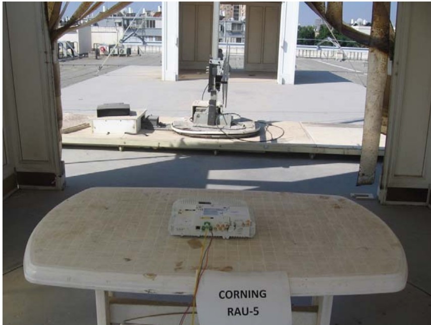
Figure 5. Radiated Emission Test
