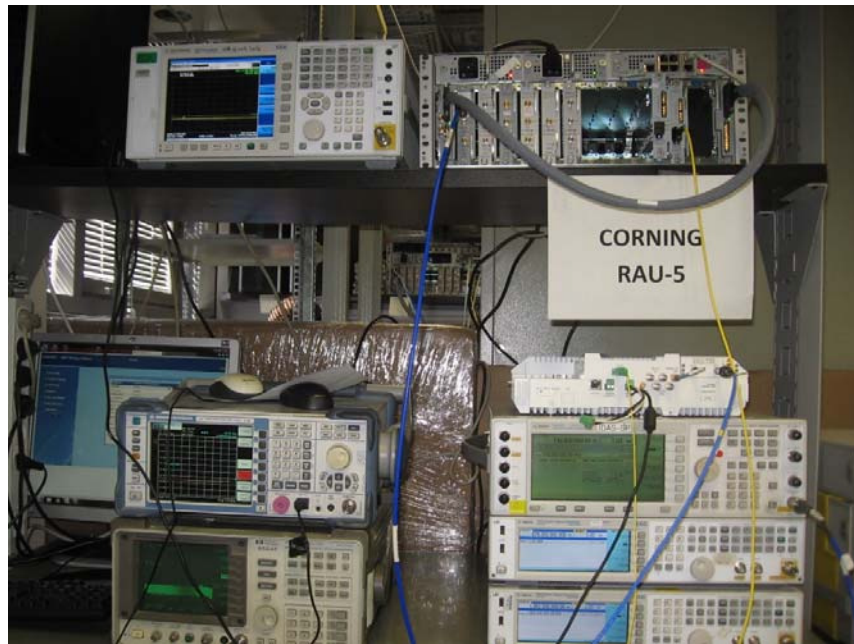
Figure 3. Conducted Emission From Antenna Port Tests
