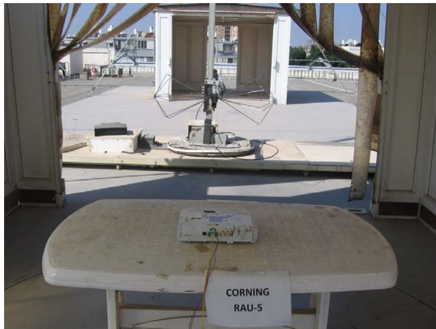
Figure 4. Radiated Emission Test
