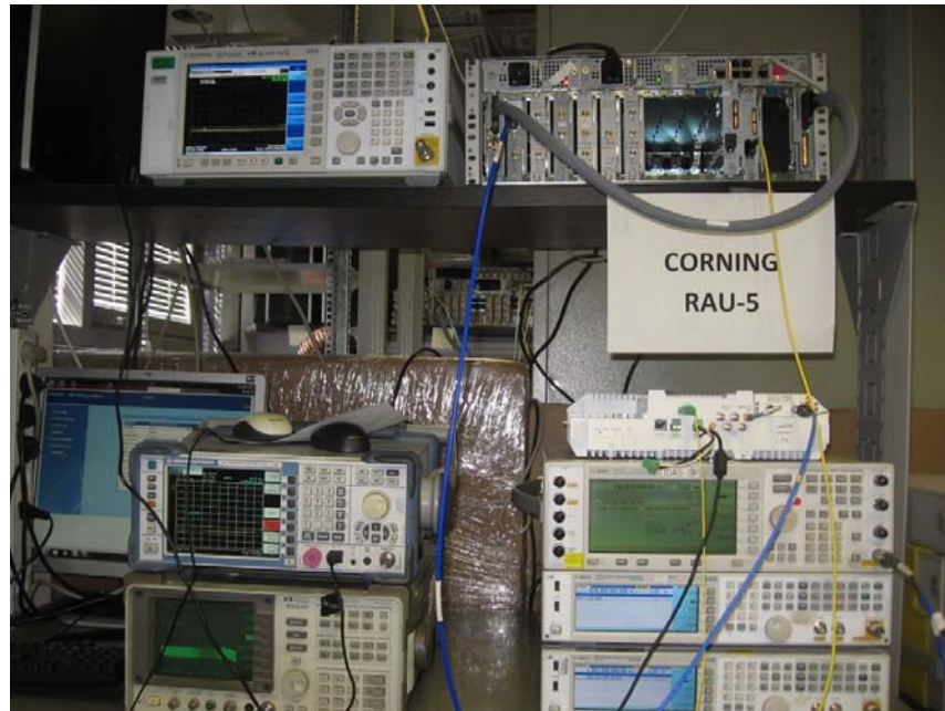
Figure 3. Conducted Emission from Antenna Ports Test
