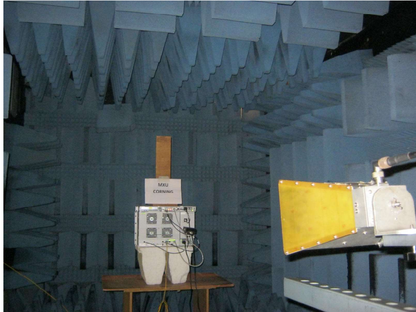
Figure 7. Radiated Emission Test Above 1GHz
