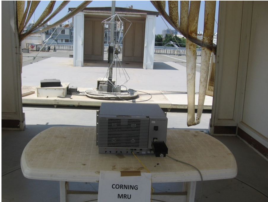
Figure 5. Radiated Emission Test 30 - 200 MHz
