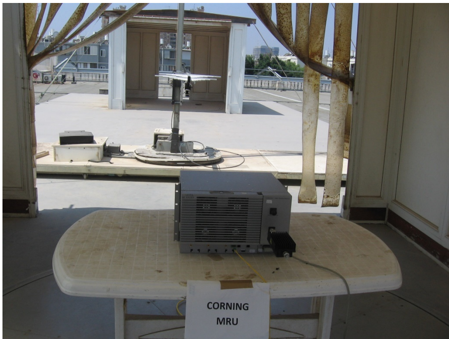
Figure 6. Radiated Emission Test 200 - 1000MHz
