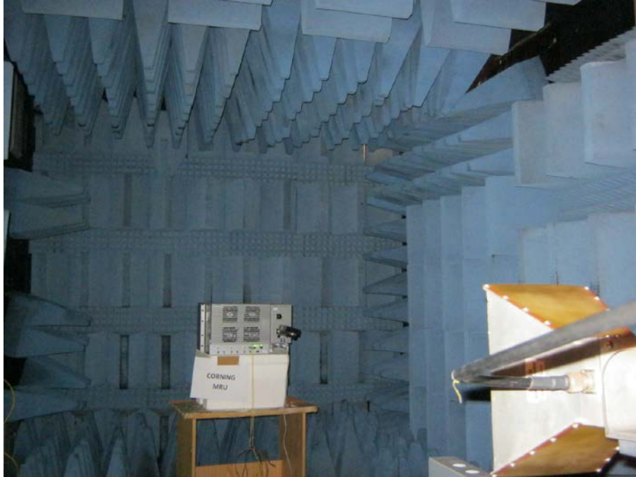
Figure 7. Radiated Emission Test 1-10GHz
