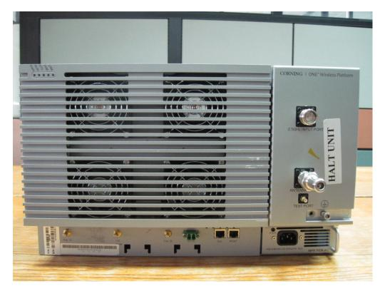
Note: The  $2.5~\mathrm{GHz}$  input connector port is currently not operational and is not to be used. It is intended for future applications.
