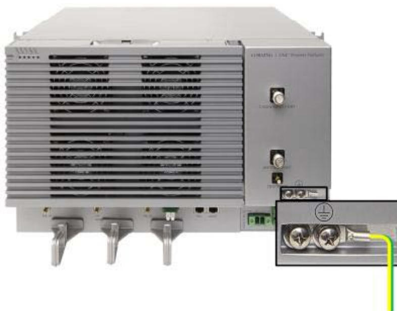
Figure 4-5. MRU Grounding Lug Connection
