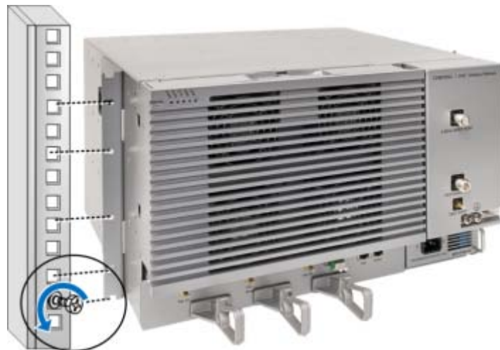
Figure 4-1 Example of MRU Chassis Rack Installation
