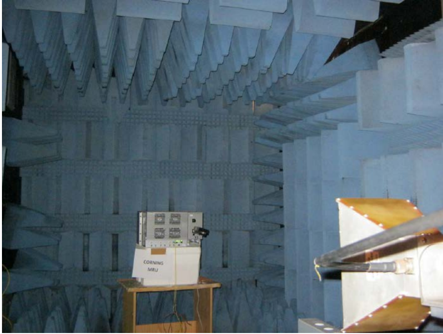
Figure 7. Radiated Emission Test 1-10GHz
