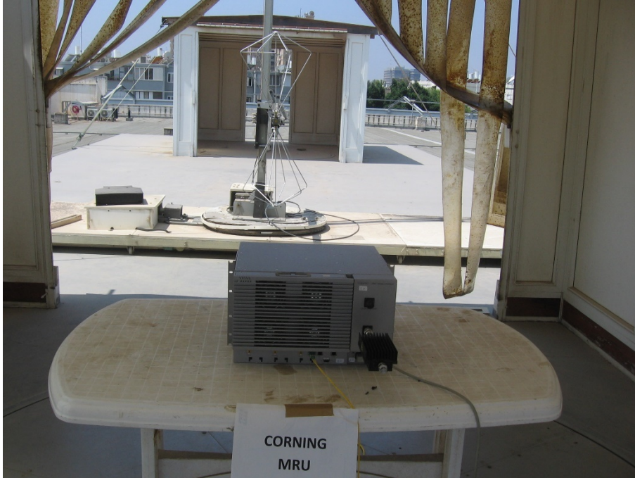
Figure 5. Radiated Emission Test 30 - 200 MHz
