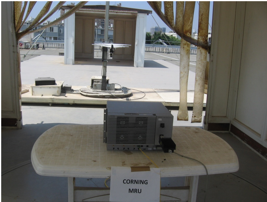
Figure 6. Radiated Emission Test 200 - 1000MHz
