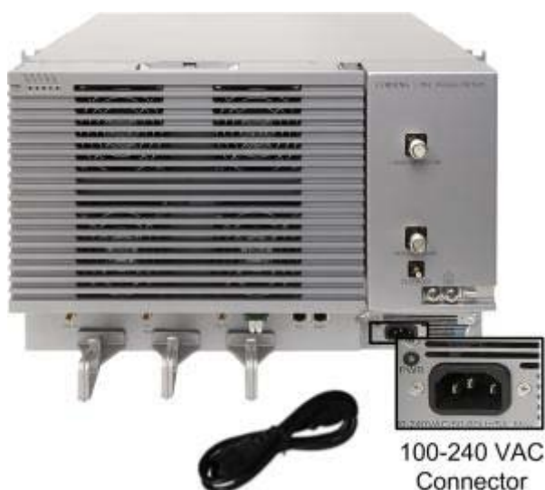
Figure 4-20. MRU AC Model Power Connector
