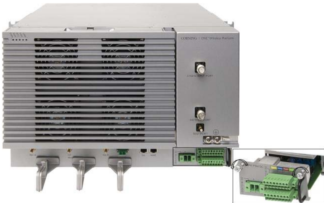
Figure 4-22. Extracting PEM from Chassis
