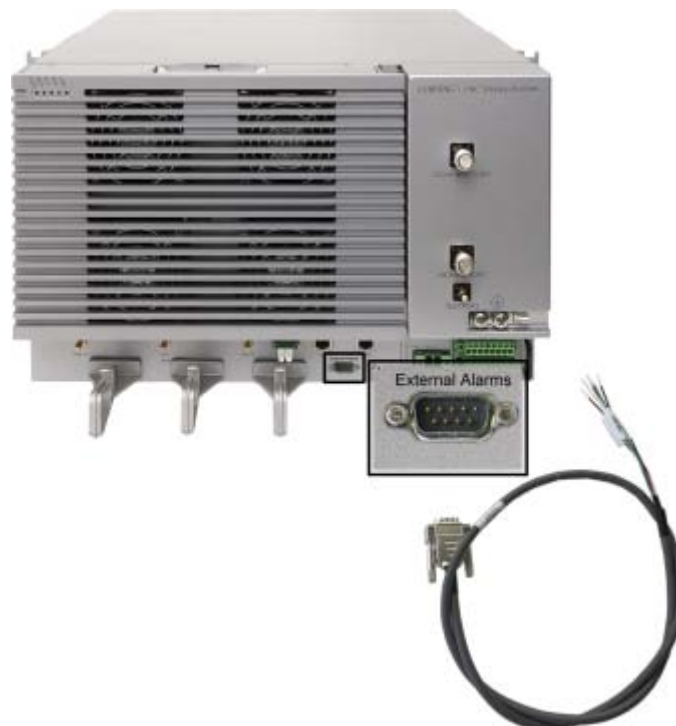
Figure 4-17. MRU External Alarms Connector and Cable
