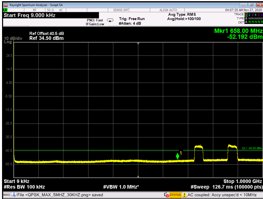
Figure 144: Spurious Emissions at Antenna Terminal 9kHz-1GHz - QPSK 5MHz B.W.; Mid, 30kHz
