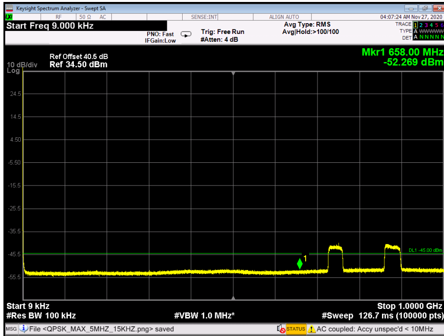
Figure 146: Spurious Emissions at Antenna Terminal 9kHz-1GHz - QPSK 5MHz B.W.; High, 30kHz
