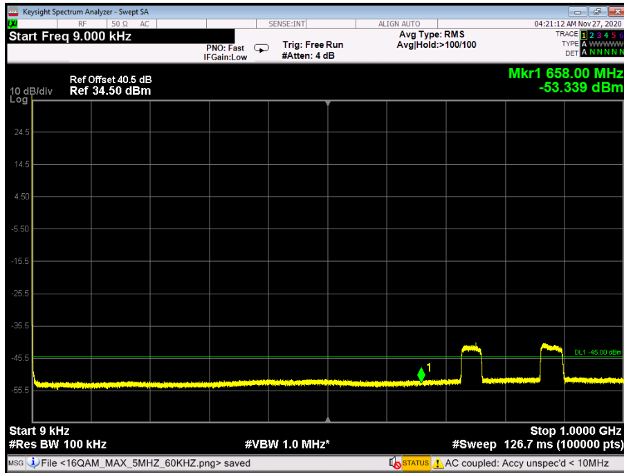
Figure 120: Spurious Emissions at Antenna Terminal 9kHz-1GHz - 16QAM 5MHz B.W.; Mid, 30kHz
