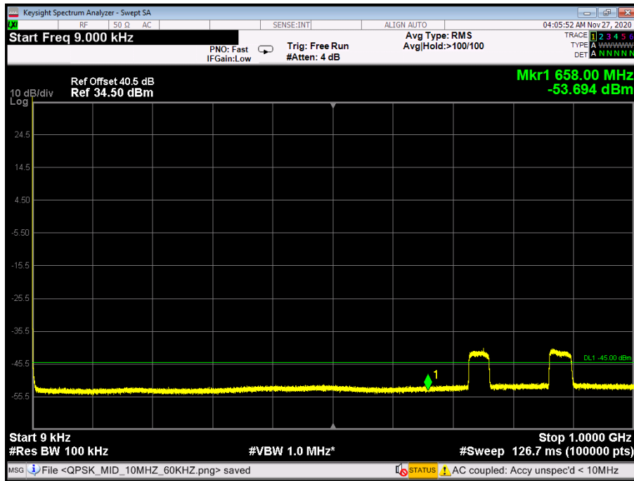
Figure 143: Spurious Emissions at Antenna Terminal 9kHz-1GHz - QPSK 5MHz B.W.; Mid, 15kHz
