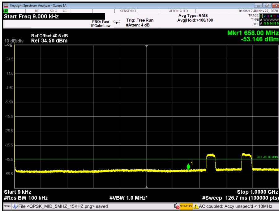
Figure 141: Spurious Emissions at Antenna Terminal 9kHz-1GHz - QPSK 5MHz B.W.; Low, 15kHz
