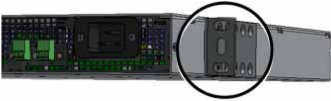
Figure 5-3. PSU6 Rack Bracket(s) for Removal
