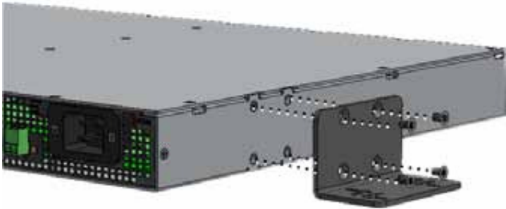
Figure 5-4. DC Assembling Wall Mount Brackets
