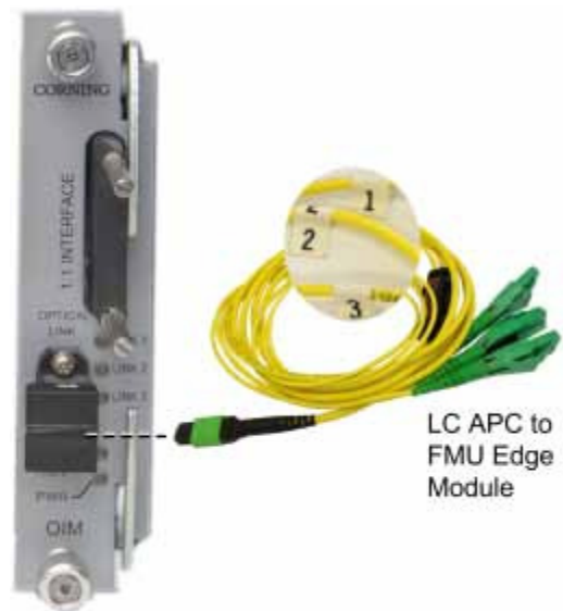
Figure 4-21. OIM Fiber Connections
