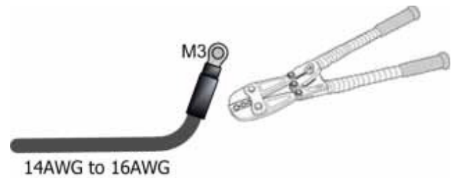
Figure 4-25. Crimping the Terminal Rings onto the DC Wire
