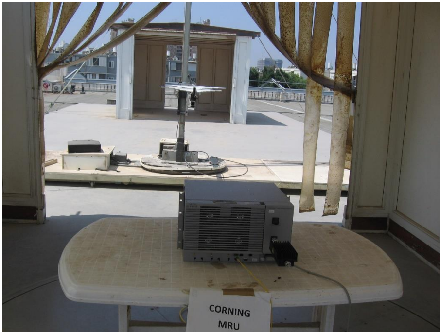
Figure 6. Radiated Emission Test
