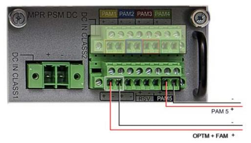
Figure 4-21. Example of CLASS2 DC Wiring Connections
