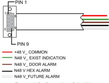
Figure 4-19. Dry Contact Alarm Cable Wiring
