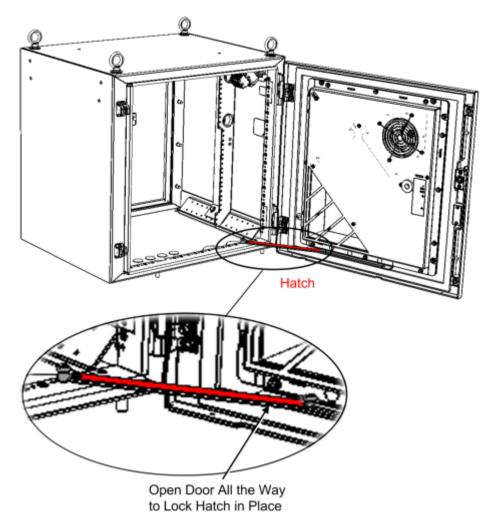
Figure 4-7. Opening Cabinet Door and Locking in Place
