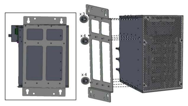
Figure 4-2. Assembling Bracket onto MRU
