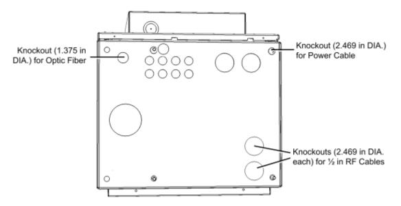
Figure 4-6. Required Knockouts Positions
