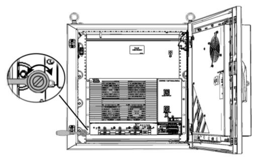
Figure 4-9. Securing MRU to Cabinet Rails
