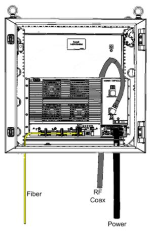
Figure 4-11. Example of Routed Connection Cables
