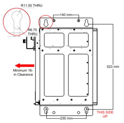
Figure 4-3. Wall-Mount Bracket Dimensions
