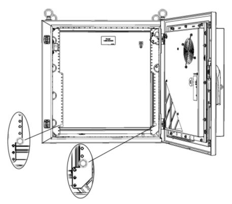
Figure 4-8. Inserting Self-Tapping Screw in each Rail
