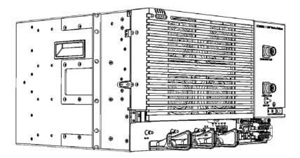
Figure 4-5. Required Position of MRU Rack Ears
