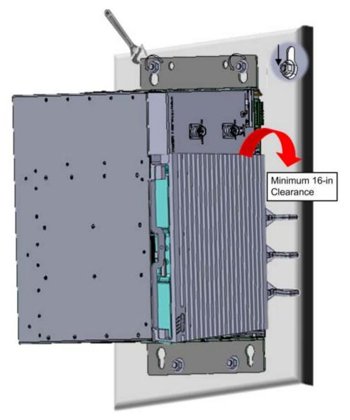
Figure 4-4. Mounting MRU on Wall
