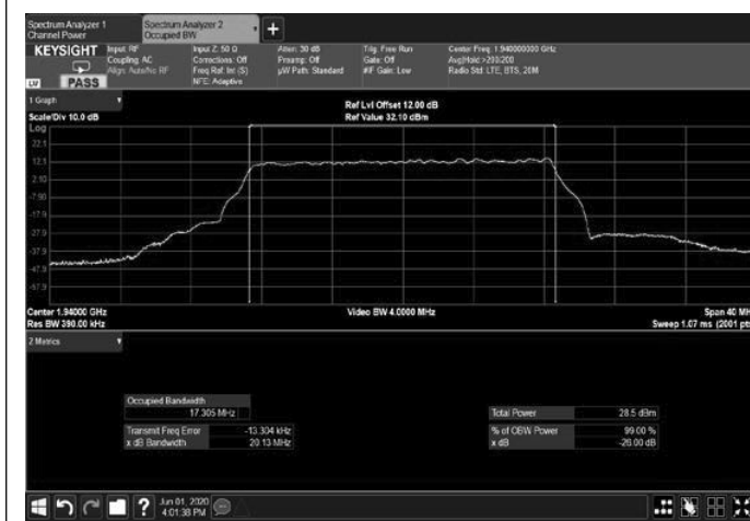
Figure 297: 256QAM 20MHz B.W.; 1940.0MHz, 60kHz Output
