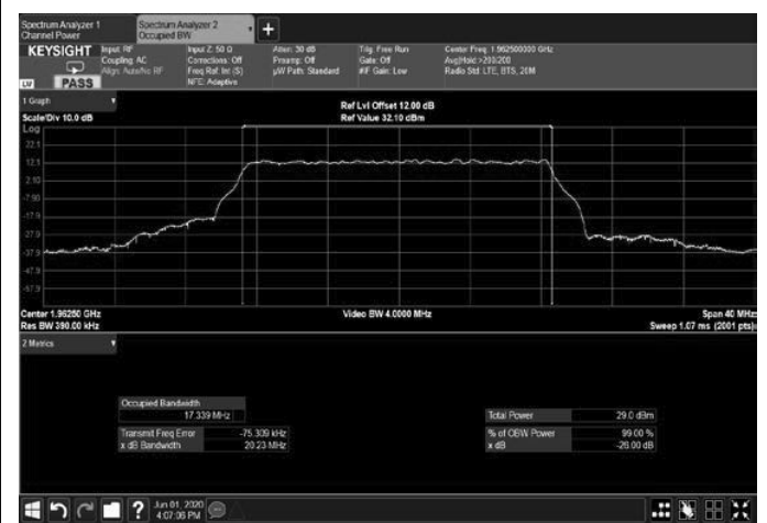
Figure 300: 256QAM 20MHz B.W.; 1962.5MHz, 60kHz Output
