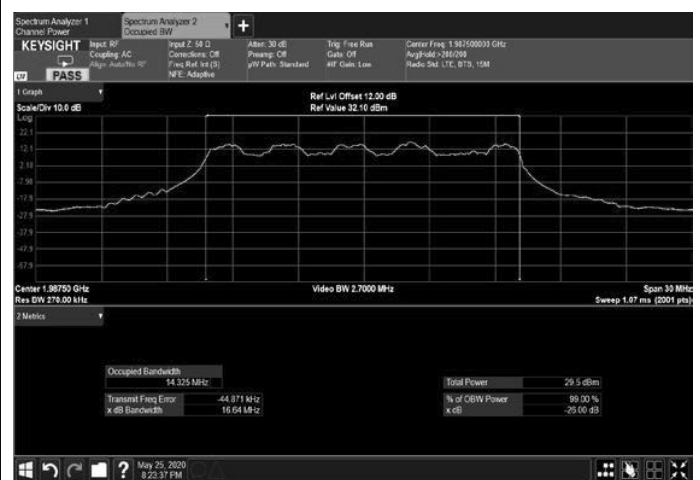
Figure 226: 16QAM 15MHz B.W.; 1987.5MHz, 15kHz Output
