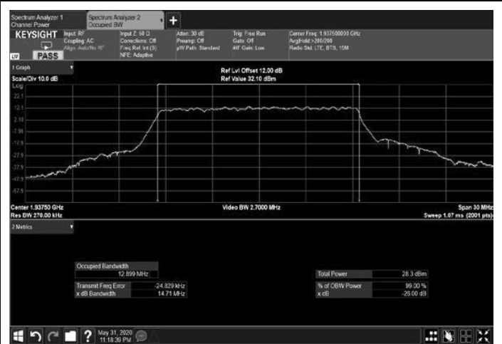
Figure 288: 256QAM 15MHz B.W.; 1937.5MHz, 60kHz Output
