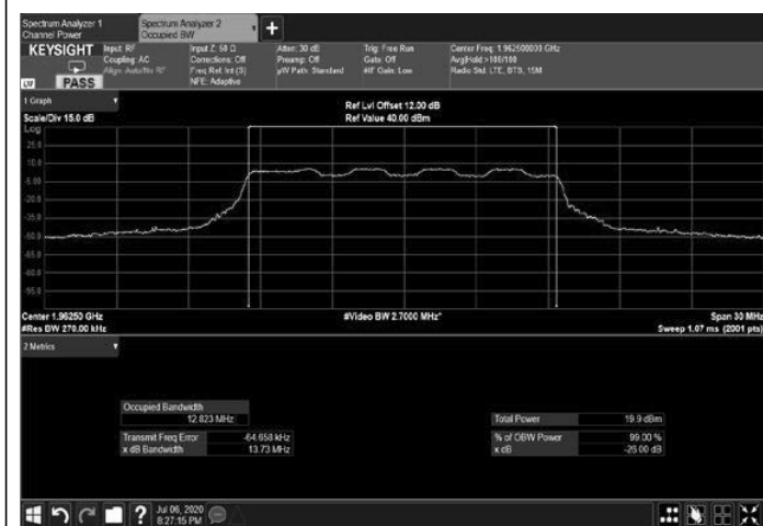
Figure 225: 16QAM 15MHz B.W.; 1962.5MHz, 60kHz Output
