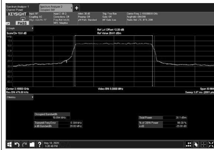
Figure 297: 256QAM 20MHz B.W.; 2155.0MHz, 15kHz Output
