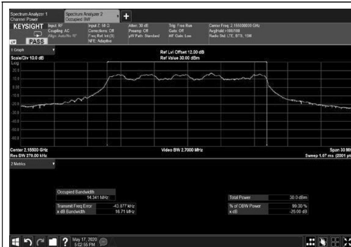
Figure 223: 16QAM 15MHz B.W.; 2155.0MHz, 15kHz Output
