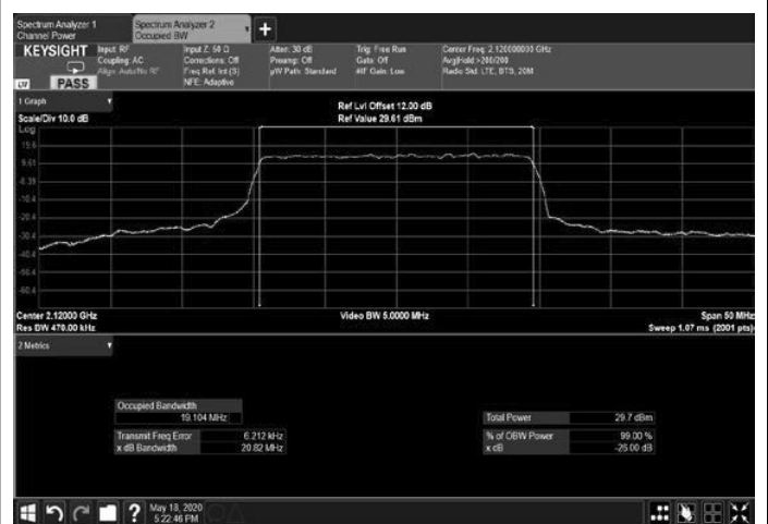
Figure 294: 256QAM 20MHz B.W.; 2120.0MHz, 15kHz Output
