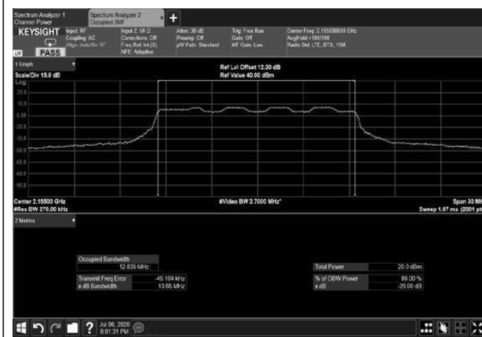
Figure 225: 16QAM 15MHz B.W.; 2155.0MHz, 60kHz Output
