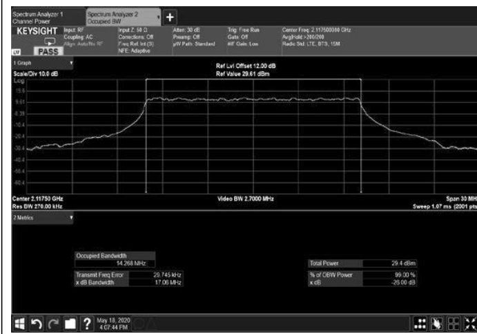
Figure 285: 256QAM 15MHz B.W.; 2117.5MHz, 15kHz Output
