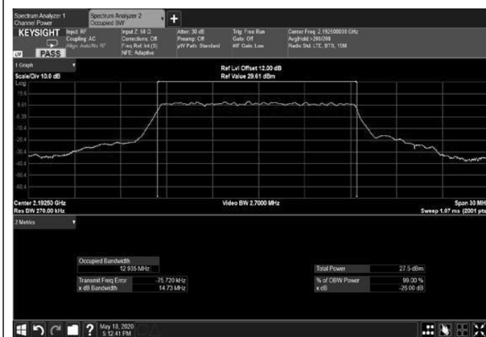
Figure 293: 256QAM 15MHz B.W.; 2192.5MHz, 60kHz Output
