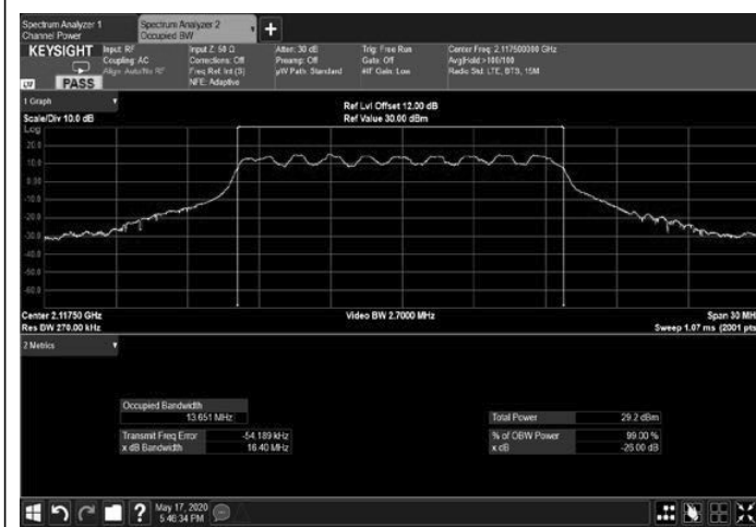
Figure 221: 16QAM 15MHz B.W.; 2117.5MHz, 30kHz Output
