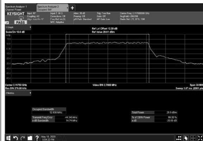
Figure 287: 256QAM 15MHz B.W.; 2117.5MHz, 60kHz Output
