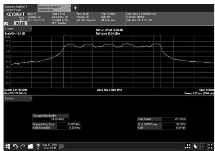
Figure 220: 16QAM 15MHz B.W.; 2117.5MHz, 15kHz Output
