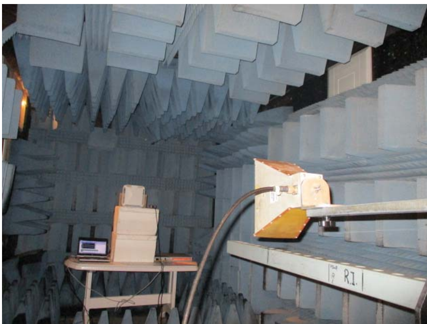
Figure 7. Radiated Emission Test, 1-18GHz
