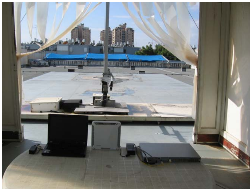
Figure 6. Radiated Emission Test, 200-1000MHz
