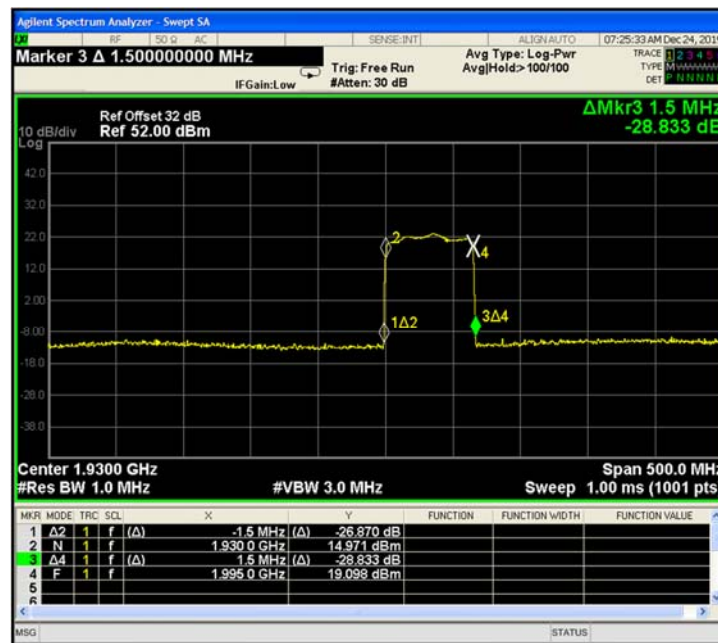
Figure 189 Out-of-Band Rejection Plot 20MHz
