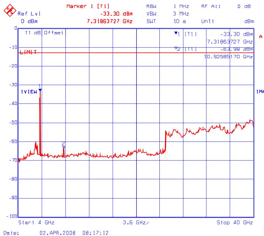
**Plot # 20(a): Transmitter Conducted Spurious Emissions**
