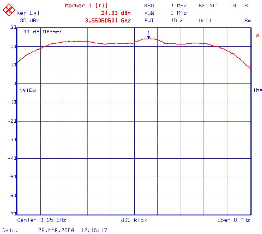
Plot # 4(b): Peak Conducted Power Density Measurement (Maximum Power Setting: 20 dBm)
