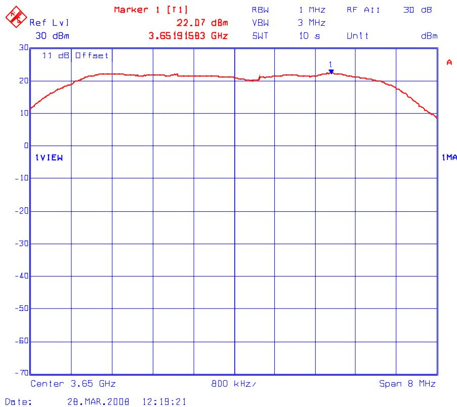
Plot # 4(d): Peak Conducted Power Density Measurement (Maximum Power Setting: 20 dBm)
