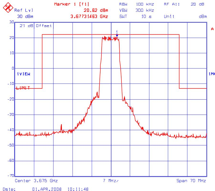
**Plot # 15(a): Transmitter Conducted Spurious Emissions**
