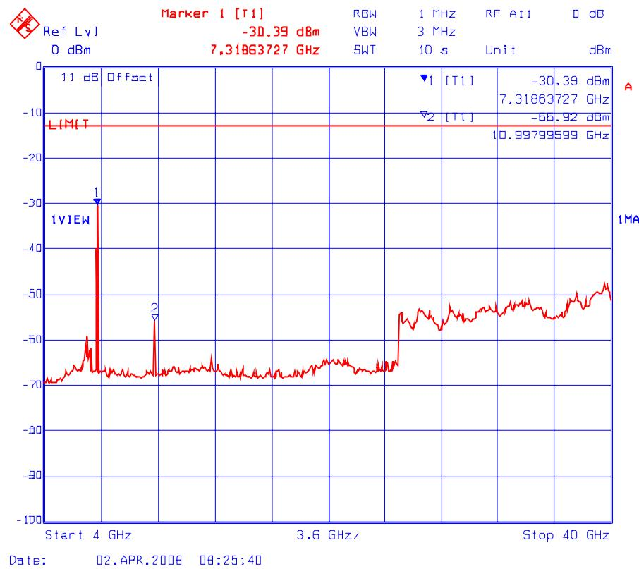
**Plot # 17(a): Transmitter Conducted Spurious Emissions**
