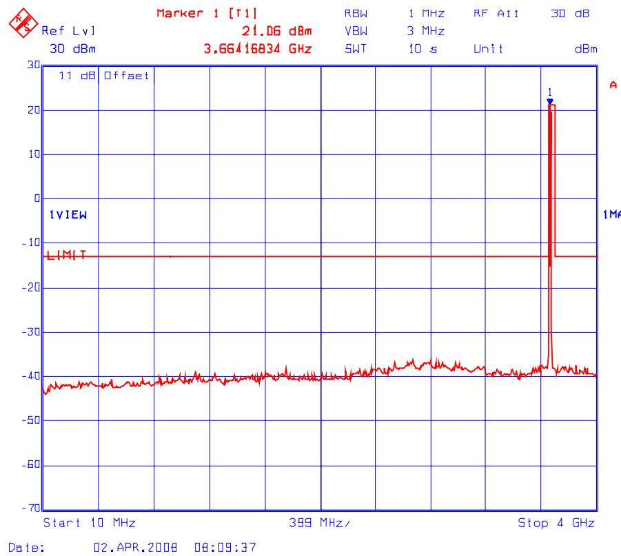
**Plot # 19(b): Transmitter Conducted Spurious Emissions**
