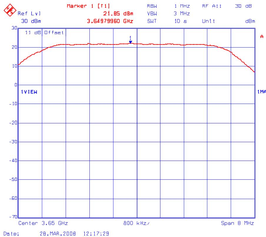
Plot # 4(c): Peak Conducted Power Density Measurement (Maximum Power Setting: 20 dBm)
