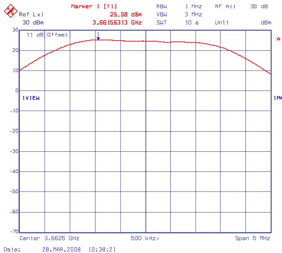
Plot # 3(a): Peak Conducted Power Density Measurement (Maximum Power Setting: 20 dBm)
