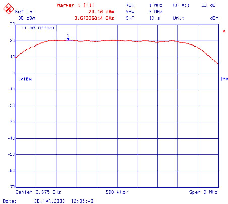
Plot # 6(c): Peak Conducted Power Density Measurement (Maximum Power Setting: 20 dBm)
