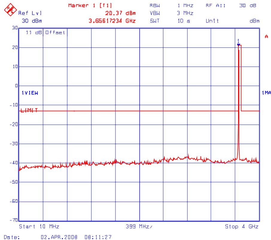
**Plot # 18(b): Transmitter Conducted Spurious Emissions**
