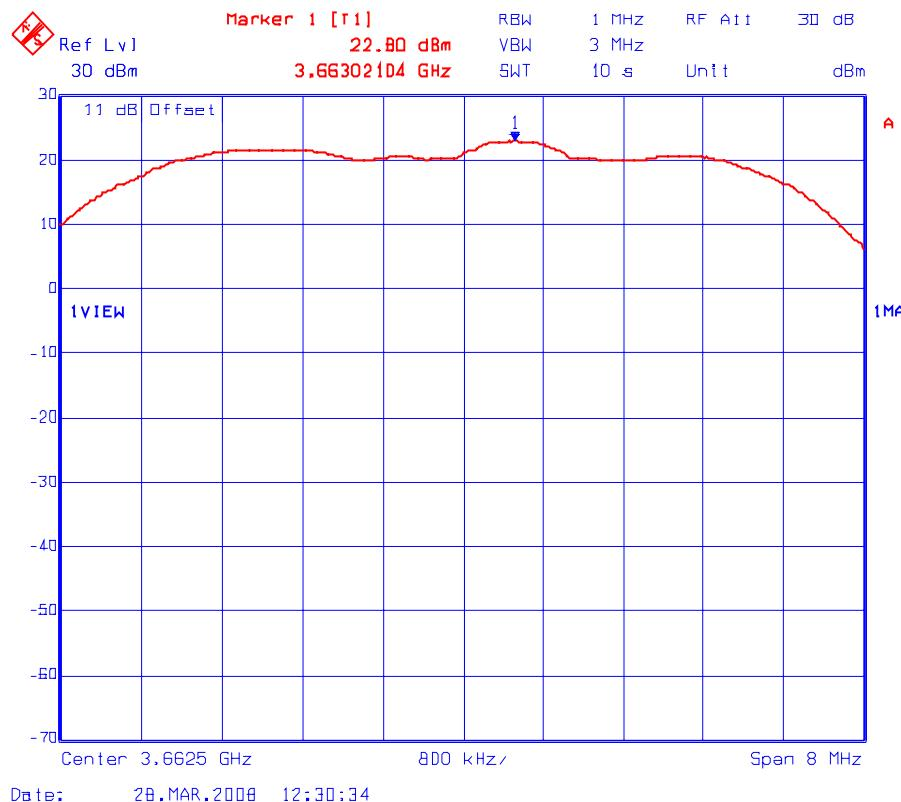
Plot # 5(c): Peak Conducted Power Density Measurement (Maximum Power Setting: 20 dBm)
