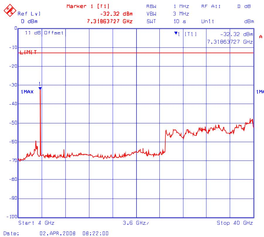
**Plot # 18(a): Transmitter Conducted Spurious Emissions**
