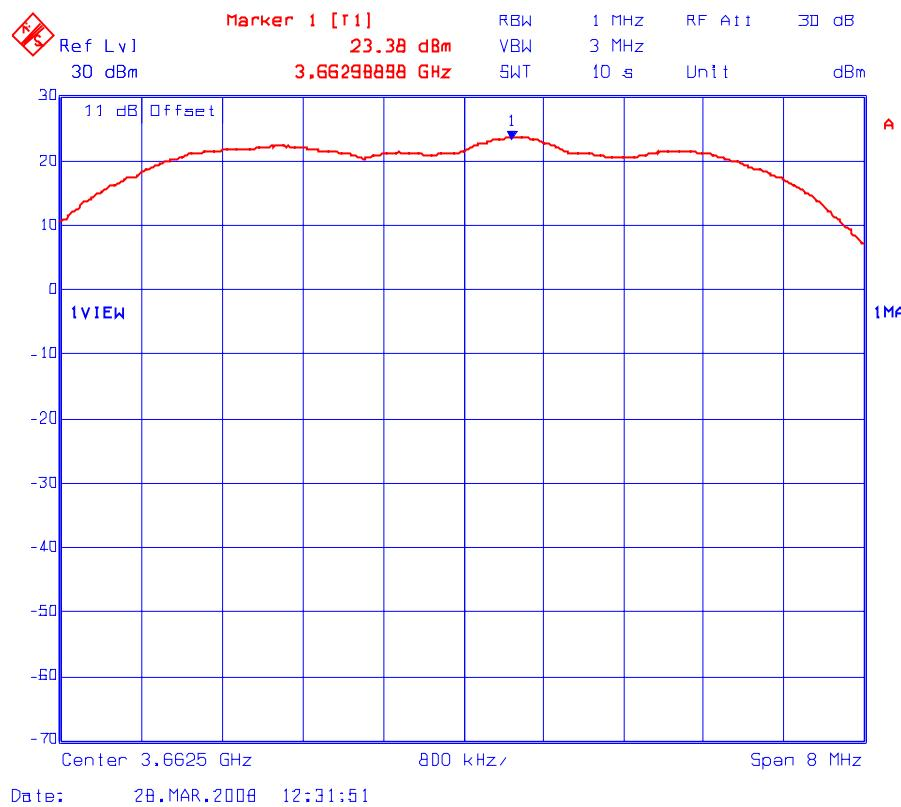
Plot # 5(b): Peak Conducted Power Density Measurement (Maximum Power Setting: 20 dBm)
