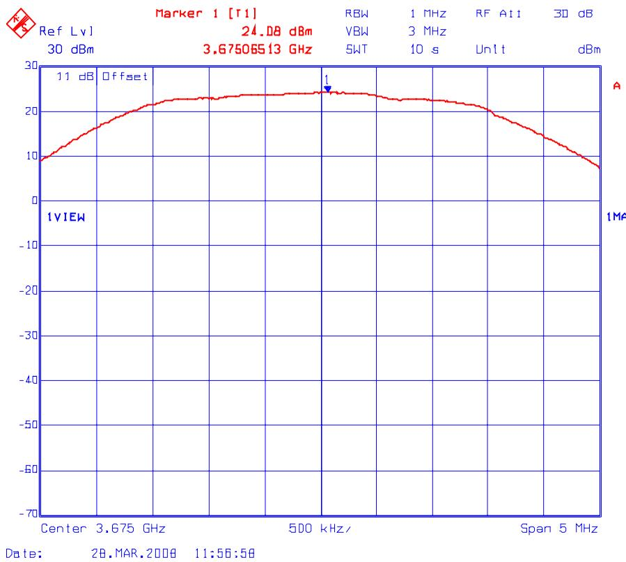
Plot # 3(d): Peak Conducted Power Density Measurement (Maximum Power Setting: 20 dBm)
