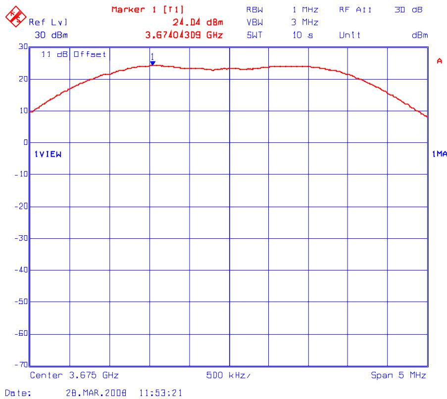
Plot # 3(b): Peak Conducted Power Density Measurement (Maximum Power Setting: 20 dBm)
