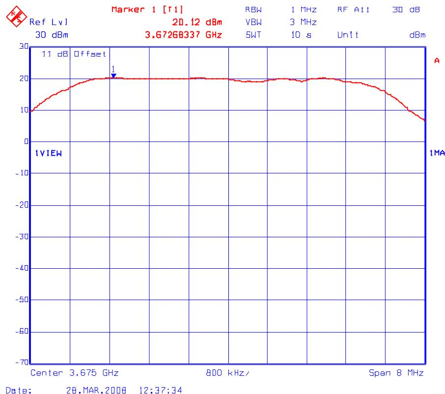
Plot # 6(d): Peak Conducted Power Density Measurement (Maximum Power Setting: 20 dBm)
