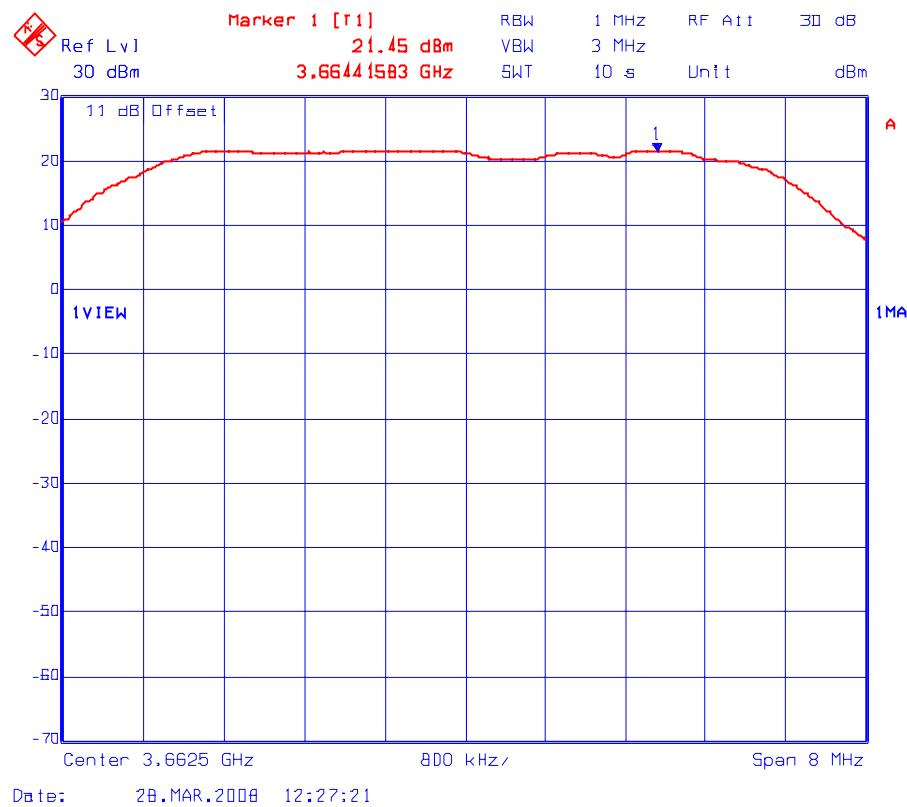
Plot # 6(a): Peak Conducted Power Density Measurement (Maximum Power Setting: 20 dBm)
