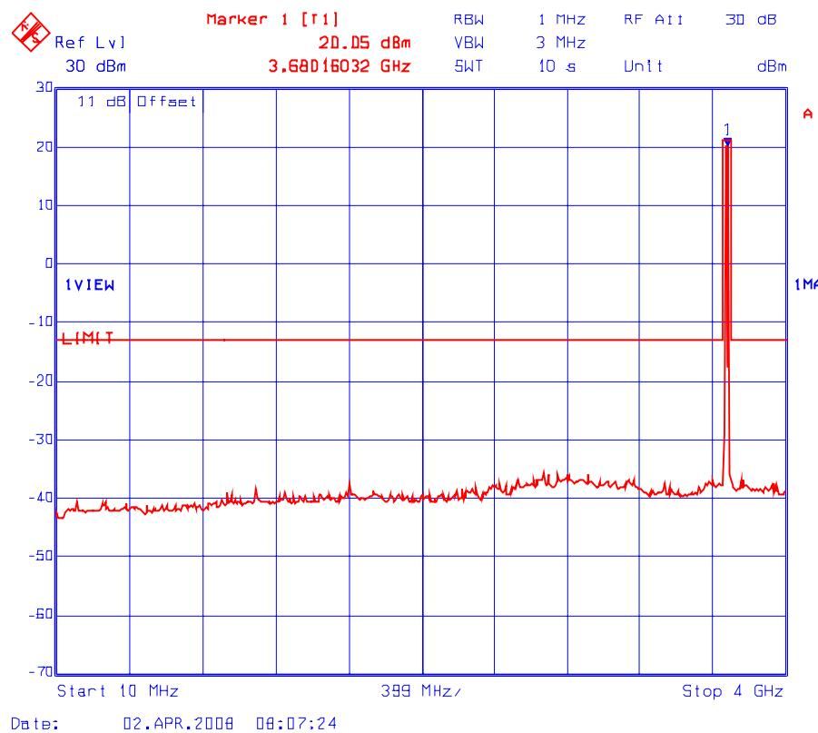
**Plot # 20(b): Transmitter Conducted Spurious Emissions**
