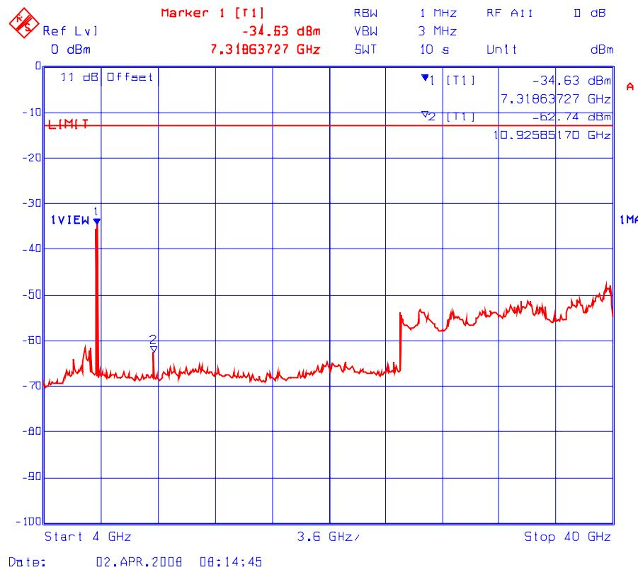
**Plot # 19(a): Transmitter Conducted Spurious Emissions**
