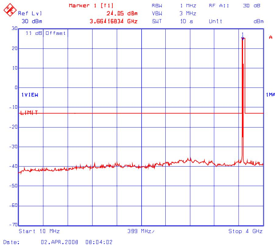
**Plot # 17(b): Transmitter Conducted Spurious Emissions**
