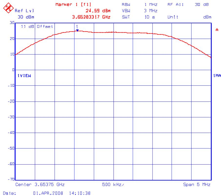
Plot # 2(a): Peak Conducted Power Density Measurement (Maximum Power Setting: 20 dBm)
