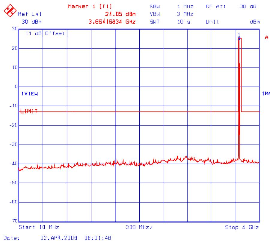
**Plot # 16(b): Transmitter Conducted Spurious Emissions**
