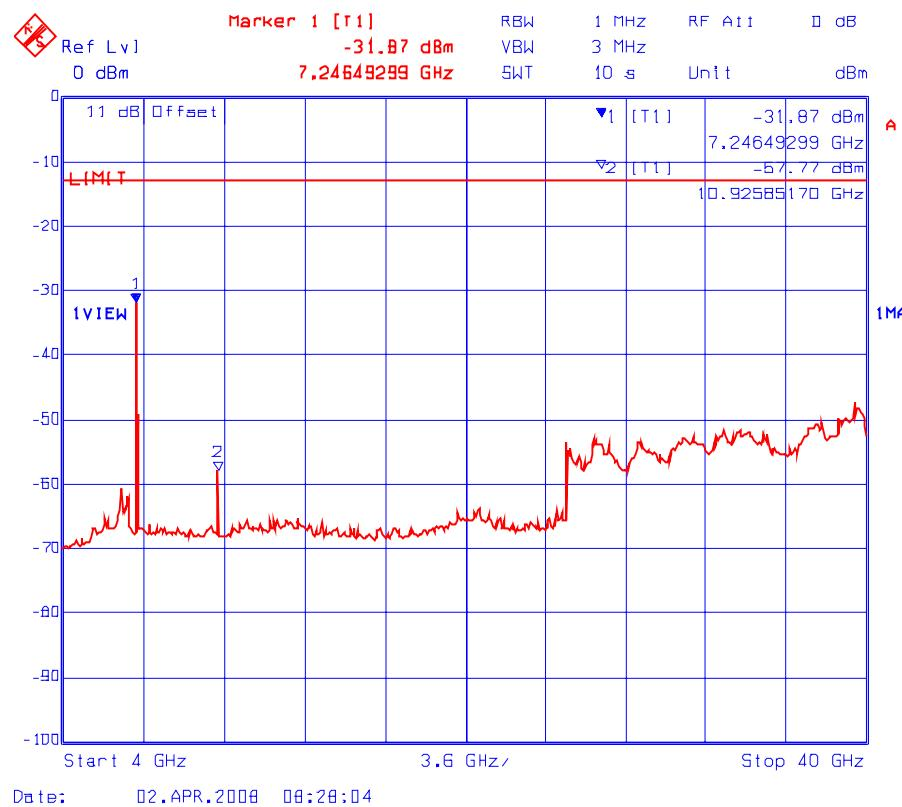
**Plot # 16(a): Transmitter Conducted Spurious Emissions**
