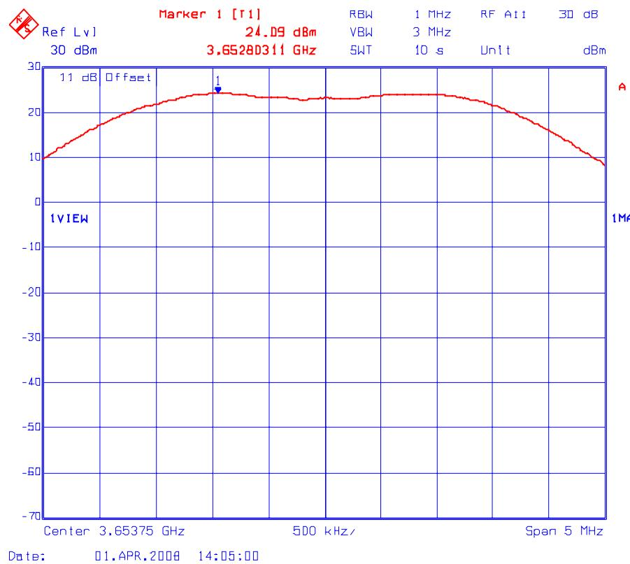
Plot # 1(b): Peak Conducted Power Density Measurement (Maximum Power Setting: 20 dBm)
