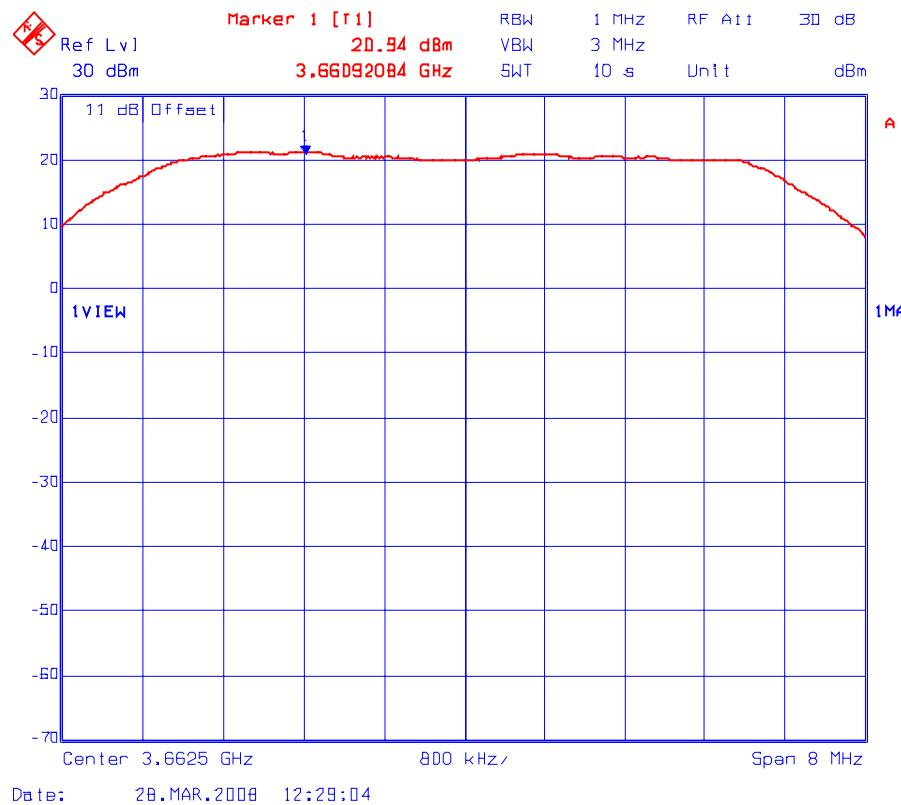
Plot # 5(d): Peak Conducted Power Density Measurement (Maximum Power Setting: 20 dBm)
