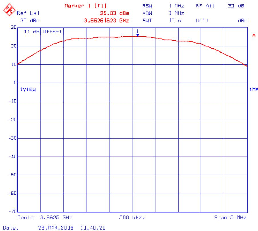
Plot # 2(d): Peak Conducted Power Density Measurement (Maximum Power Setting: 20 dBm)
