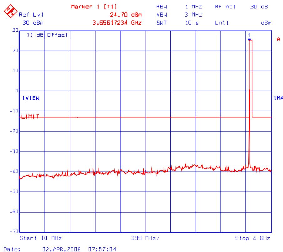
**Plot # 15(b): Transmitter Conducted Spurious Emissions**
