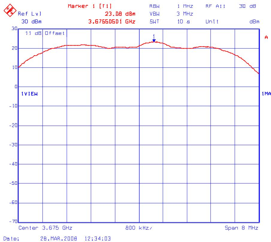
Plot # 6(b): Peak Conducted Power Density Measurement (Maximum Power Setting: 20 dBm)
