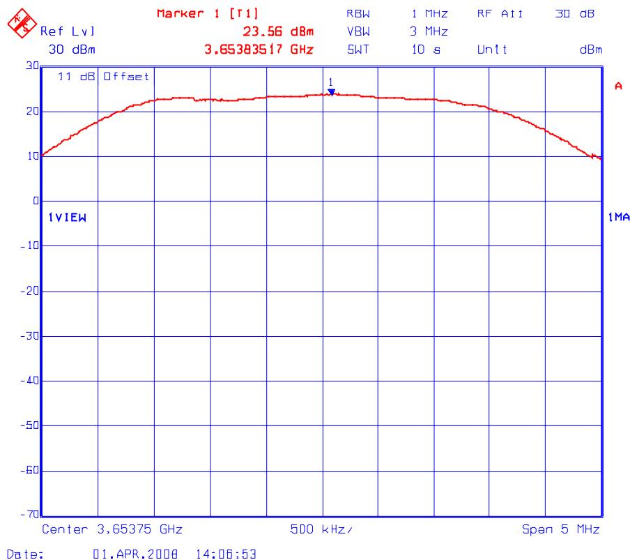
Plot # 1(c): Peak Conducted Power Density Measurement (Maximum Power Setting: 20 dBm)
