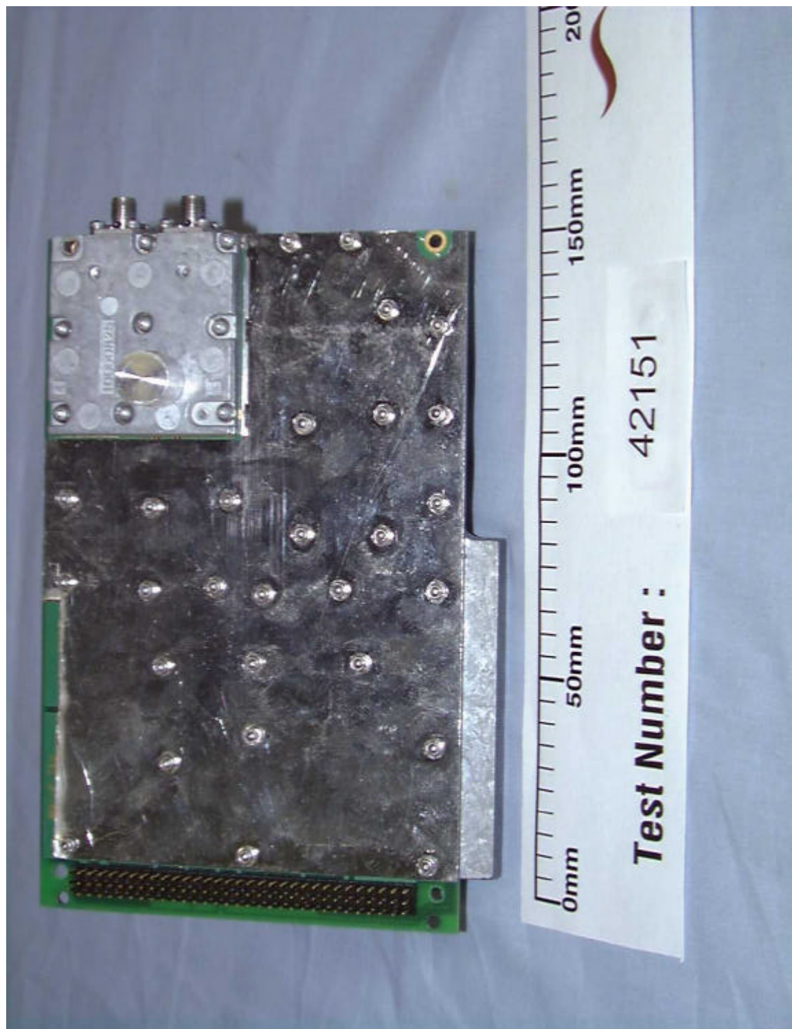
PHT/42151SUPB/001 Bottom view of transceiver module.
