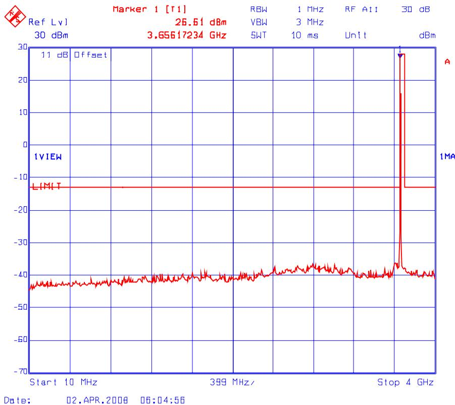
**Plot # 15(b): Transmitter Conducted Spurious Emissions**
