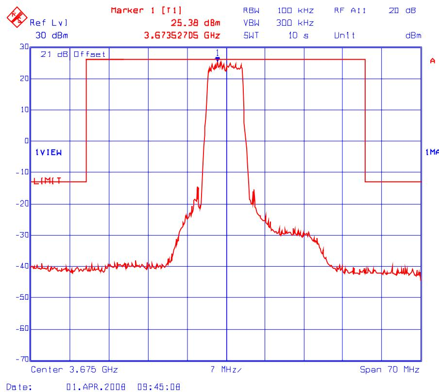
**Plot # 15(a): Transmitter Conducted Spurious Emissions**
