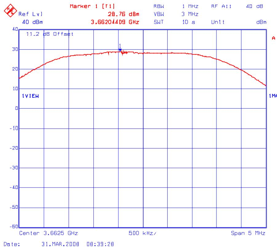
Plot # 2(c): Peak Conducted Power Density Measurement (Maximum Power Setting: 23 dBm)
