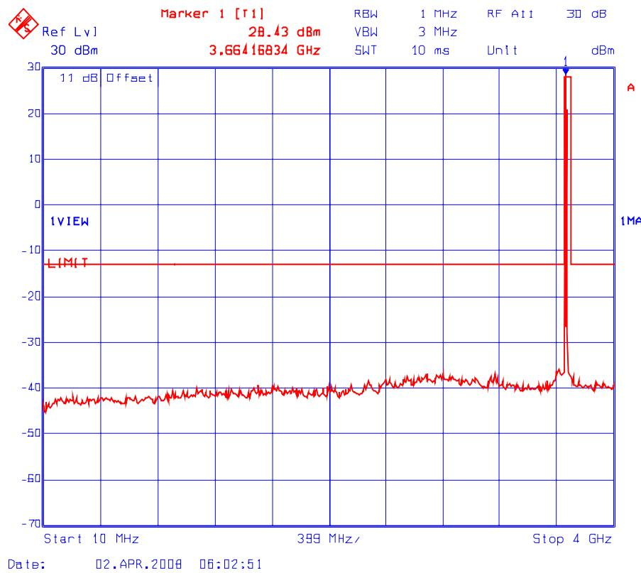
**Plot # 16(b): Transmitter Conducted Spurious Emissions**
