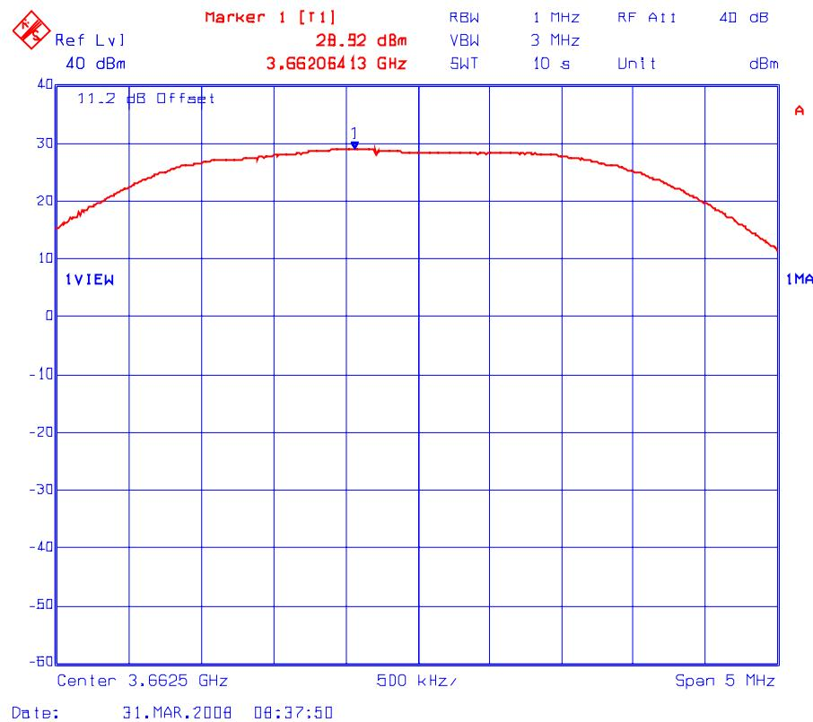
Plot # 2(d): Peak Conducted Power Density Measurement (Maximum Power Setting: 23 dBm)
