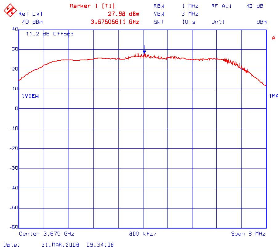
Plot # 6(b): Peak Conducted Power Density Measurement (Maximum Power Setting: 23 dBm)
