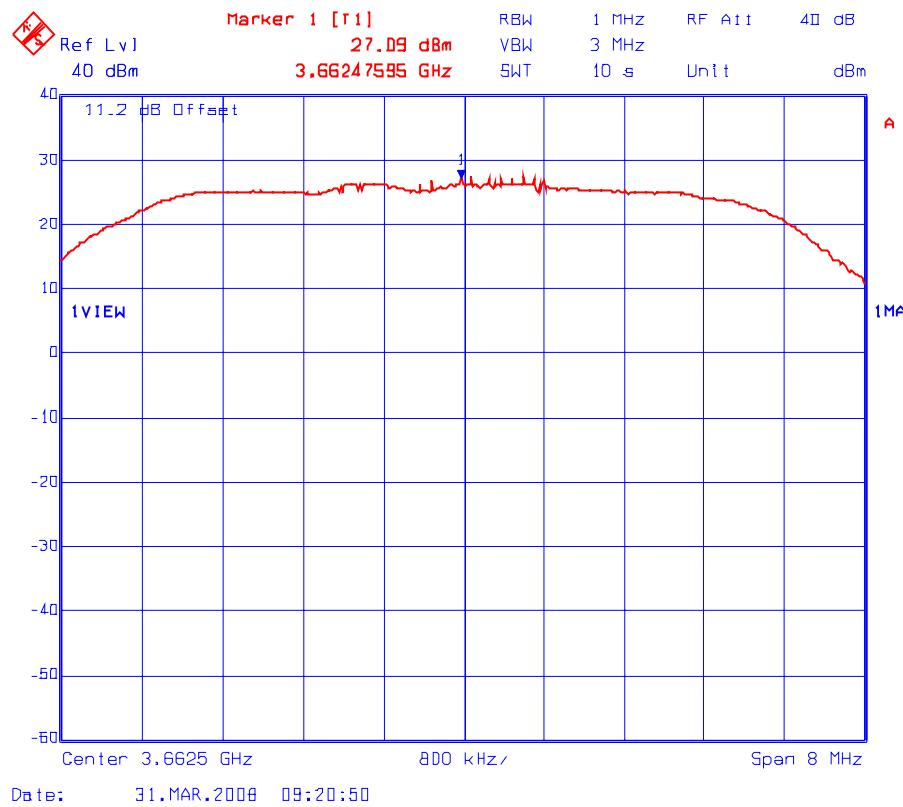
Plot # 5(c): Peak Conducted Power Density Measurement (Maximum Power Setting: 23 dBm)
