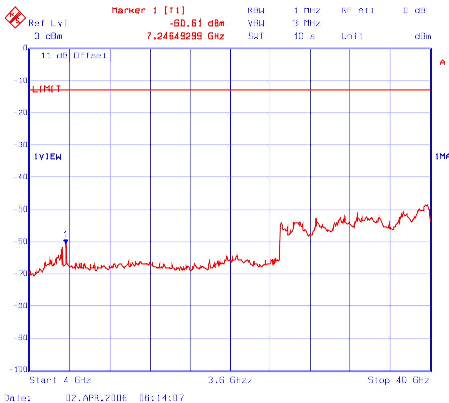
**Plot # 16(a): Transmitter Conducted Spurious Emissions**
