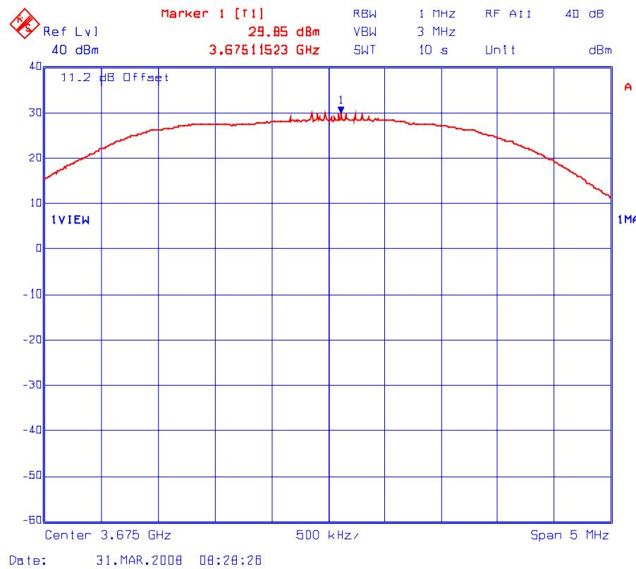
Plot # 4(a): Peak Conducted Power Density Measurement (Maximum Power Setting: 23 dBm)
