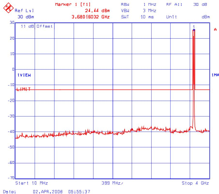
**Plot # 20(b): Transmitter Conducted Spurious Emissions**
