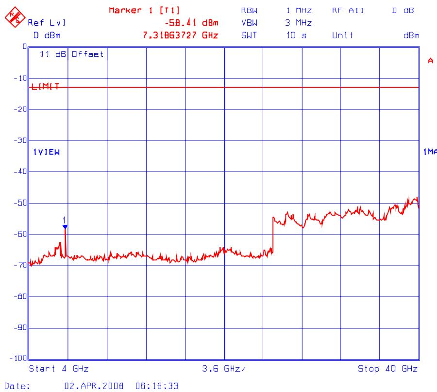
**Plot # 18(a): Transmitter Conducted Spurious Emissions**
