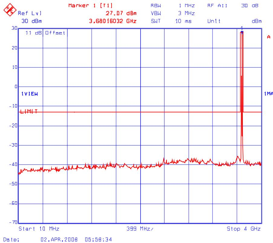
**Plot # 17(b): Transmitter Conducted Spurious Emissions**
