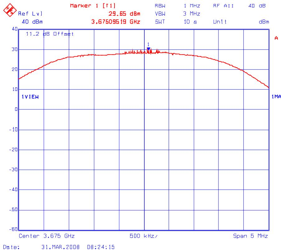
Plot # 3(b): Peak Conducted Power Density Measurement (Maximum Power Setting: 23 dBm)
