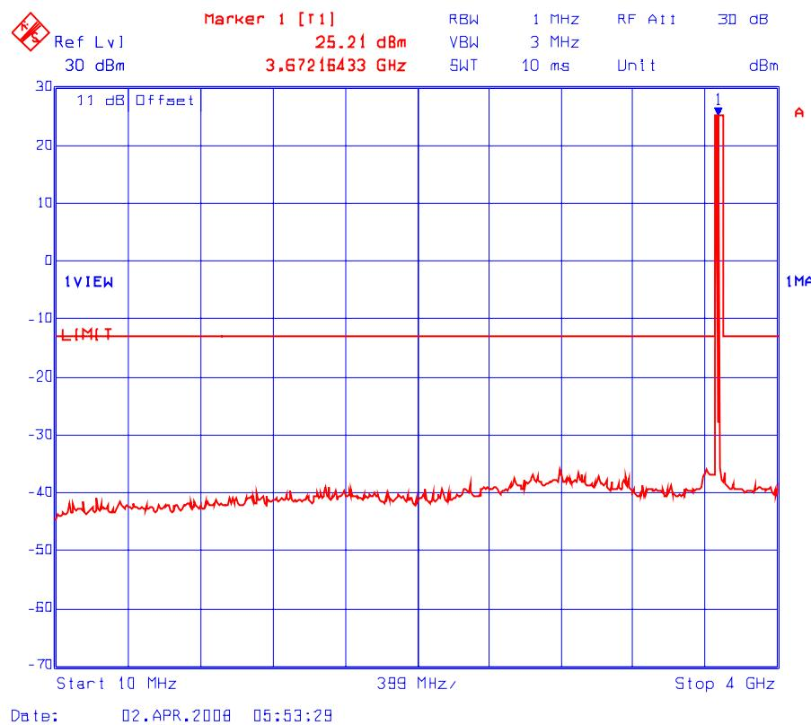
**Plot # 19(b): Transmitter Conducted Spurious Emissions**
