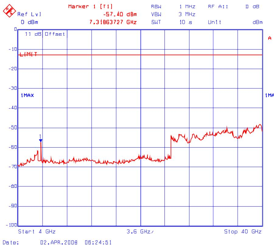
**Plot # 20(a): Transmitter Conducted Spurious Emissions**
