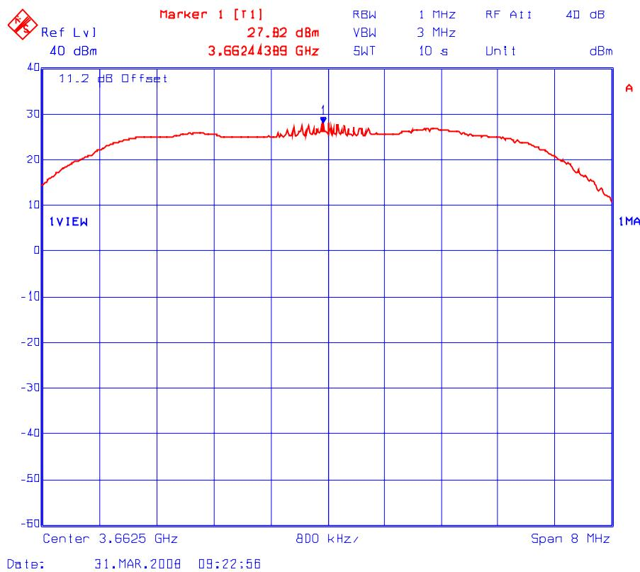
Plot # 5(d): Peak Conducted Power Density Measurement (Maximum Power Setting: 23 dBm)
