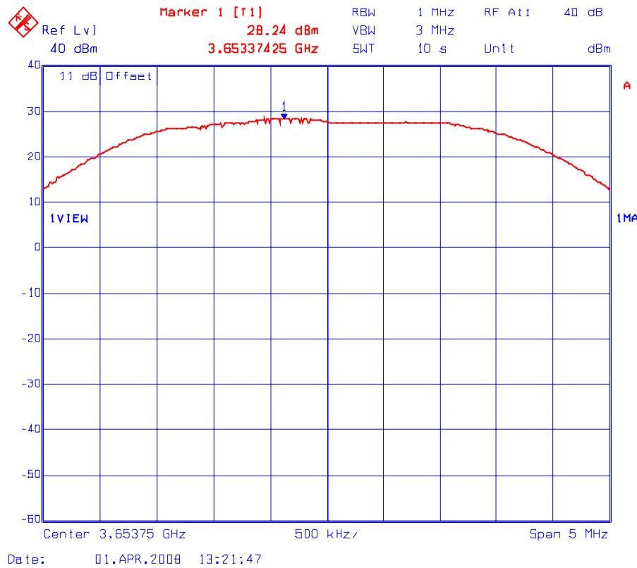
Plot # 1(d): Peak Conducted Power Density Measurement (Maximum Power Setting: 23 dBm)
