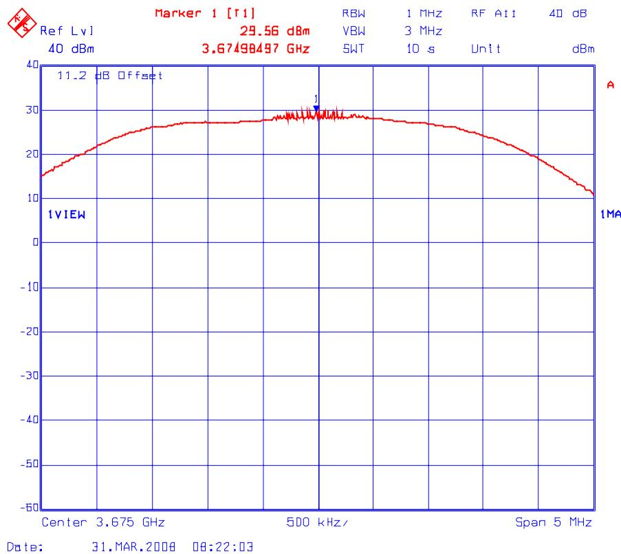
Plot # 3(c): Peak Conducted Power Density Measurement (Maximum Power Setting: 23 dBm)
