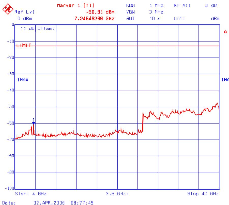
**Plot # 19(a): Transmitter Conducted Spurious Emissions**
