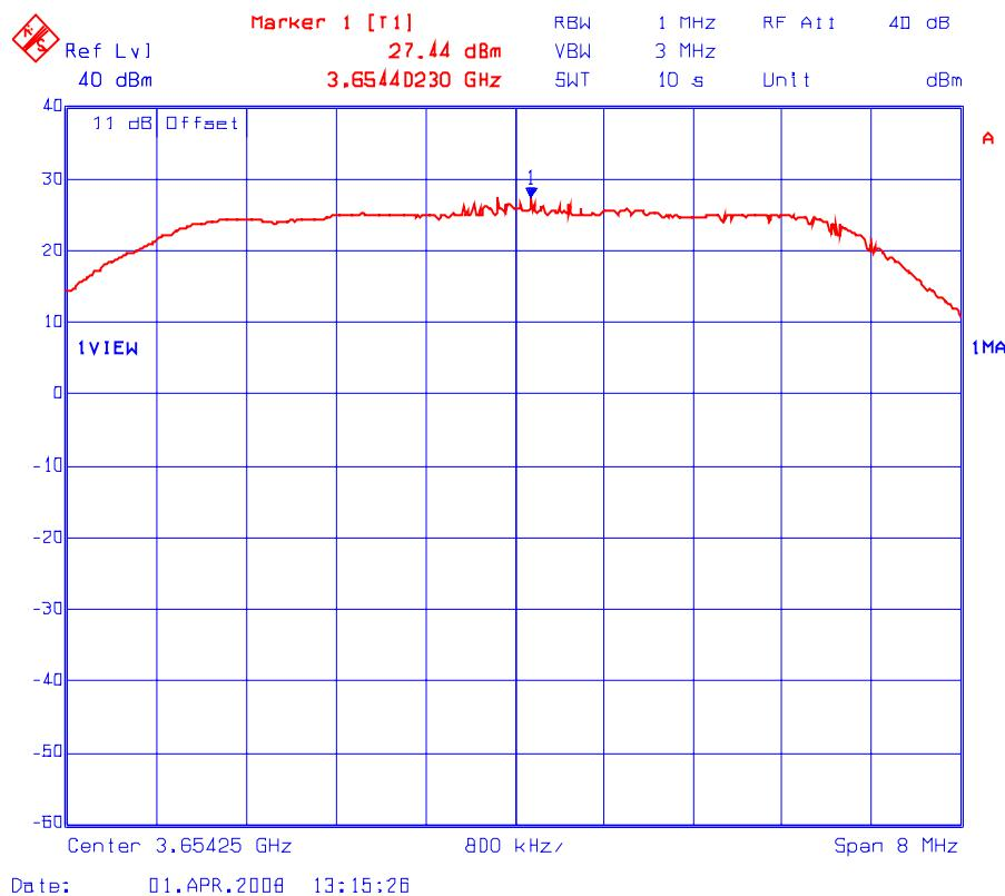
Plot # 4(b): Peak Conducted Power Density Measurement (Maximum Power Setting: 23 dBm)
