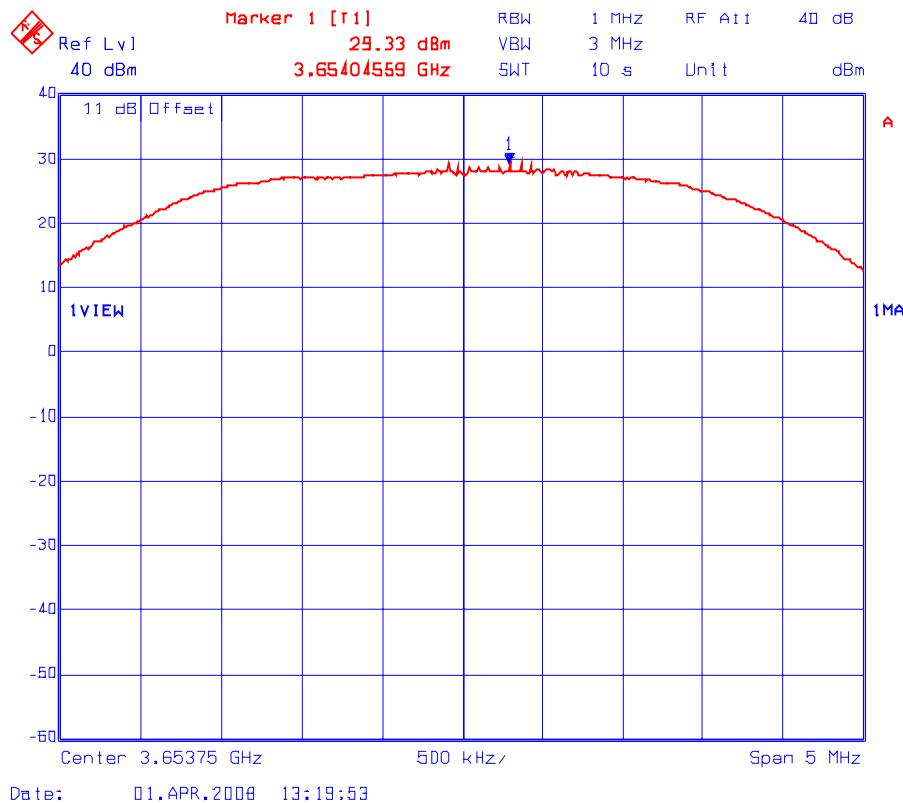
Plot # 1(c): Peak Conducted Power Density Measurement (Maximum Power Setting: 23 dBm)
