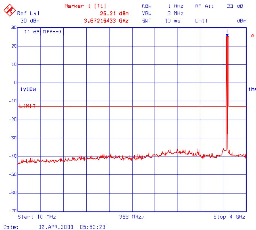
**Plot # 19(b): Transmitter Conducted Spurious Emissions**
