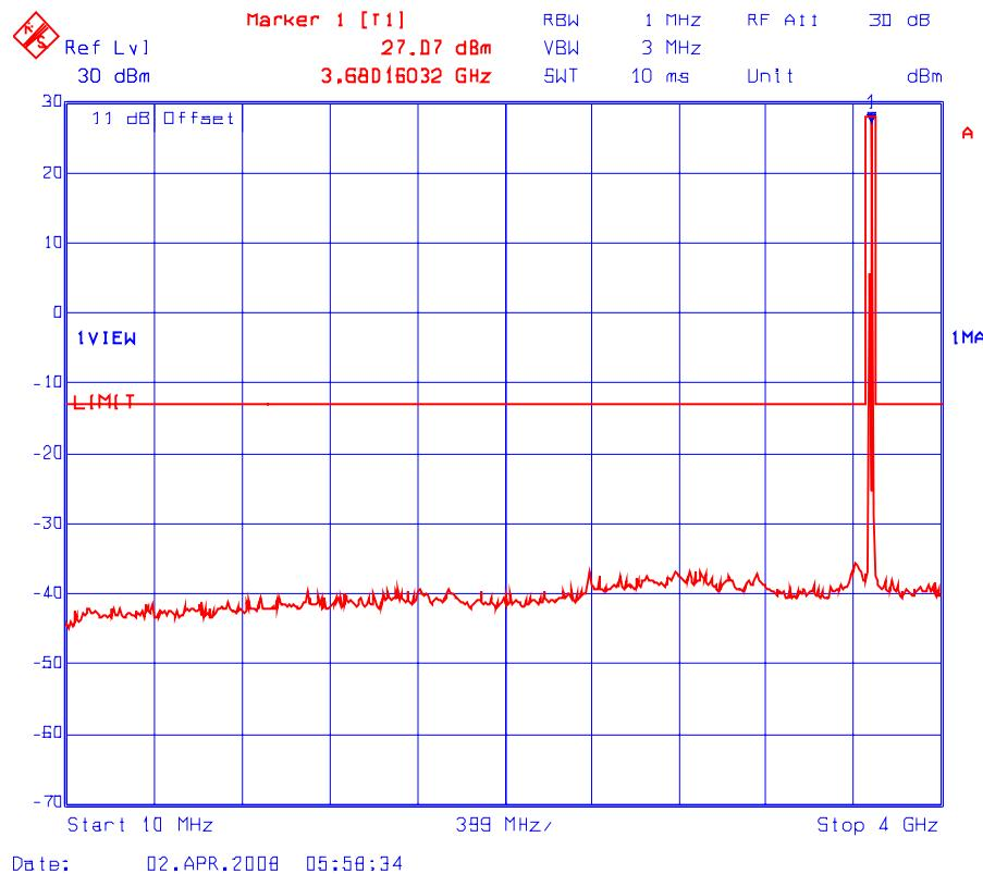
**Plot # 17(b): Transmitter Conducted Spurious Emissions**
