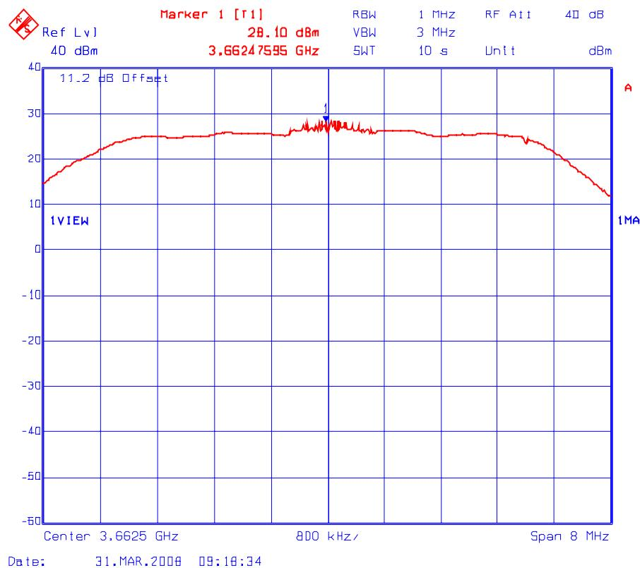
Plot # 5(b): Peak Conducted Power Density Measurement (Maximum Power Setting: 23 dBm)
