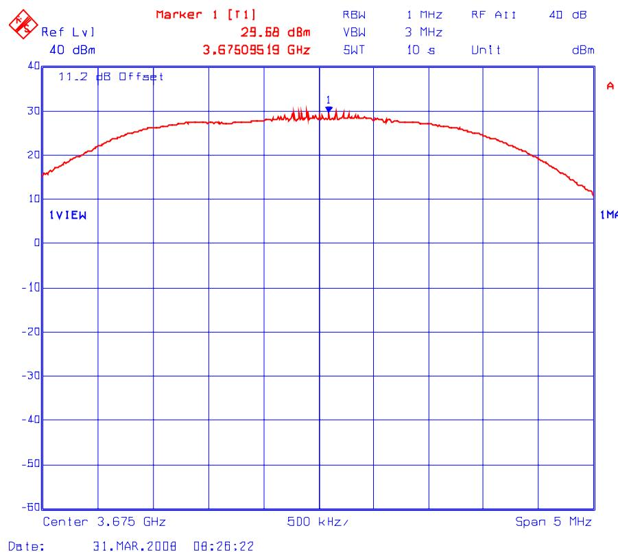
Plot # 3(d): Peak Conducted Power Density Measurement (Maximum Power Setting: 23 dBm)
