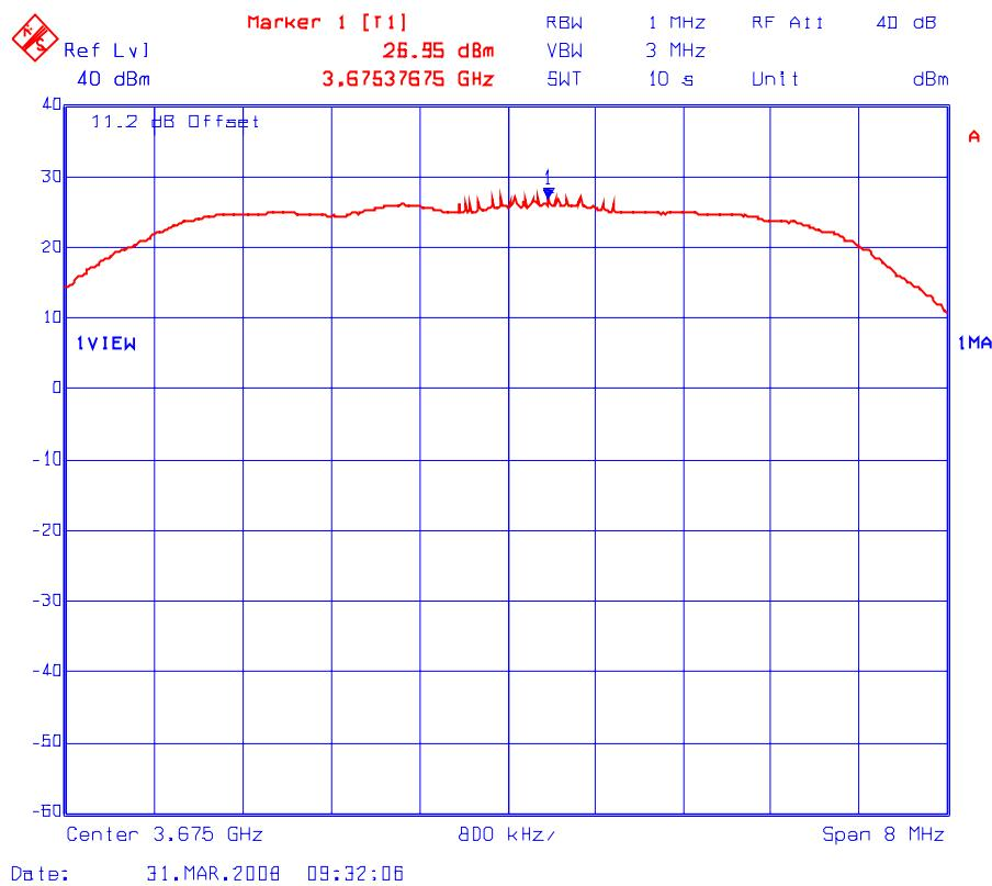
Plot # 6(c): Peak Conducted Power Density Measurement (Maximum Power Setting: 23 dBm)
