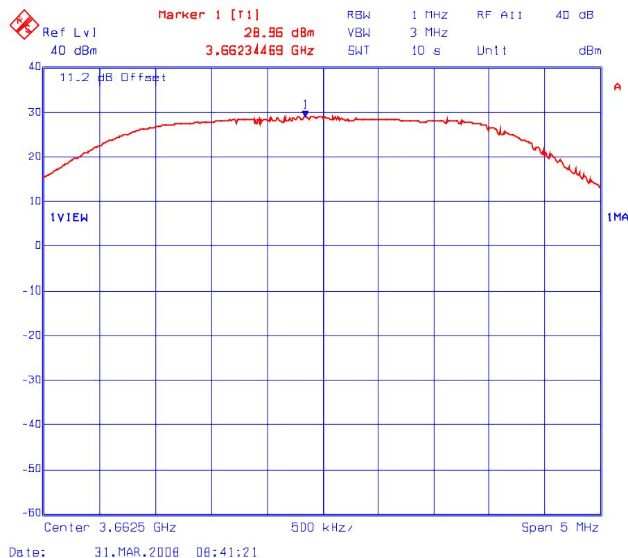
Plot # 2(b): Peak Conducted Power Density Measurement (Maximum Power Setting: 23 dBm)
