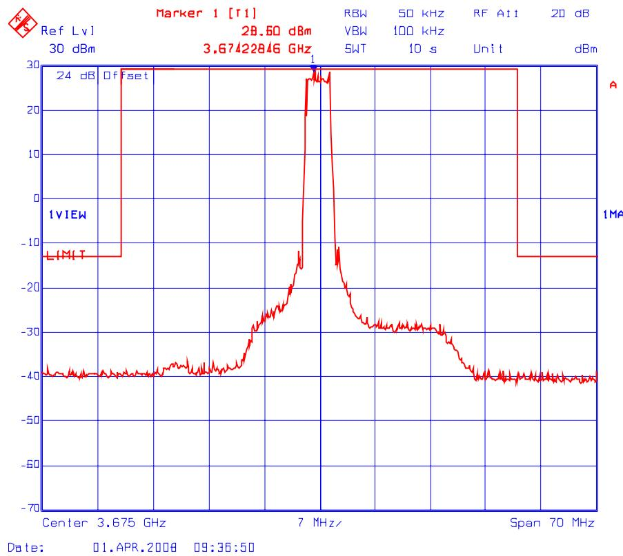
**Plot # 14(a): Conducted Band-edge Emissions (Lower Edge)
