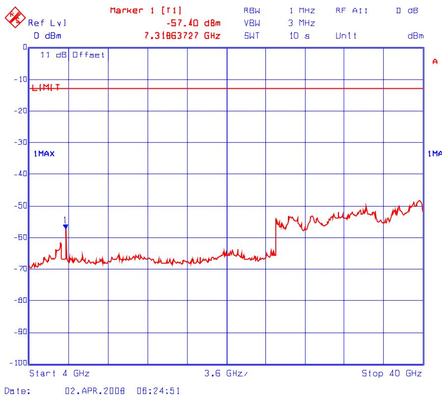
**Plot # 20(a): Transmitter Conducted Spurious Emissions**
