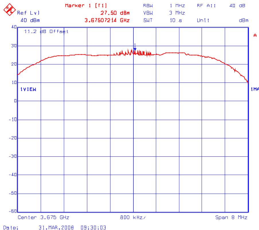
Plot # 6(d): Peak Conducted Power Density Measurement (Maximum Power Setting: 23 dBm)
