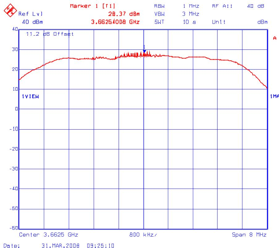
Plot # 6(a): Peak Conducted Power Density Measurement (Maximum Power Setting: 23 dBm)
