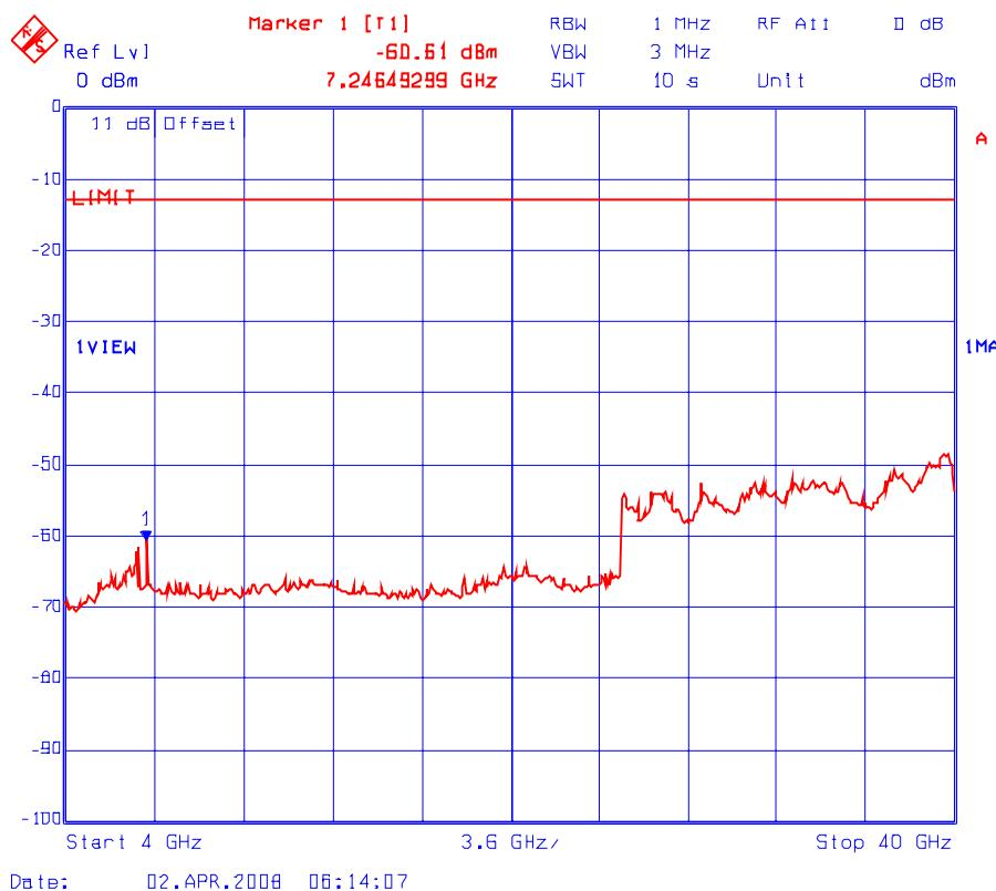
**Plot # 16(a): Transmitter Conducted Spurious Emissions**
