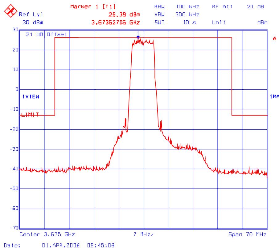
**Plot # 15(a): Transmitter Conducted Spurious Emissions**
