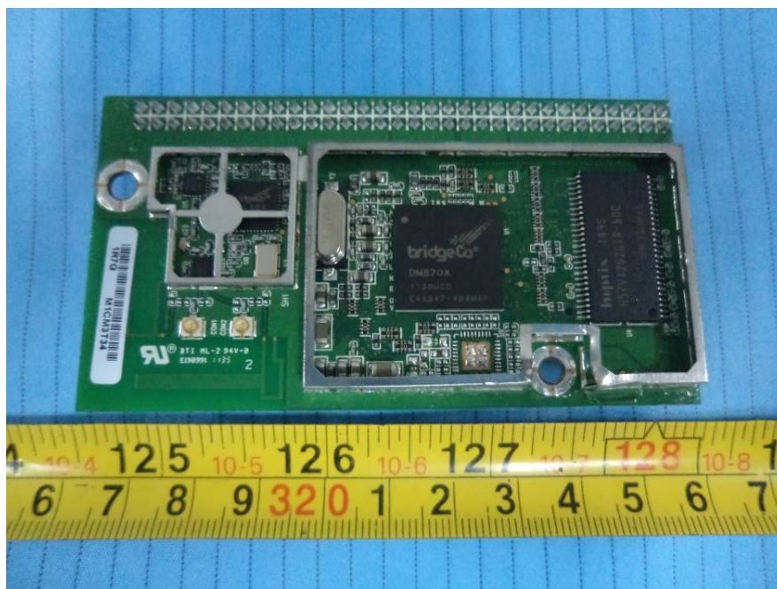
EUT – RF Module Shielding off Top View
