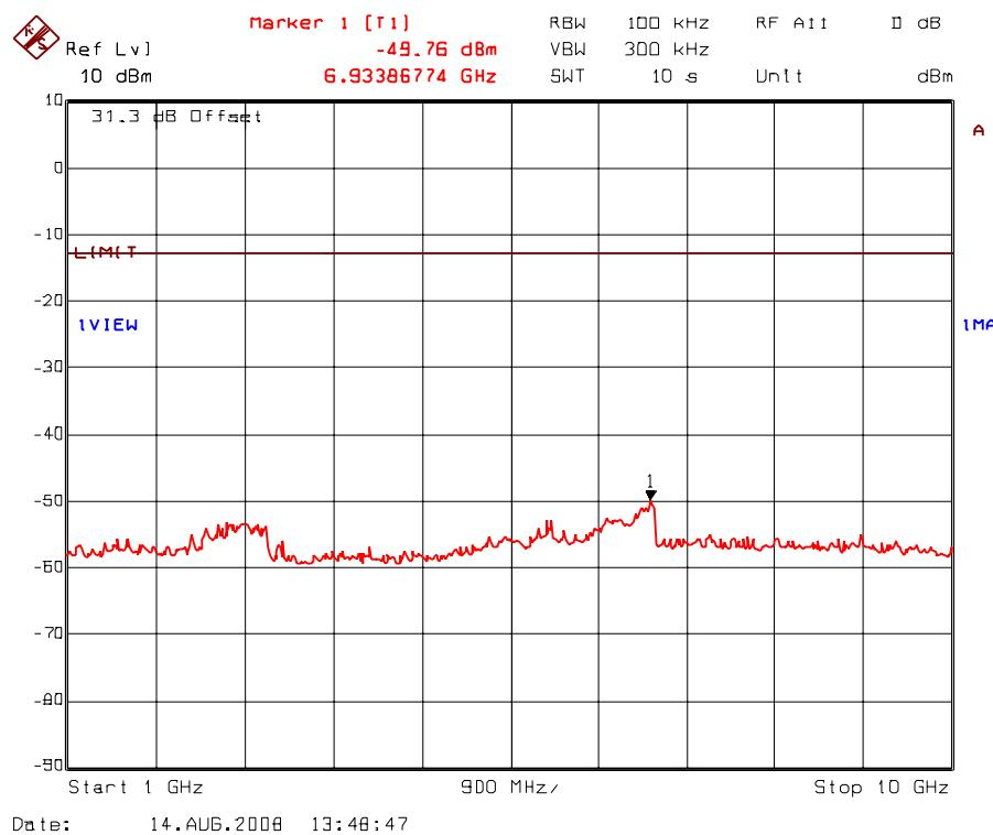
Plot 5.8.5.27. Transmitter antenna conducted RF spurious emissions at antenna port
