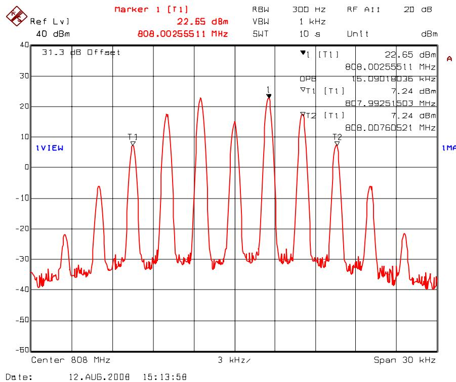
Plot 5.7.4.1.15. 99% Occupied Bandwidth – RF Output Signal
