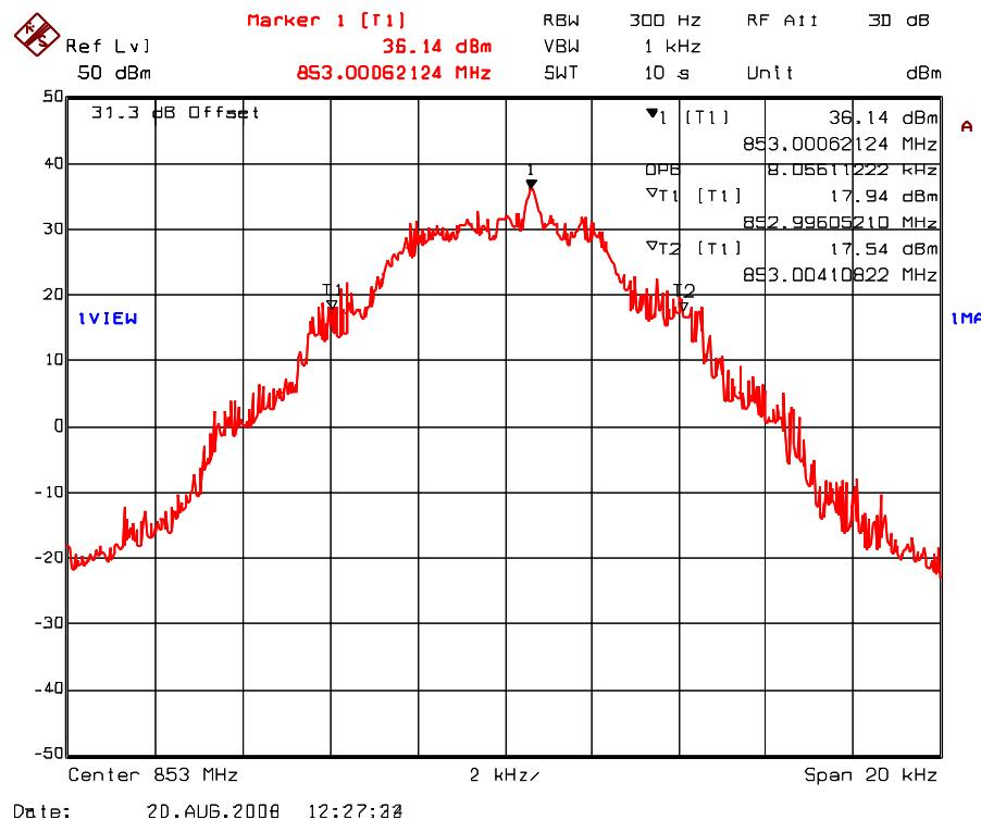
Plot 5.7.4.1.58. 99% Occupied Bandwidth – RF Output Signal
