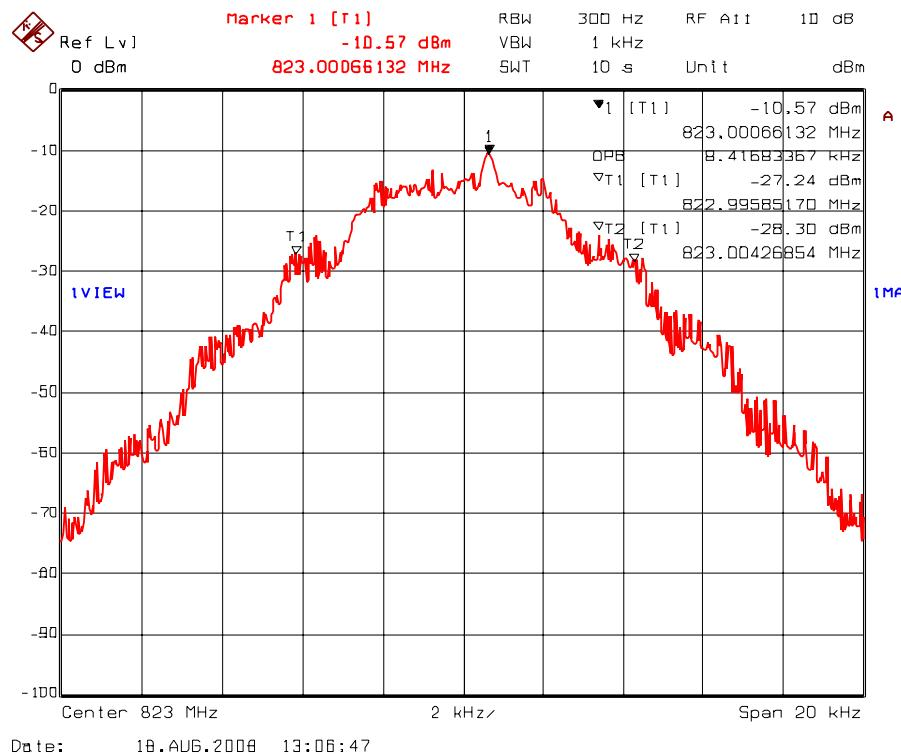
Plot 5.7.4.1.21. 99% Occupied Bandwidth – RF Output Signal
