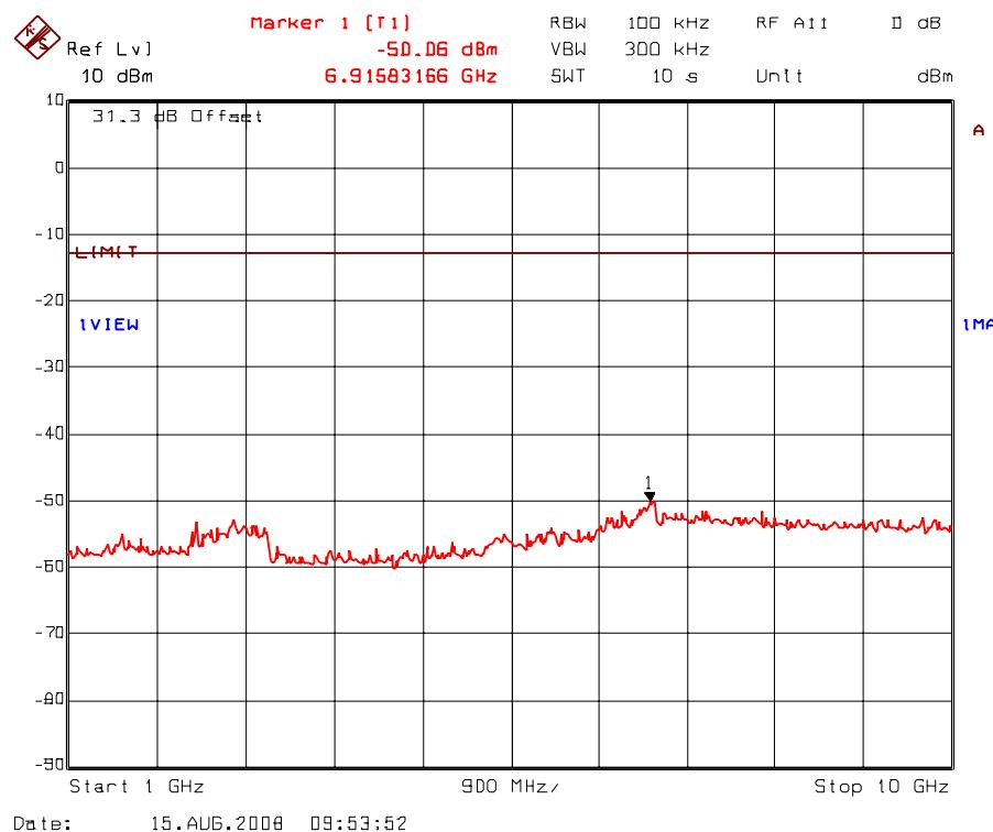
Plot 5.8.5.39. Transmitter antenna conducted RF spurious emissions at antenna port
