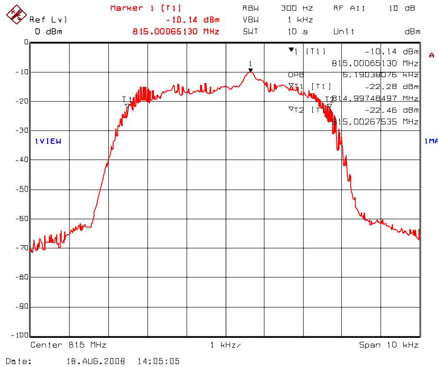
Plot 5.7.4.1.28. 99% Occupied Bandwidth – RF Input Signal
