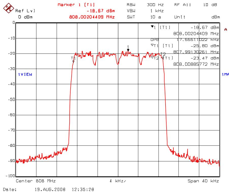
Plot 5.7.4.1.35. 99% Occupied Bandwidth – RF Input Signal
