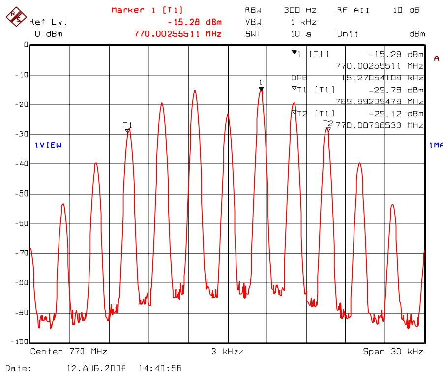
Plot 5.7.4.1.48. 99% Occupied Bandwidth – RF Input Signal
