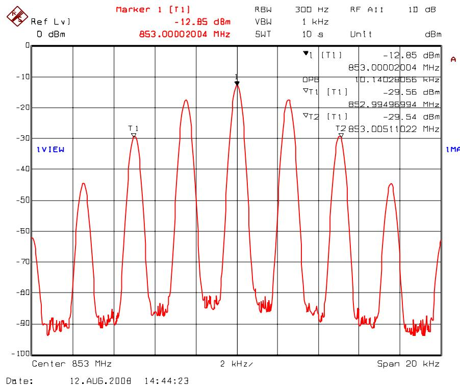
Plot 5.7.4.1.43. 99% Occupied Bandwidth – RF Input Signal
