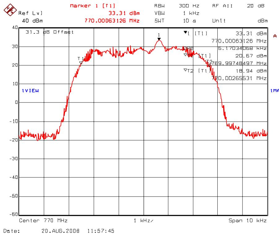
Plot 5.7.4.1.63. 99% Occupied Bandwidth – RF Output Signal
