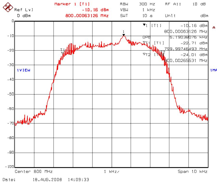
Plot 5.7.4.1.26. 99% Occupied Bandwidth – RF Input Signal
