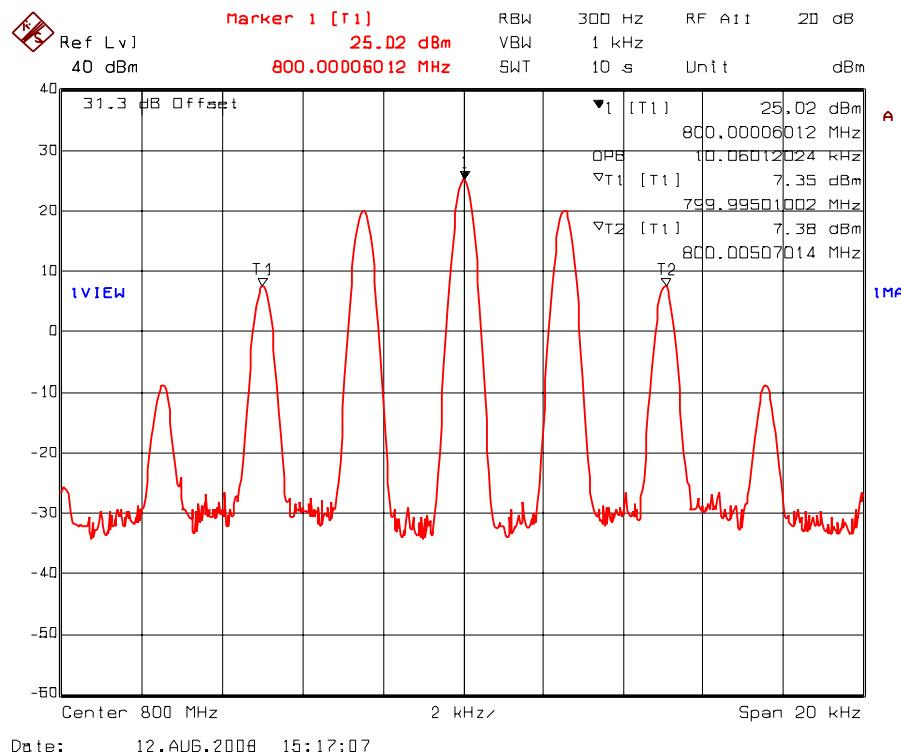
Plot 5.7.4.1.6. 99% Occupied Bandwidth – RF Output Signal
