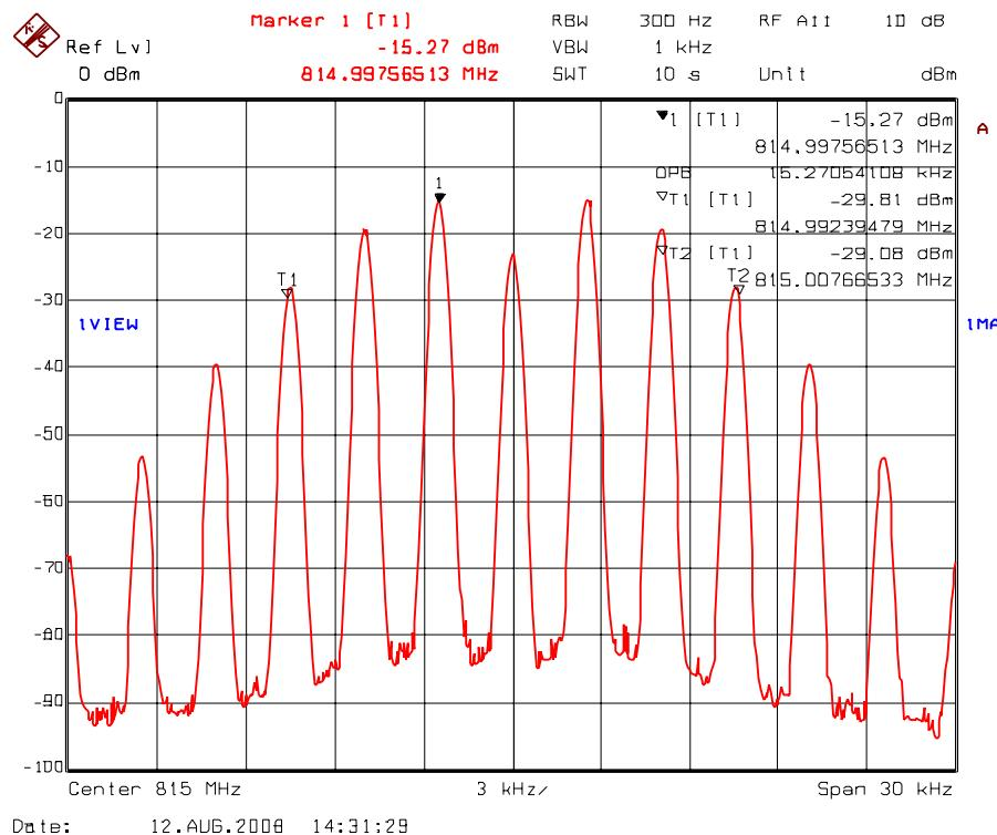
Plot 5.7.4.1.12. 99% Occupied Bandwidth – RF Input Signal
