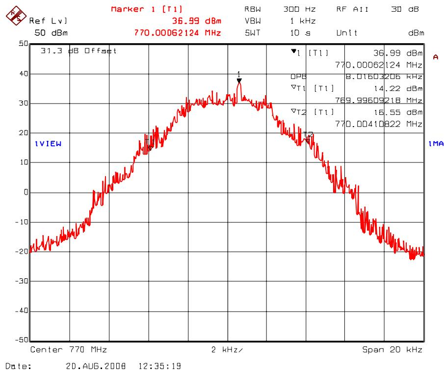
Plot 5.7.4.1.57. 99% Occupied Bandwidth – RF Output Signal
