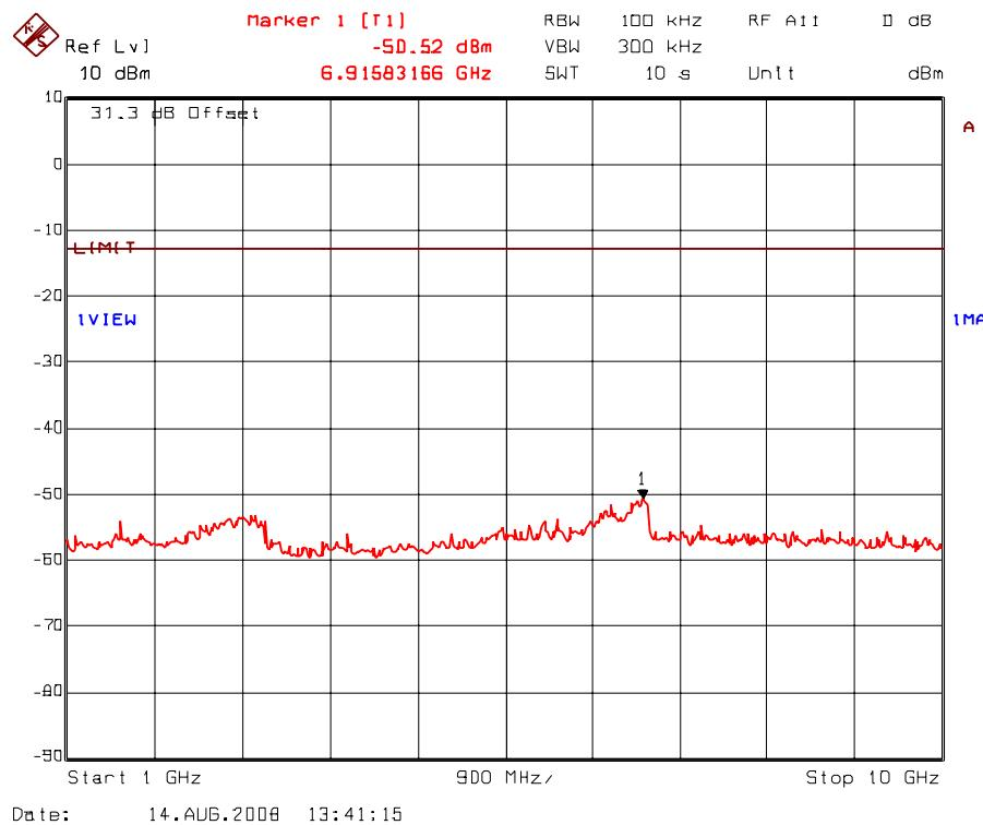
Plot 5.8.5.25. Transmitter antenna conducted RF spurious emissions at antenna port
