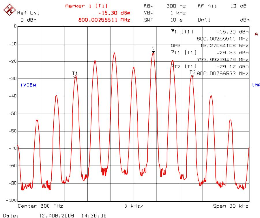
Plot 5.7.4.1.10. 99% Occupied Bandwidth – RF Input Signal
