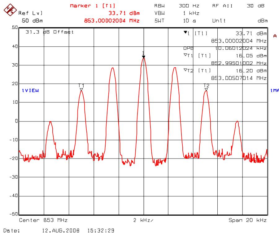
Plot 5.7.4.1.46. 99% Occupied Bandwidth – RF Output Signal
