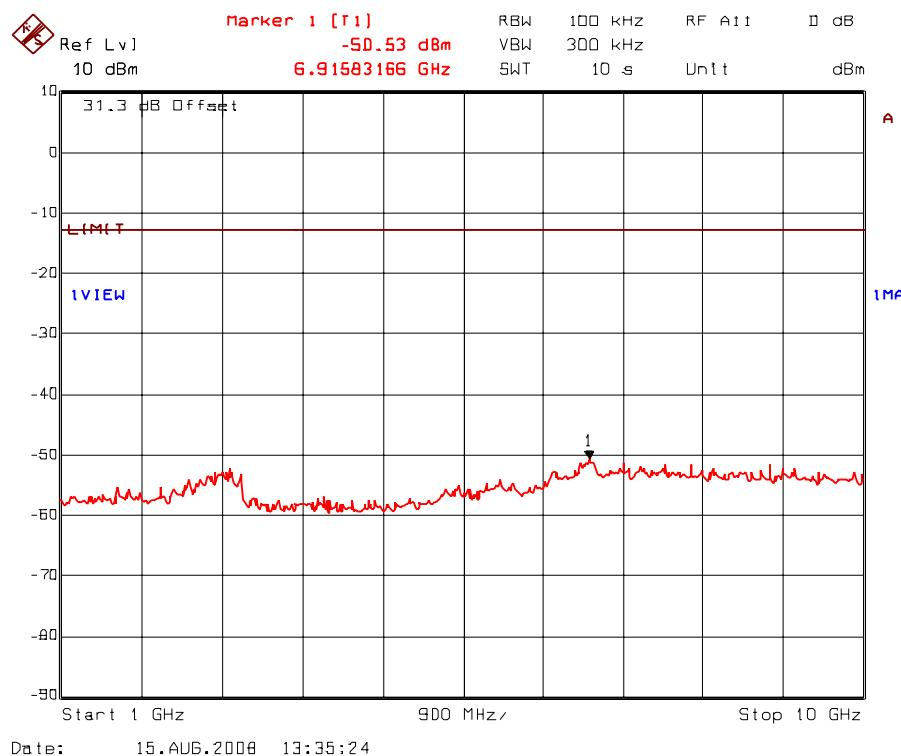
Plot 5.8.5.23. Transmitter antenna conducted RF spurious emissions at antenna port
