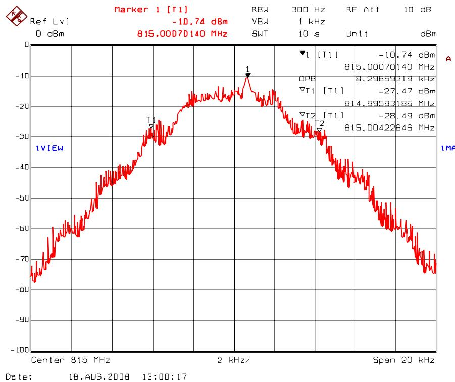
Plot 5.7.4.1.20. 99% Occupied Bandwidth – RF Input Signal
