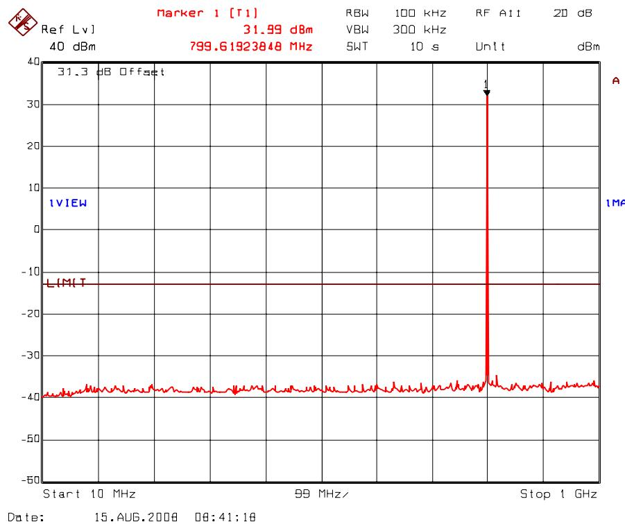
Plot 5.8.5.30. Transmitter antenna conducted RF spurious emissions at antenna port
