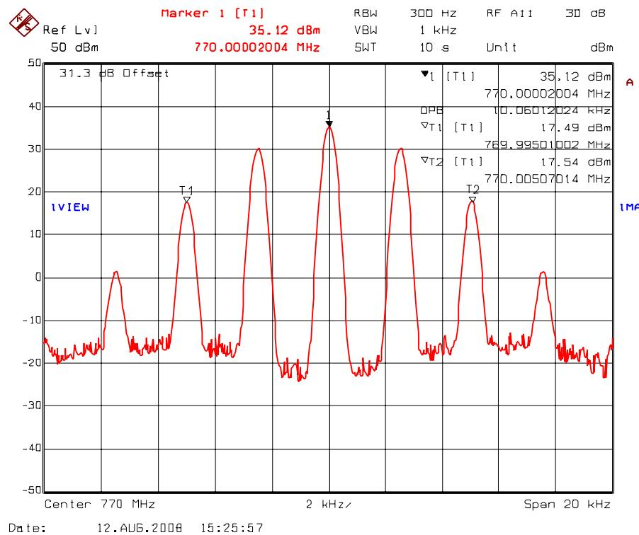
Plot 5.7.4.1.45. 99% Occupied Bandwidth – RF Output Signal
