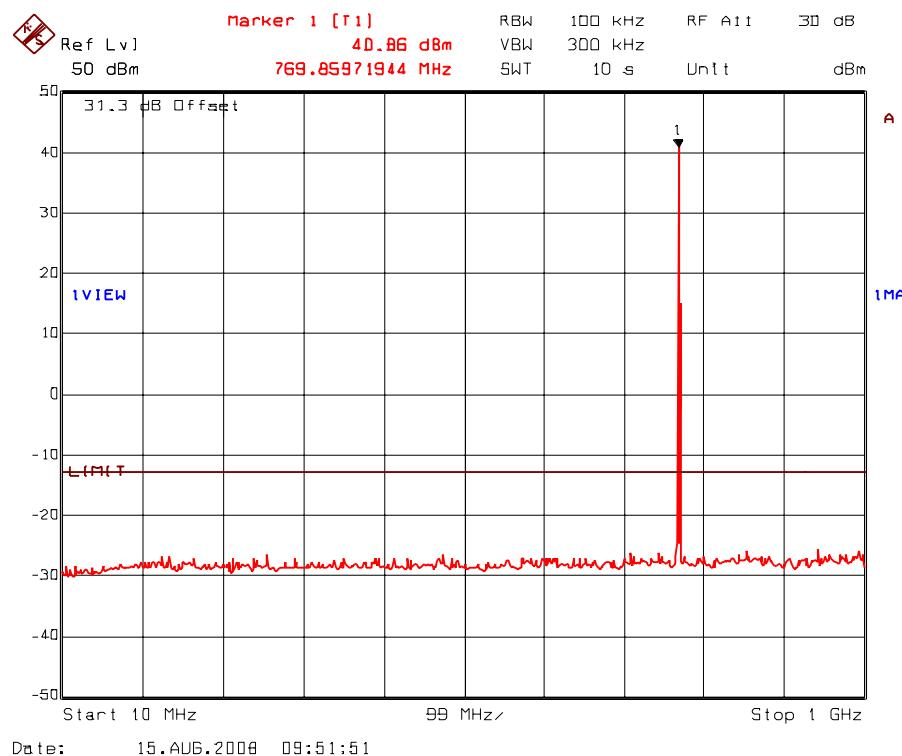
Plot 5.8.5.38. Transmitter antenna conducted RF spurious emissions at antenna port
