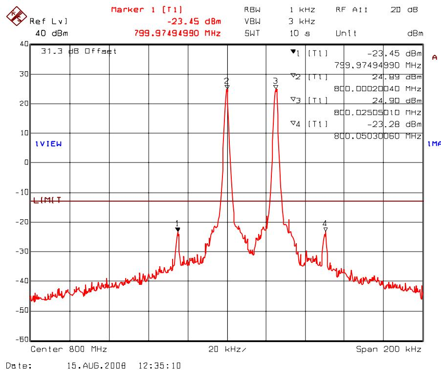
**Plot 5.5.4.2.2. Intermodulation with 2 RF signal inputs/outputs**
