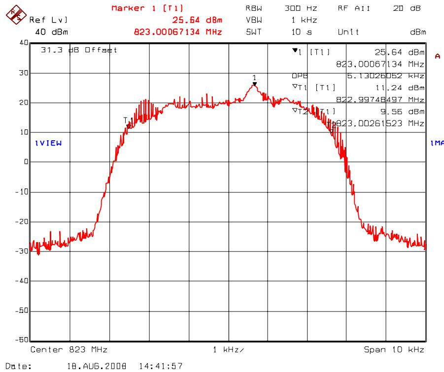
Plot 5.7.4.1.33. 99% Occupied Bandwidth – RF Input Signal
