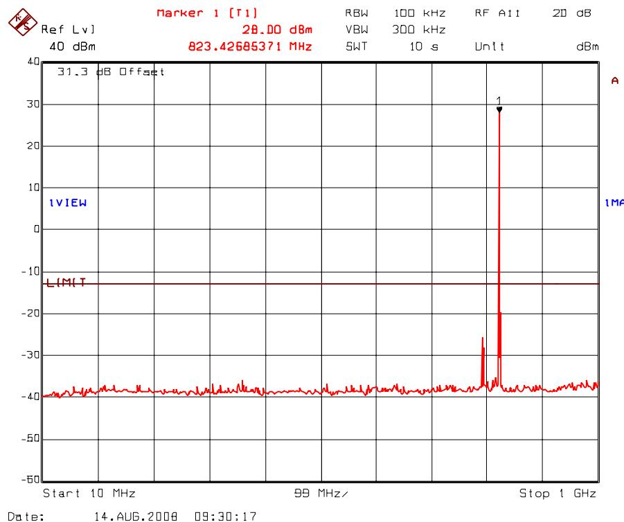
Plot 5.8.5.8. Transmitter antenna conducted RF spurious emissions at antenna port
