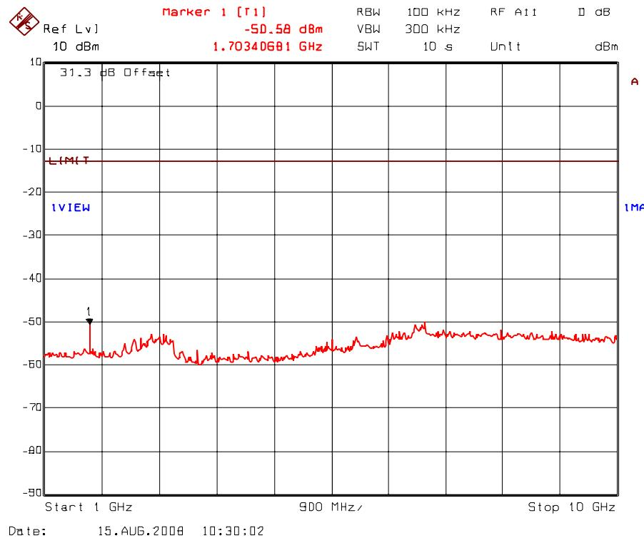
Plot 5.8.5.41. Transmitter antenna conducted RF spurious emissions at antenna port
