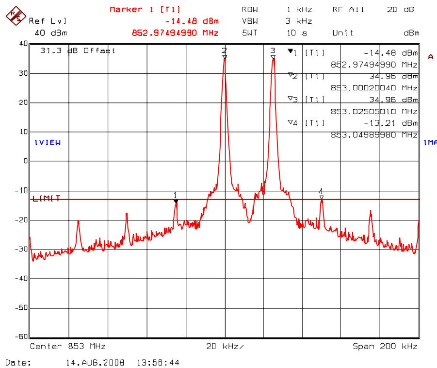
**Plot 5.5.4.2.11. Intermodulation with 2 RF signal inputs/outputs**
