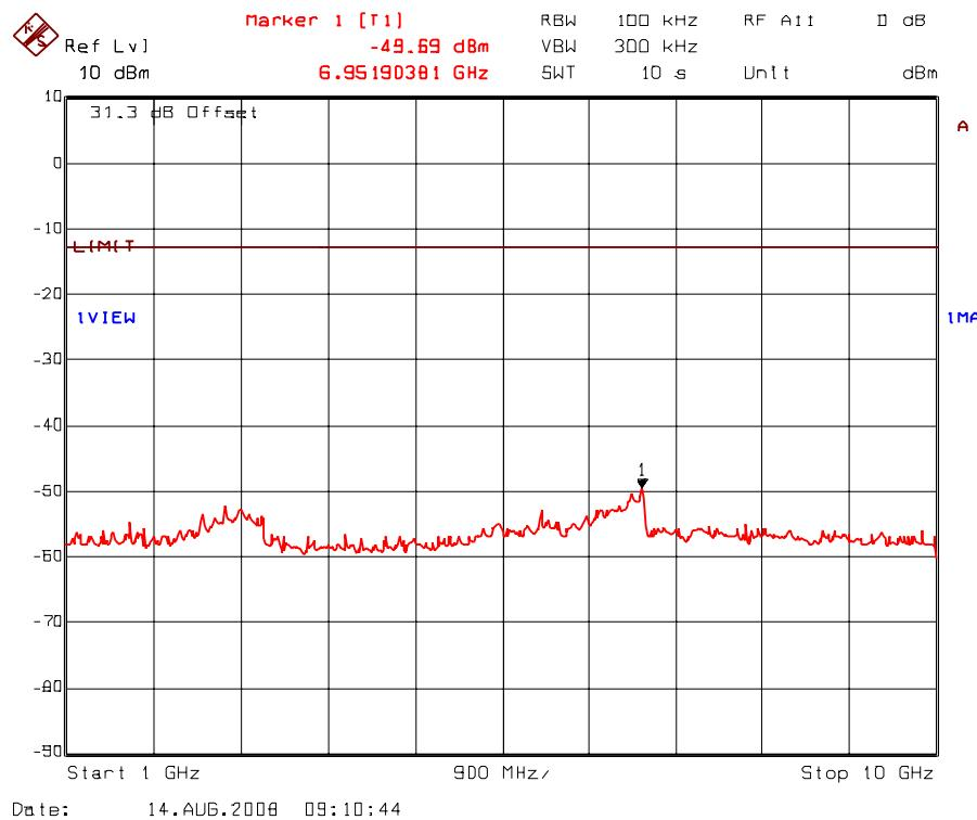
Plot 5.8.5.5. Transmitter antenna conducted RF spurious emissions at antenna port
