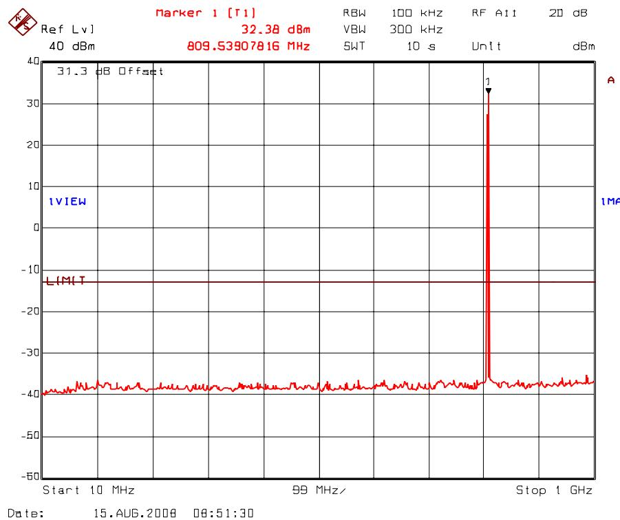
Plot 5.8.5.32. Transmitter antenna conducted RF spurious emissions at antenna port
