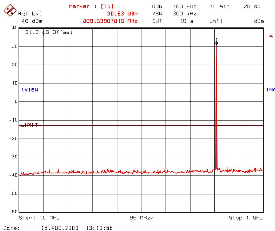
Plot 5.8.5.18. Transmitter antenna conducted RF spurious emissions at antenna port
