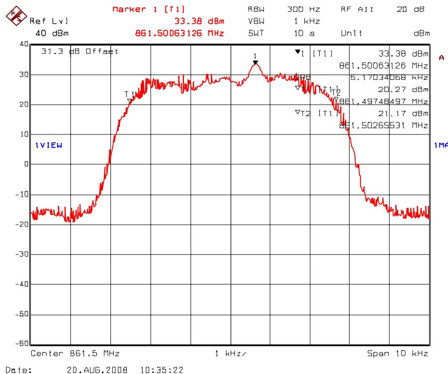
Plot 5.7.4.1.65. 99% Occupied Bandwidth – RF Input Signal
