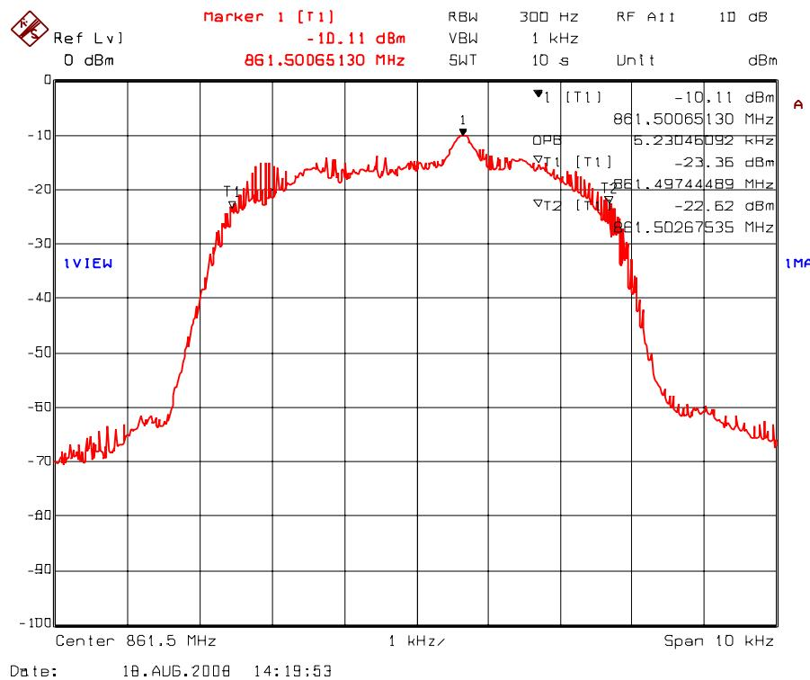
Plot 5.7.4.1.62. 99% Occupied Bandwidth – RF Output Signal
