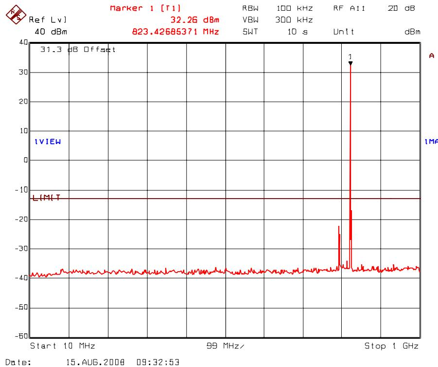
Plot 5.8.5.36. Transmitter antenna conducted RF spurious emissions at antenna port
