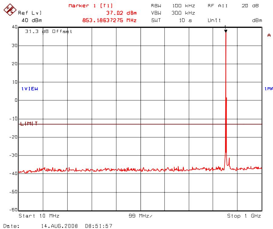
Plot 5.8.5.12. Transmitter antenna conducted RF spurious emissions at antenna port
