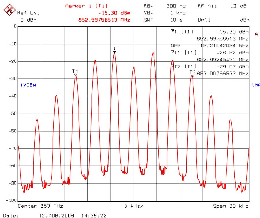
Plot 5.7.4.1.49. 99% Occupied Bandwidth – RF Input Signal
