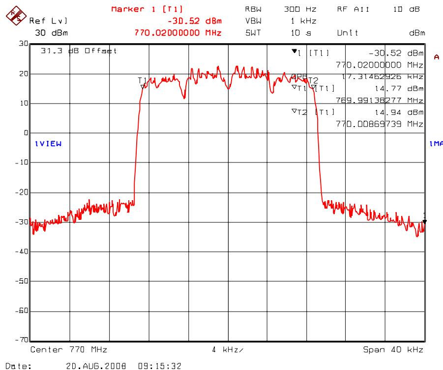
Plot 5.7.4.1.69. 99% Occupied Bandwidth – RF Output Signal
