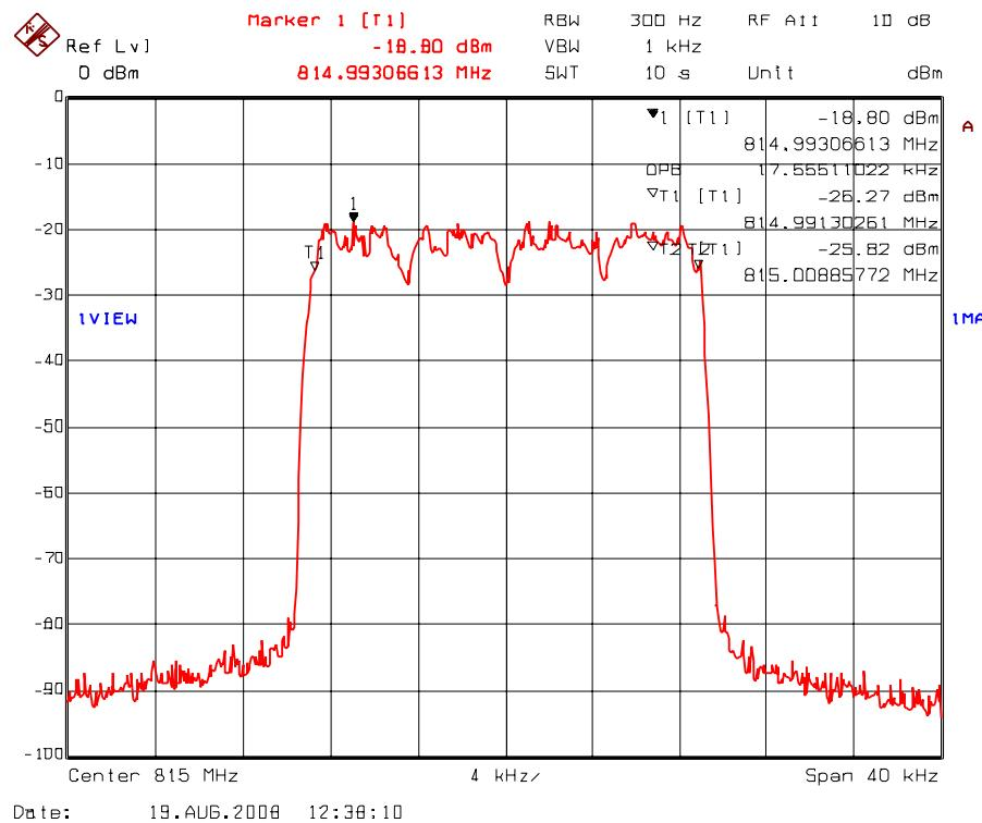
Plot 5.7.4.1.36. 99% Occupied Bandwidth – RF Input Signal
