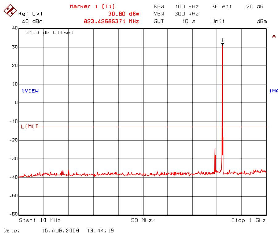
Plot 5.8.5.22. Transmitter antenna conducted RF spurious emissions at antenna port
