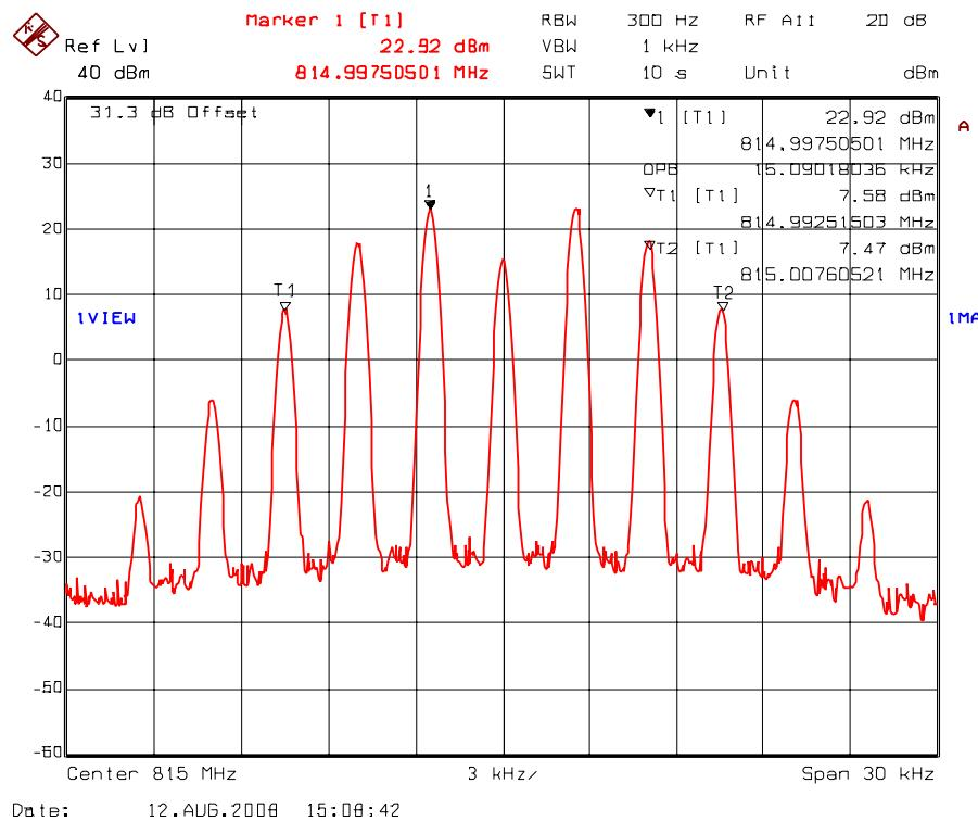
Plot 5.7.4.1.16. 99% Occupied Bandwidth – RF Output Signal
