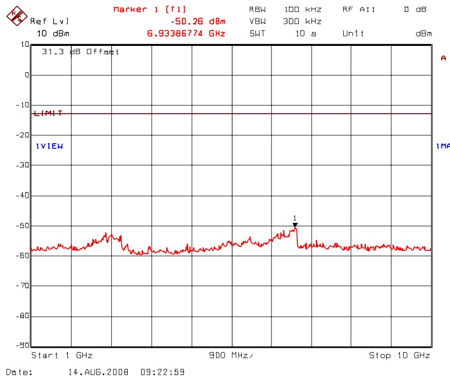
Plot 5.8.5.7. Transmitter antenna conducted RF spurious emissions at antenna port
