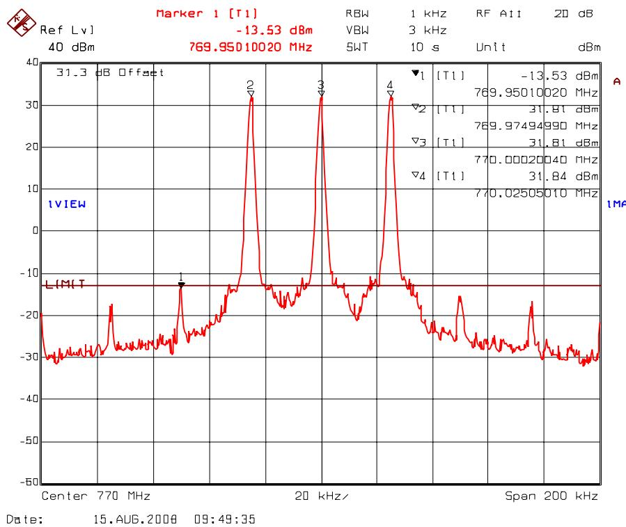
**Plot 5.5.4.2.13. Intermodulation with 3 RF signal inputs/outputs**
