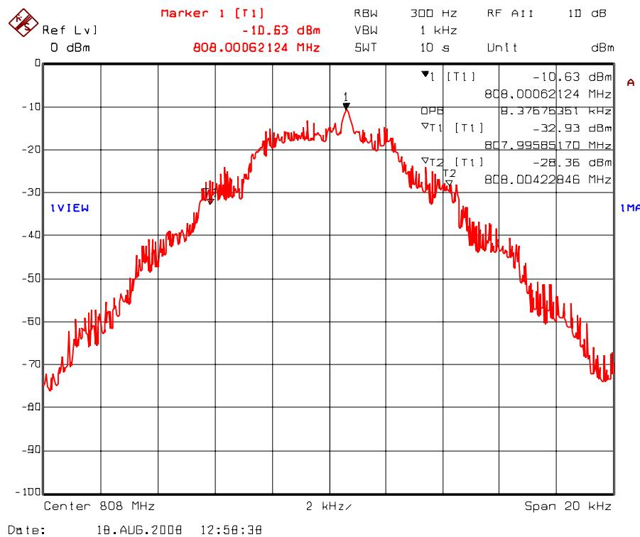
Plot 5.7.4.1.19. 99% Occupied Bandwidth – RF Input Signal
