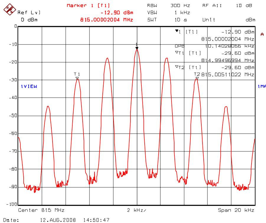
Plot 5.7.4.1.4. 99% Occupied Bandwidth – RF Input Signal
