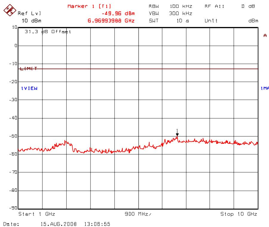
Plot 5.8.5.17. Transmitter antenna conducted RF spurious emissions at antenna port
