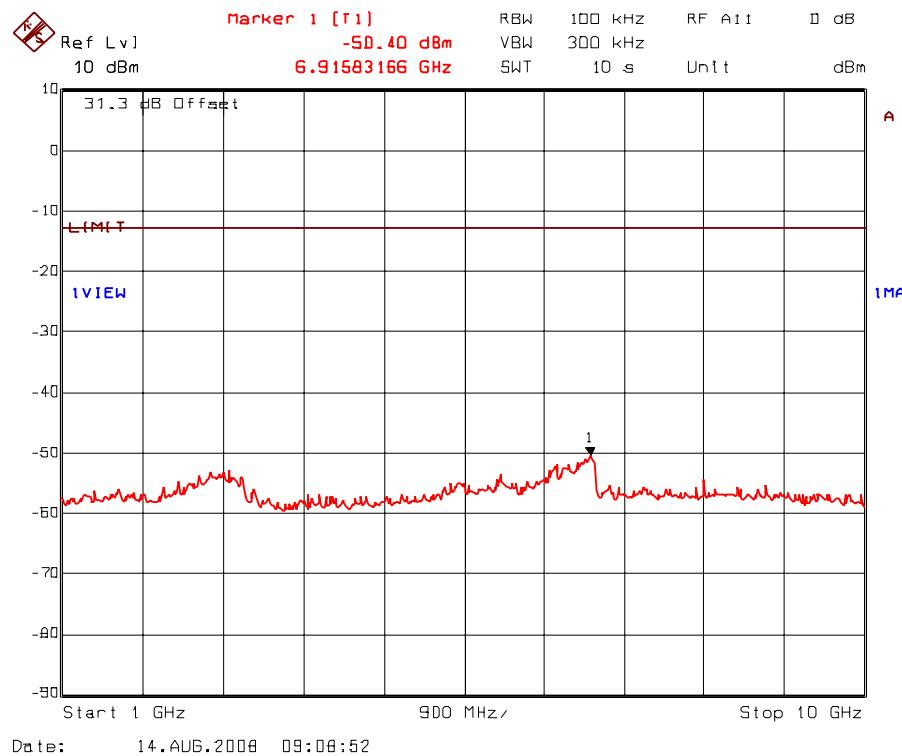
Plot 5.8.5.3. Transmitter antenna conducted RF spurious emissions at antenna port
