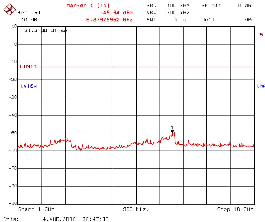
Plot 5.8.5.13. Transmitter antenna conducted RF spurious emissions at antenna port
