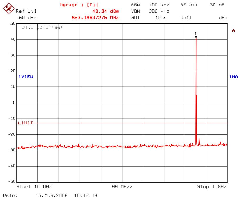
Plot 5.8.5.40. Transmitter antenna conducted RF spurious emissions at antenna port
