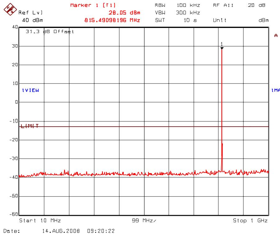
Plot 5.8.5.6. Transmitter antenna conducted RF spurious emissions at antenna port
