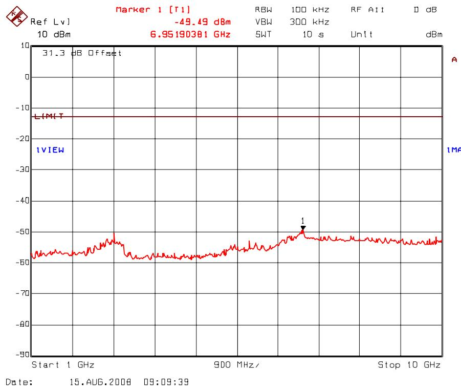
Plot 5.8.5.35. Transmitter antenna conducted RF spurious emissions at antenna port
