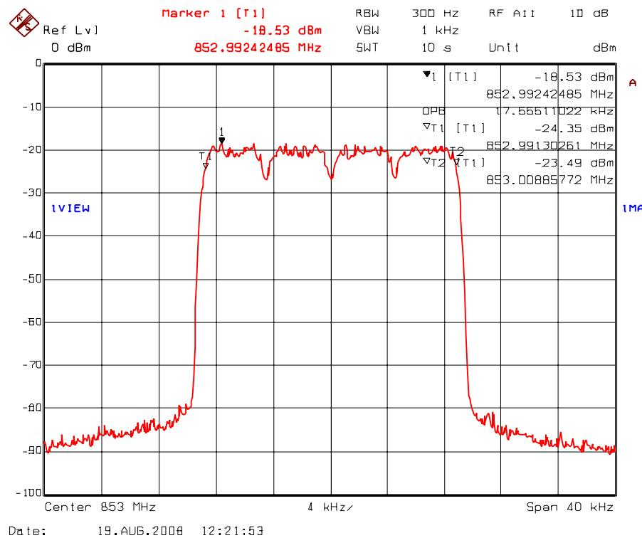
Plot 5.7.4.1.67. 99% Occupied Bandwidth – RF Input Signal
