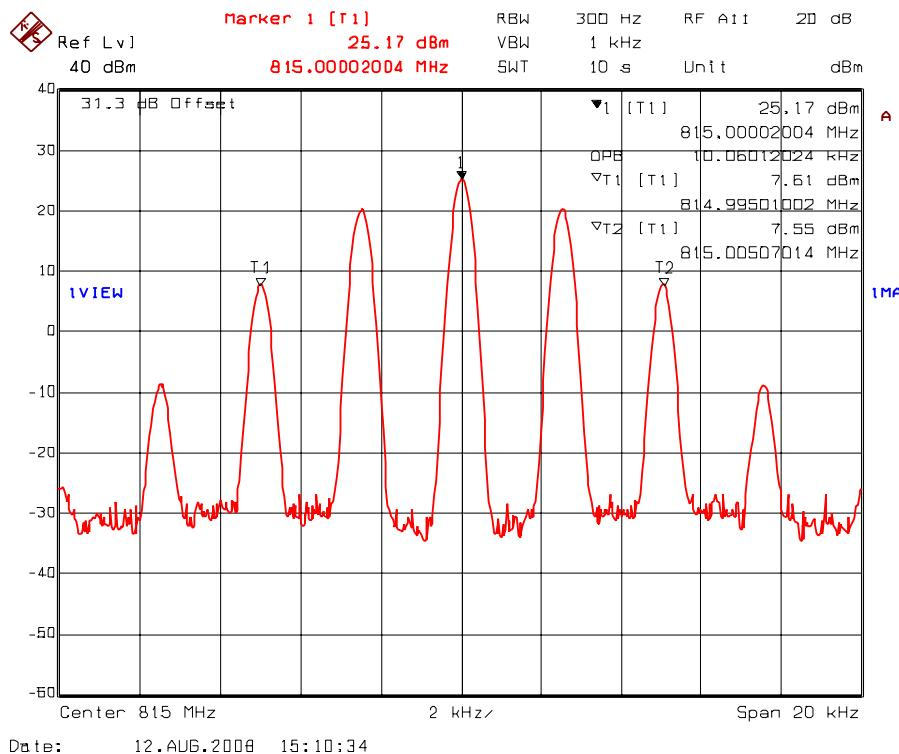
Plot 5.7.4.1.8. 99% Occupied Bandwidth – RF Output Signal
