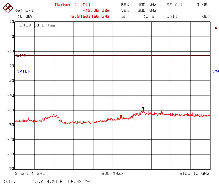
Plot 5.8.5.31. Transmitter antenna conducted RF spurious emissions at antenna port
