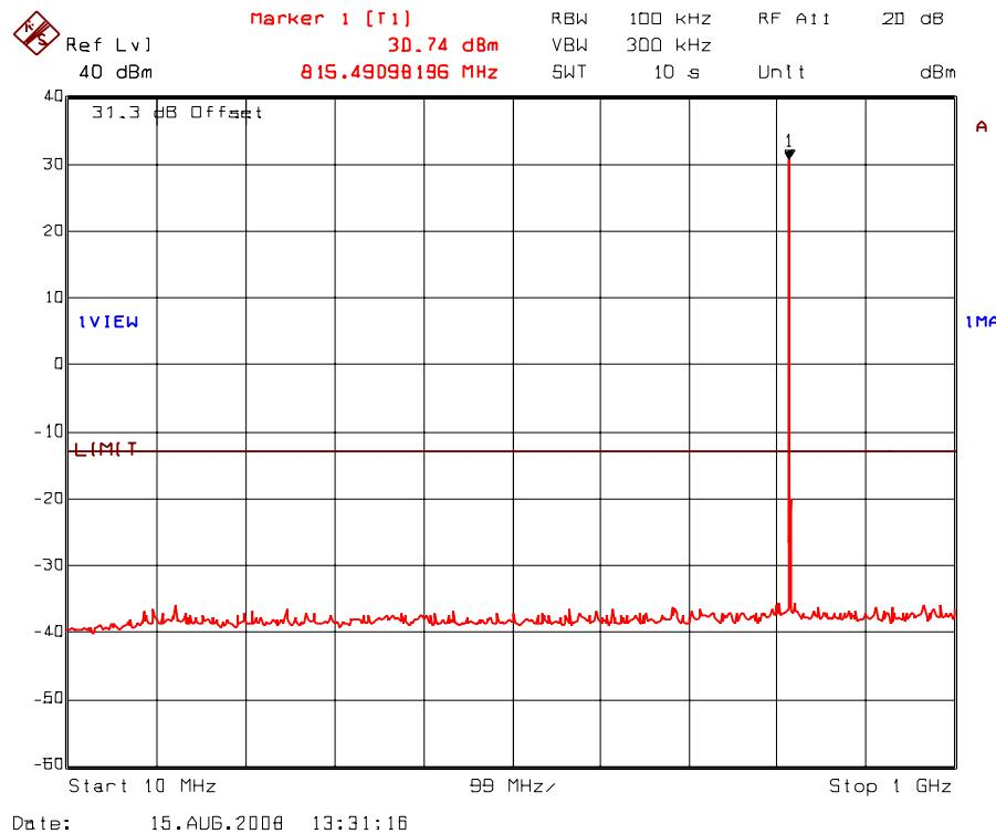
Plot 5.8.5.20. Transmitter antenna conducted RF spurious emissions at antenna port
