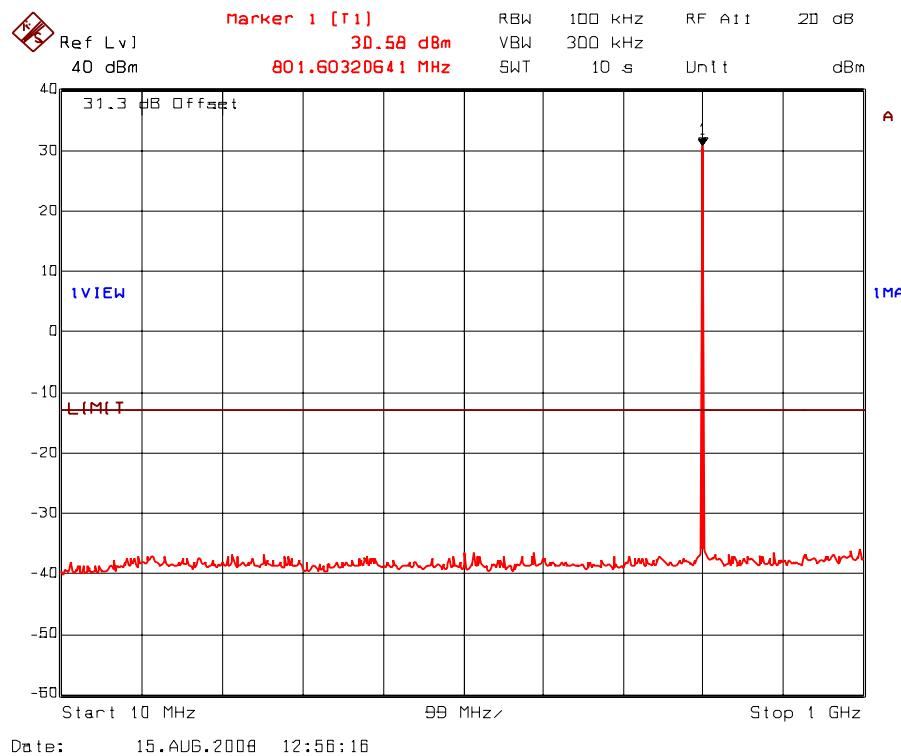
Plot 5.8.5.16. Transmitter antenna conducted RF spurious emissions at antenna port
