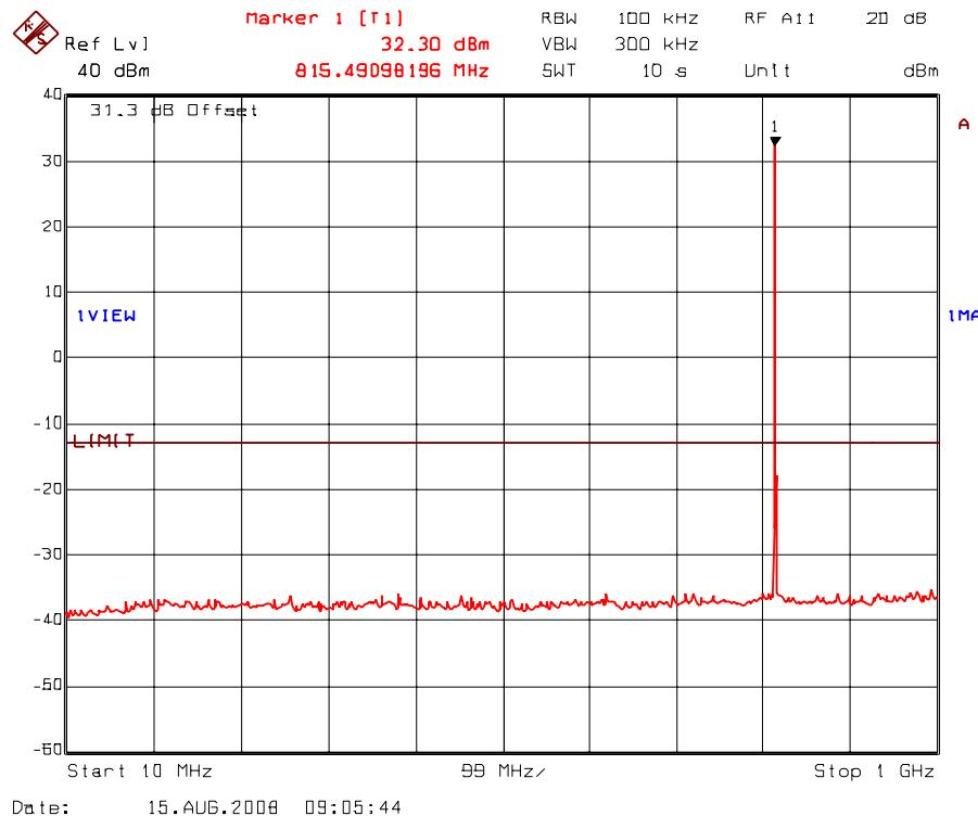
Plot 5.8.5.34. Transmitter antenna conducted RF spurious emissions at antenna port
