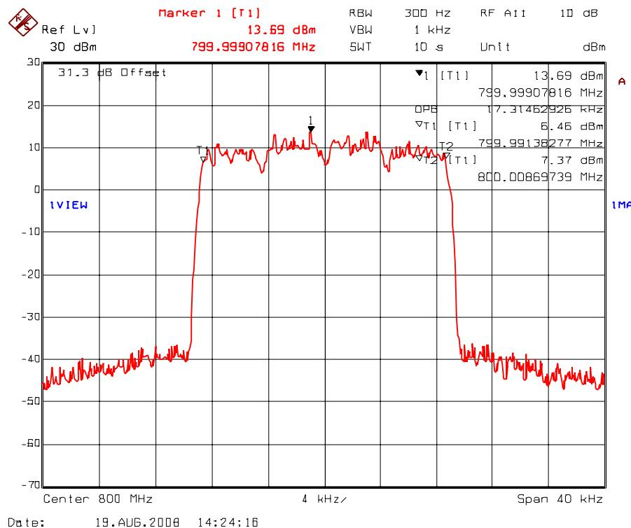
Plot 5.7.4.1.38. 99% Occupied Bandwidth – RF Output Signal
