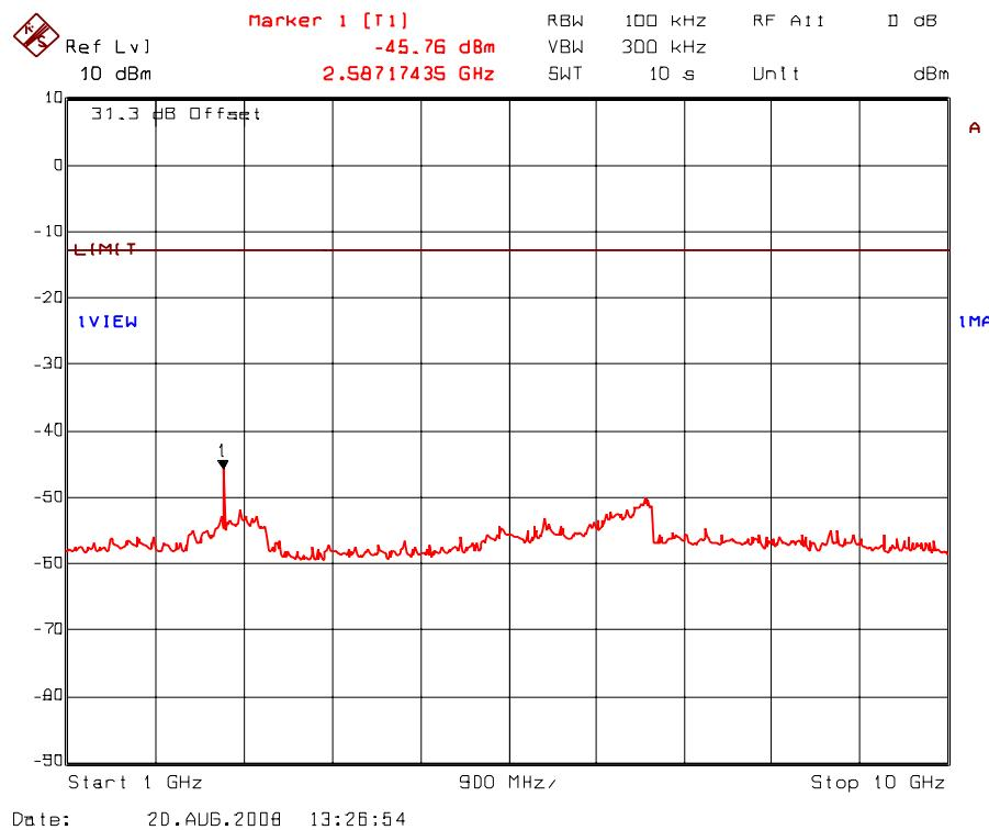
Plot 5.8.5.15. Transmitter antenna conducted RF spurious emissions at antenna port
