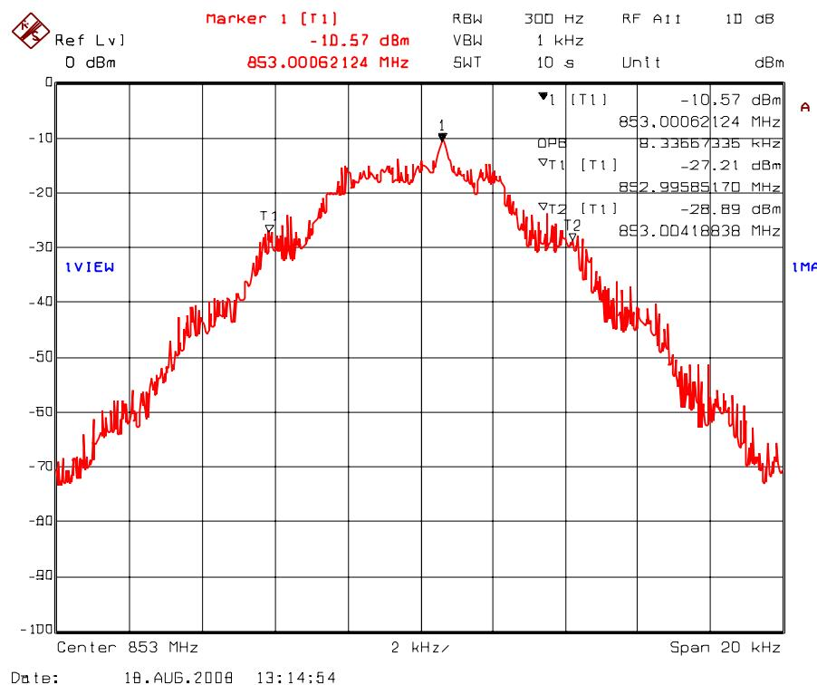
Plot 5.7.4.1.55. 99% Occupied Bandwidth – RF Input Signal
