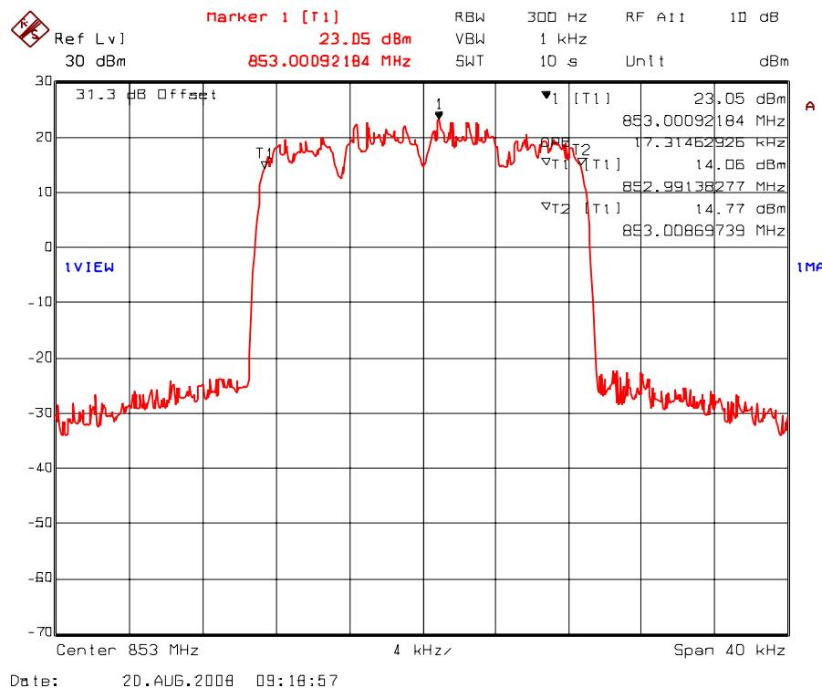
Plot 5.7.4.1.70. 99% Occupied Bandwidth – RF Output Signal
