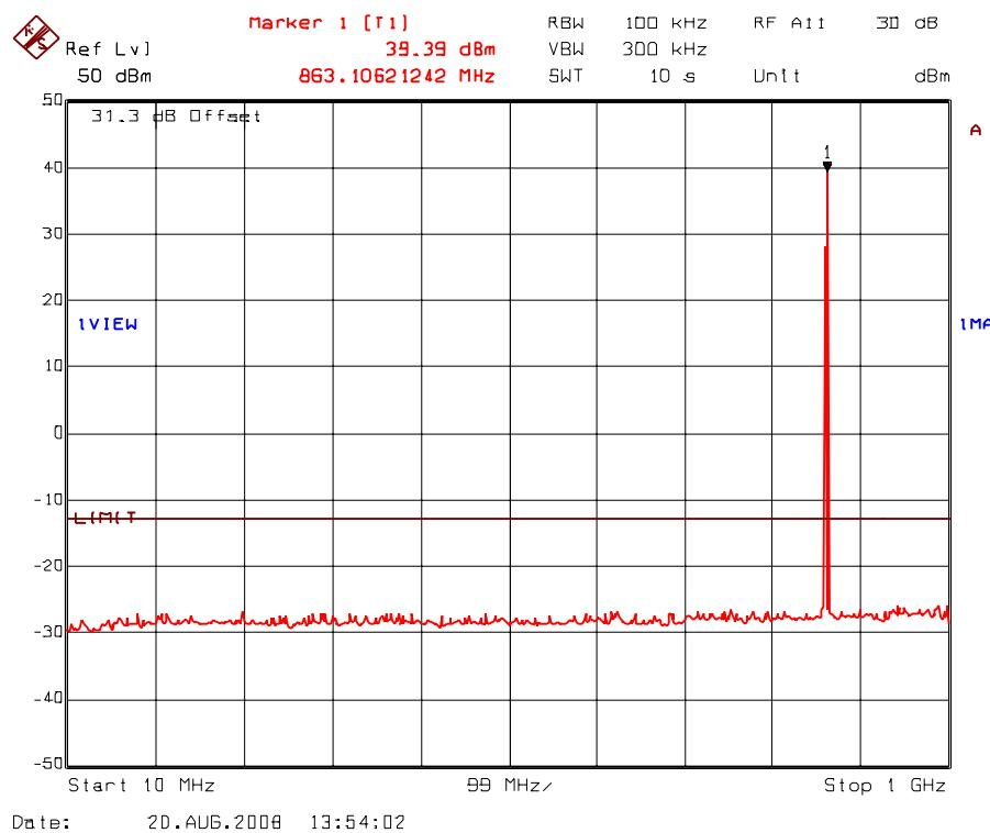
Plot 5.8.5.28. Transmitter antenna conducted RF spurious emissions at antenna port
