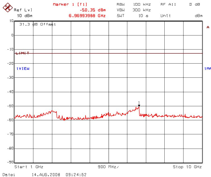
Plot 5.8.5.9. Transmitter antenna conducted RF spurious emissions at antenna port
