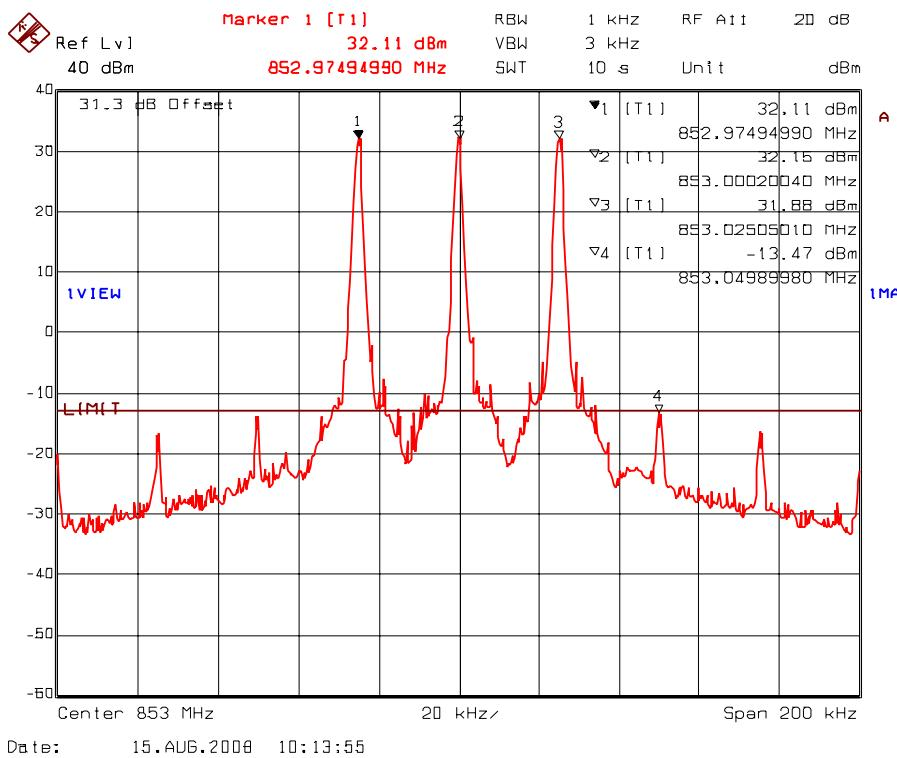
**Plot 5.5.4.2.14. Intermodulation with 3 RF signal inputs/outputs**
