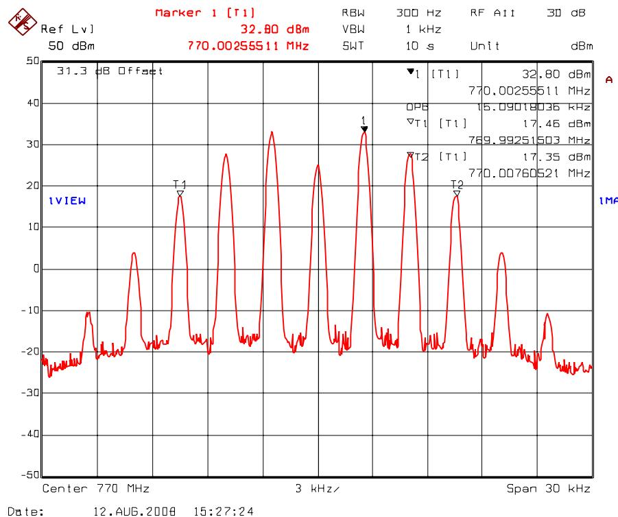
Plot 5.7.4.1.51. 99% Occupied Bandwidth – RF Output Signal
