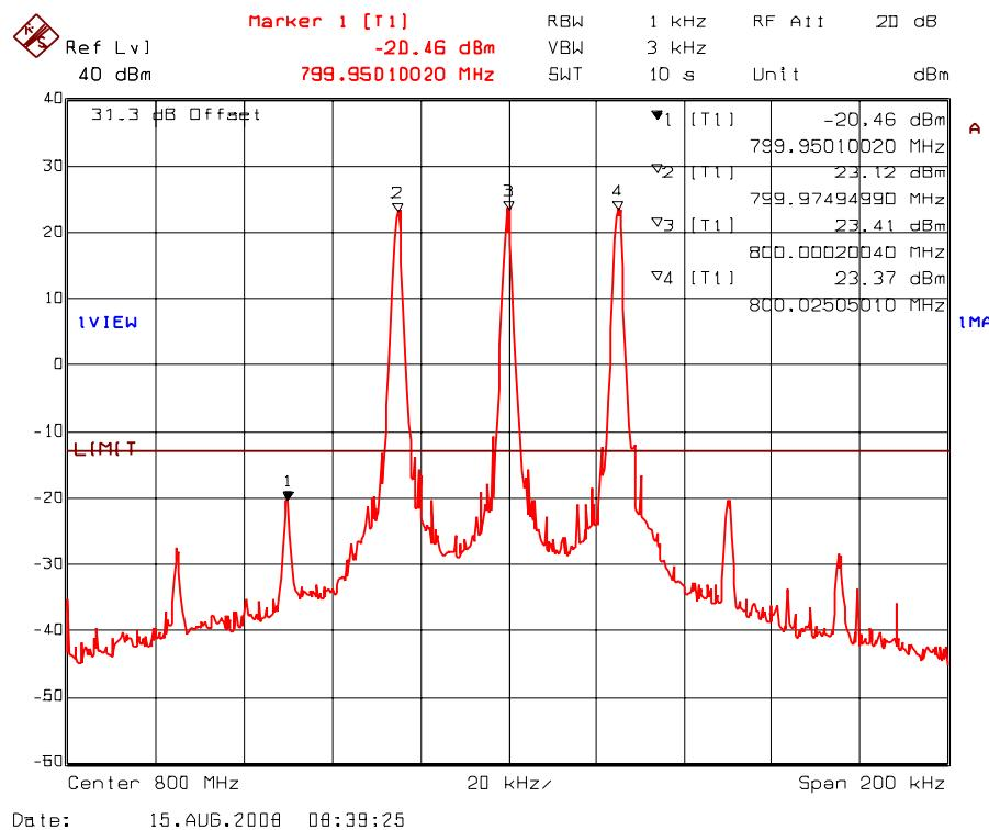
**Plot 5.5.4.2.6. Intermodulation with 3 RF signal inputs/outputs**
