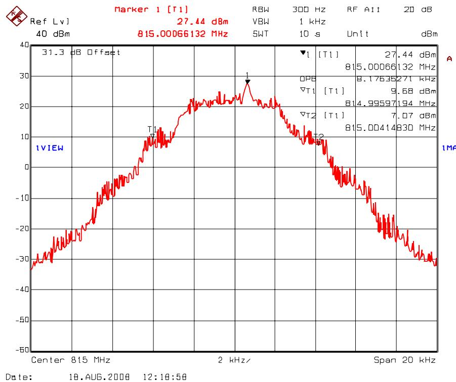
Plot 5.7.4.1.24. 99% Occupied Bandwidth – RF Output Signal
