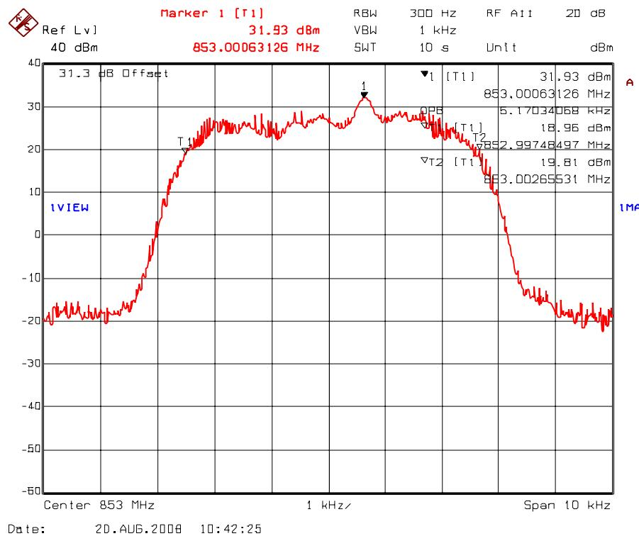
Plot 5.7.4.1.64. 99% Occupied Bandwidth – RF Output Signal
