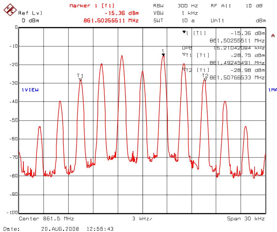
Plot 5.7.4.1.50. 99% Occupied Bandwidth – RF Output Signal
