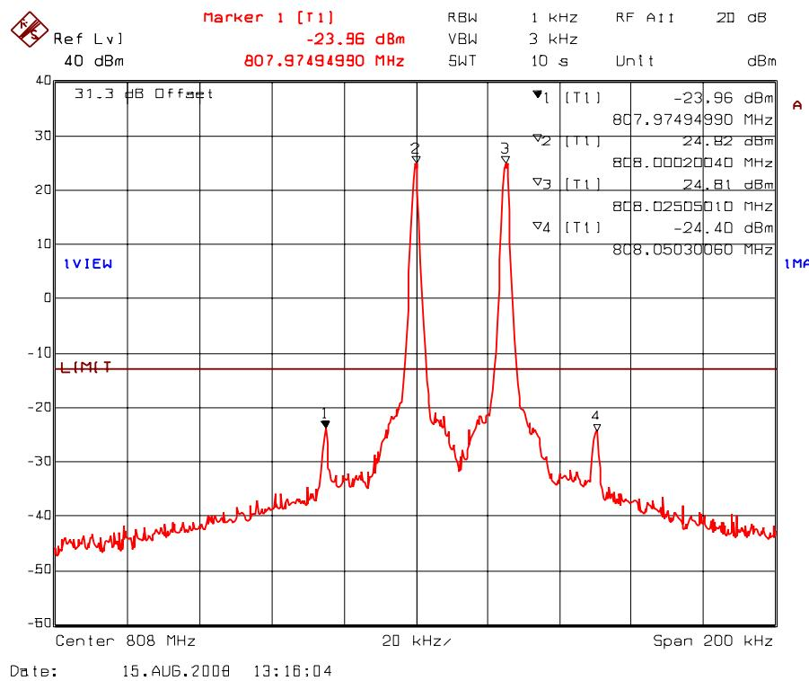
**Plot 5.5.4.2.3. Intermodulation with 2 RF signal inputs/outputs**
