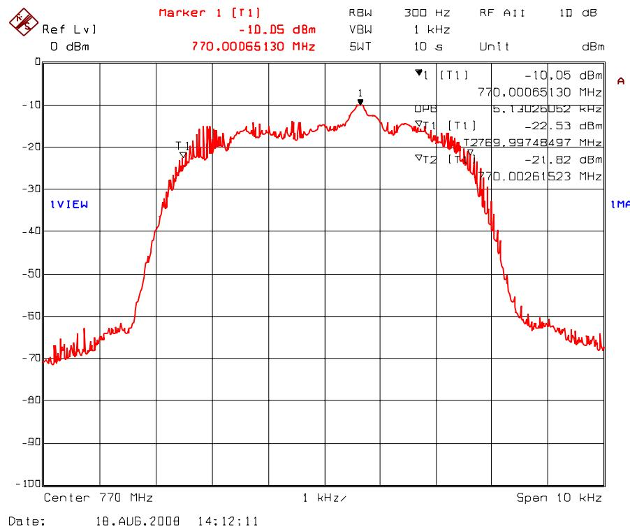
Plot 5.7.4.1.60. 99% Occupied Bandwidth – RF Input Signal
