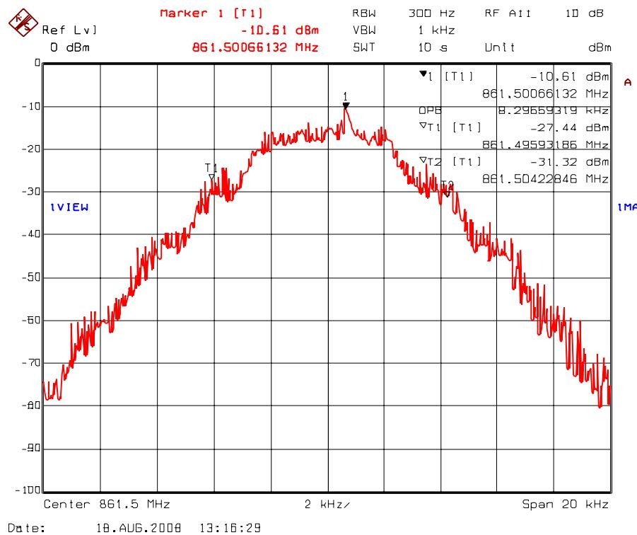
Plot 5.7.4.1.56. 99% Occupied Bandwidth – RF Output Signal
