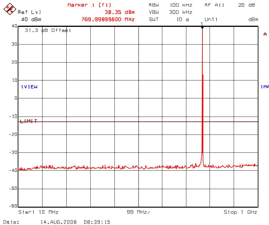
Plot 5.8.5.10. Transmitter antenna conducted RF spurious emissions at antenna port
