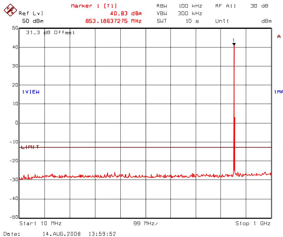
Plot 5.8.5.26. Transmitter antenna conducted RF spurious emissions at antenna port
