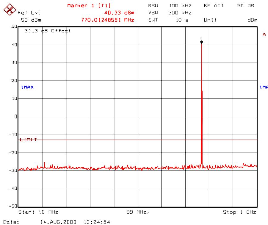
Plot 5.8.5.24. Transmitter antenna conducted RF spurious emissions at antenna port
