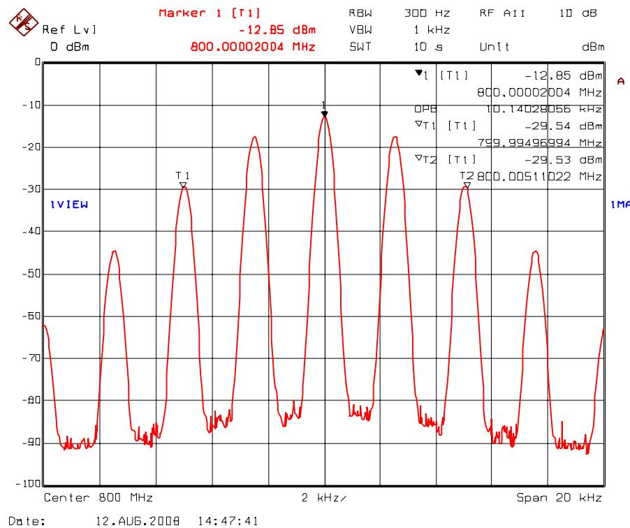
Plot 5.7.4.1.2. 99% Occupied Bandwidth – RF Input Signal
