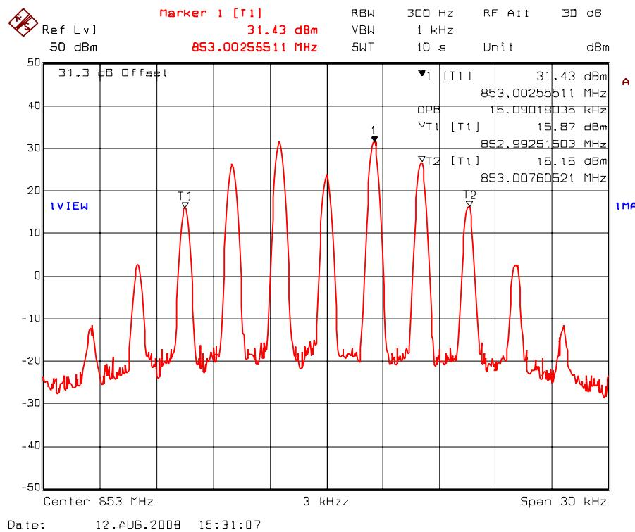
Plot 5.7.4.1.52. 99% Occupied Bandwidth – RF Output Signal
