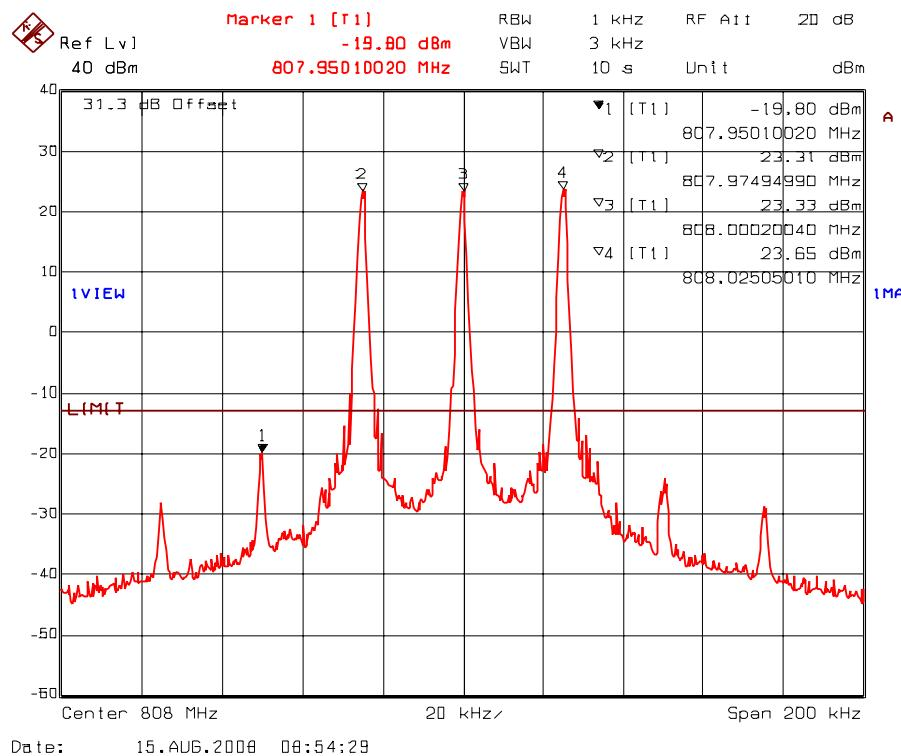
**Plot 5.5.4.2.7. Intermodulation with 3 RF signal inputs/outputs**
