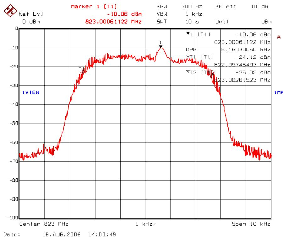
Plot 5.7.4.1.29. 99% Occupied Bandwidth – RF Output Signal
