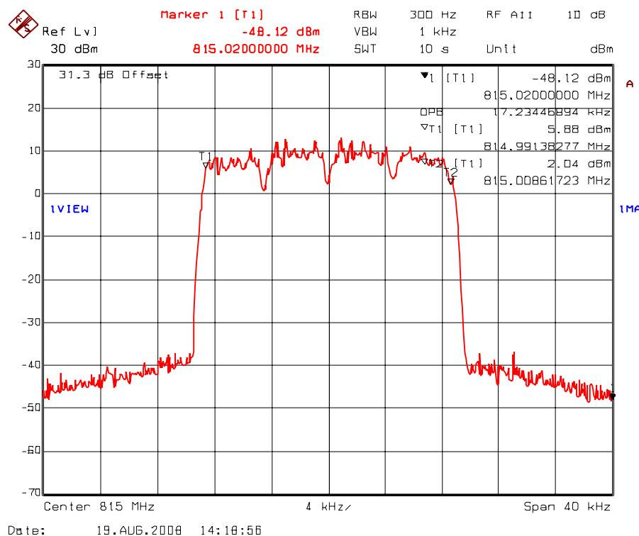
Plot 5.7.4.1.40. 99% Occupied Bandwidth – RF Output Signal
