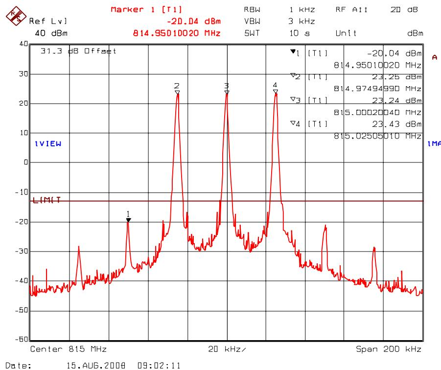
**Plot 5.5.4.2.8. Intermodulation with 3 RF signal inputs/outputs**
