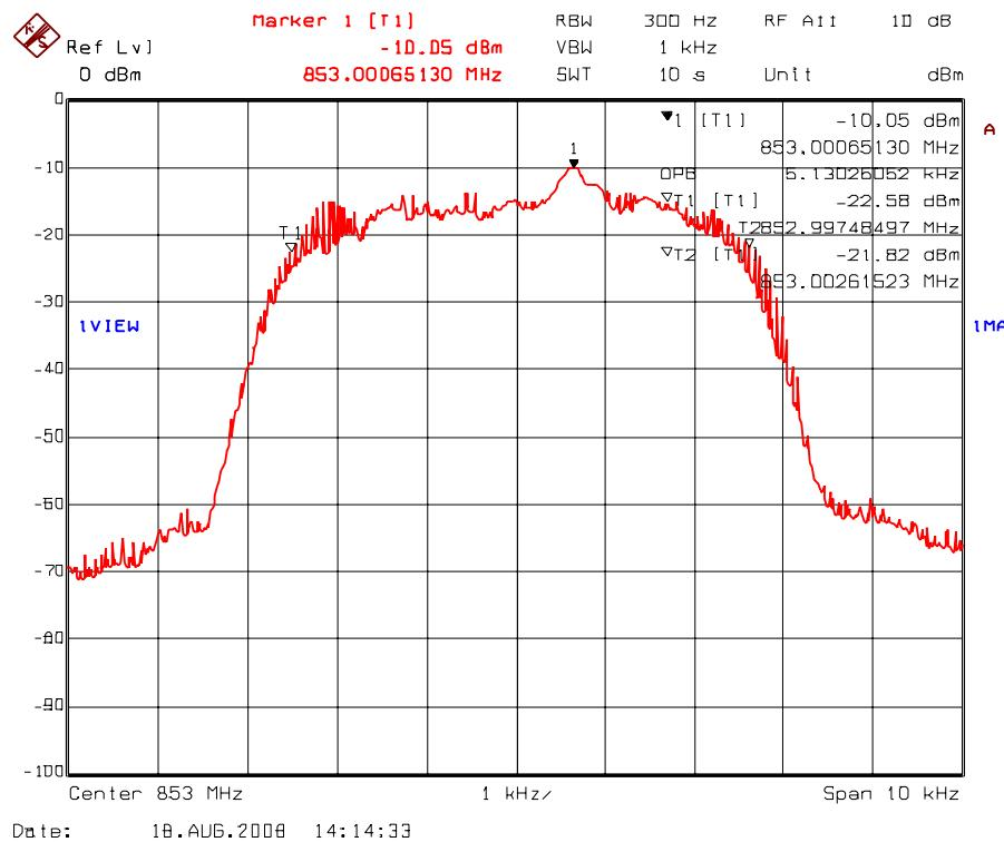
Plot 5.7.4.1.61. 99% Occupied Bandwidth – RF Input Signal
