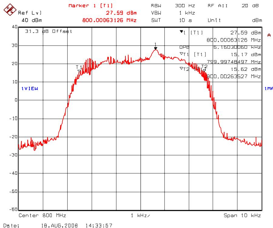
Plot 5.7.4.1.30. 99% Occupied Bandwidth – RF Output Signal
