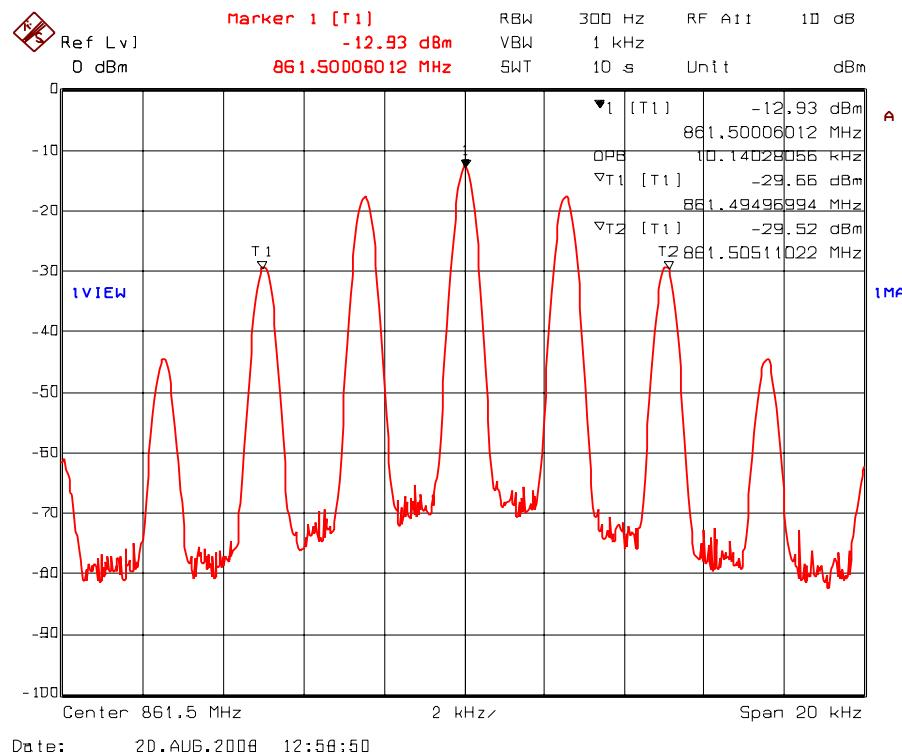
Plot 5.7.4.1.44. 99% Occupied Bandwidth – RF Output Signal
