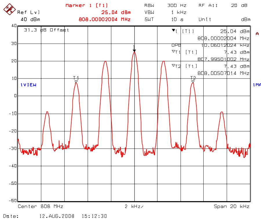
Plot 5.7.4.1.7. 99% Occupied Bandwidth – RF Output Signal
