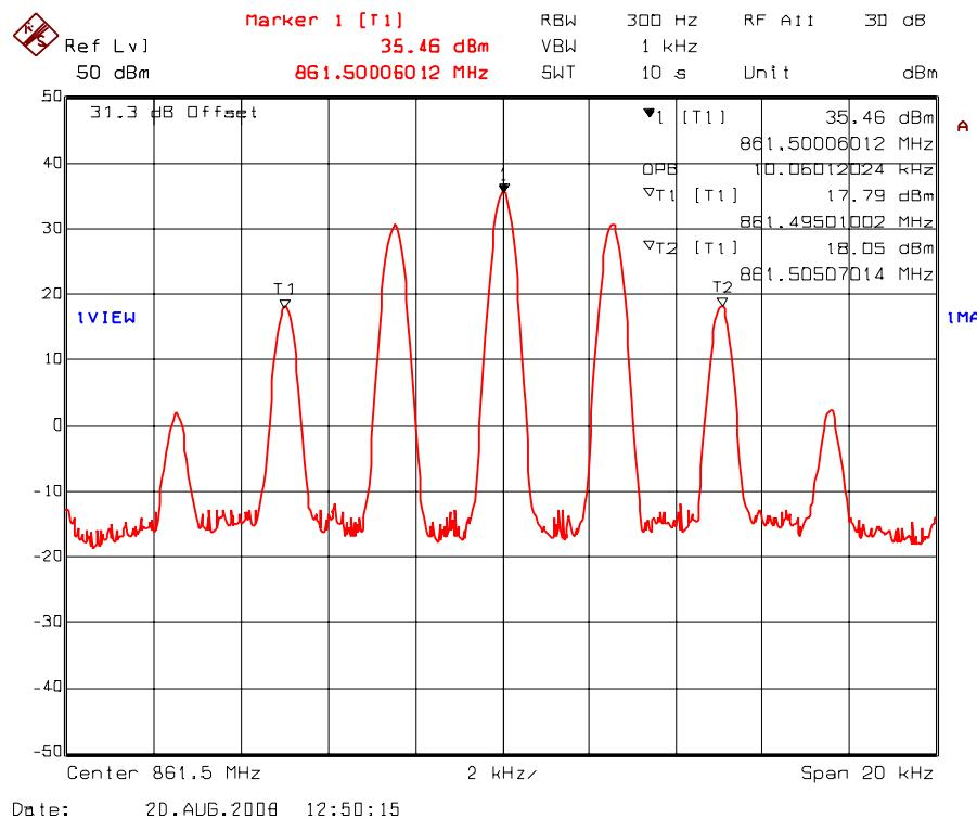
Plot 5.7.4.1.47. 99% Occupied Bandwidth – RF Input Signal
