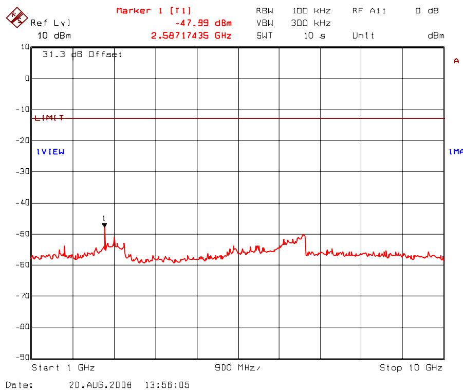
Plot 5.8.5.29. Transmitter antenna conducted RF spurious emissions at antenna port
