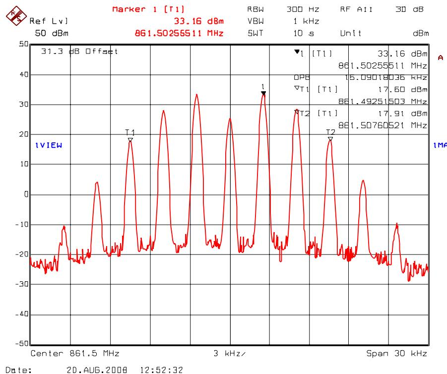
Plot 5.7.4.1.53. 99% Occupied Bandwidth – RF Input Signal
