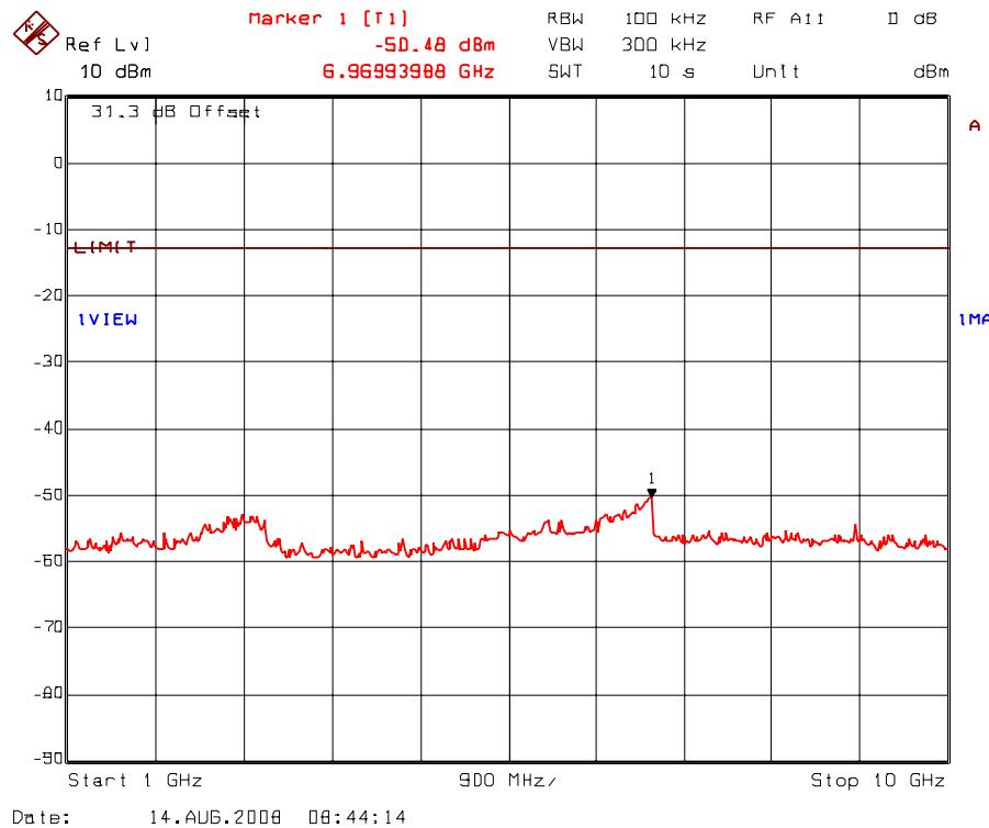
Plot 5.8.5.11. Transmitter antenna conducted RF spurious emissions at antenna port
