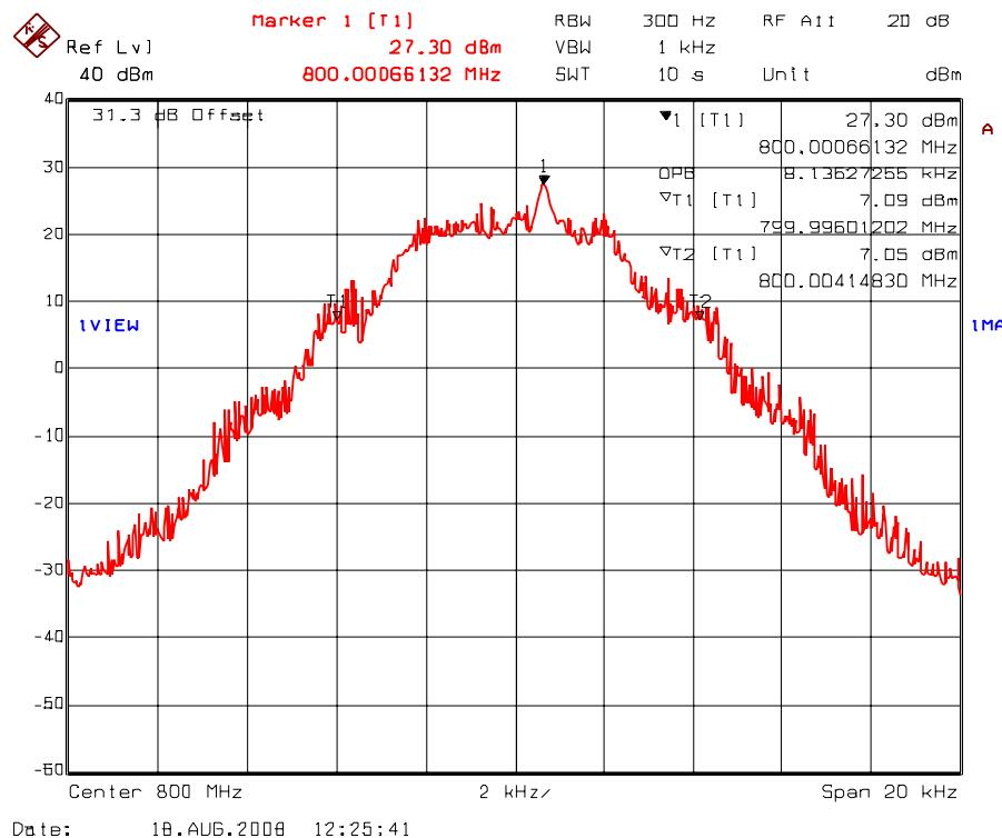
Plot 5.7.4.1.22. 99% Occupied Bandwidth – RF Output Signal
