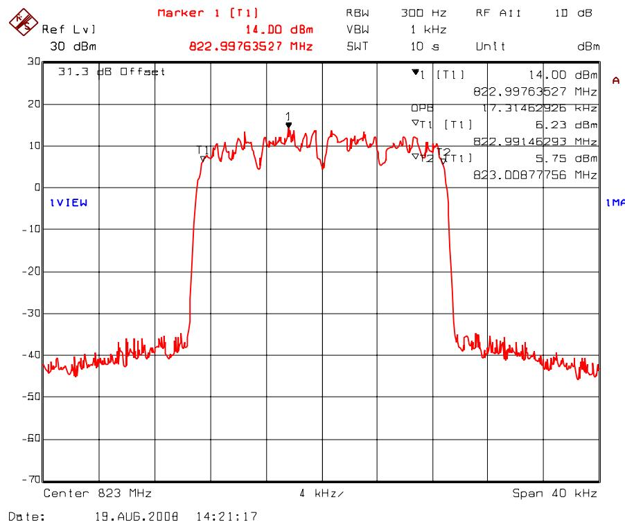
Plot 5.7.4.1.41. 99% Occupied Bandwidth – RF Input Signal
