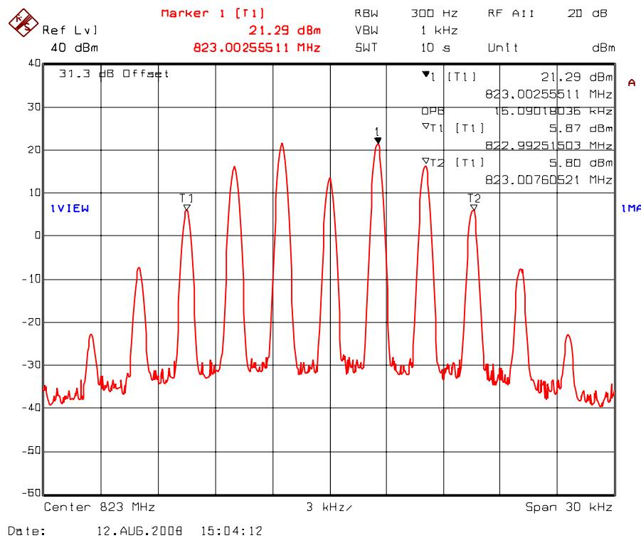
Plot 5.7.4.1.17. 99% Occupied Bandwidth – RF Input Signal
