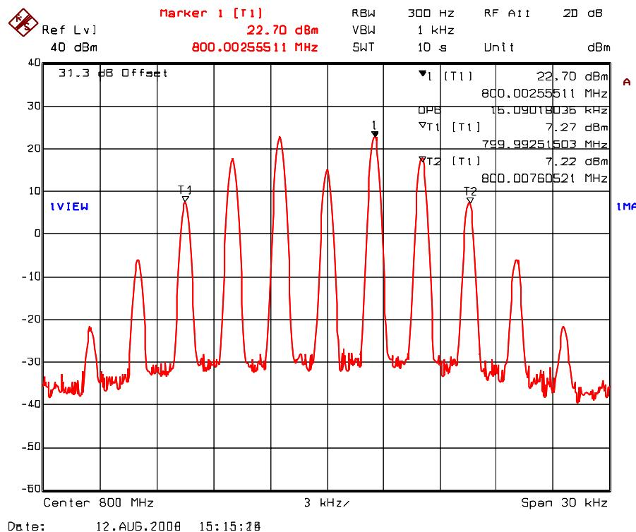
Plot 5.7.4.1.14. 99% Occupied Bandwidth – RF Output Signal
