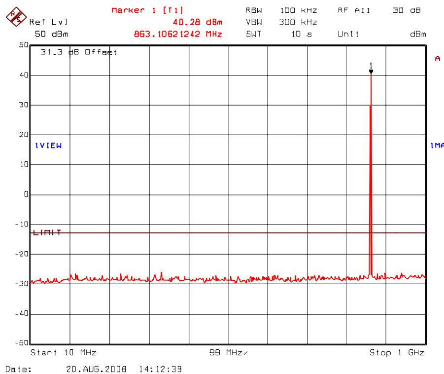
Plot 5.8.5.42. Transmitter antenna conducted RF spurious emissions at antenna port
