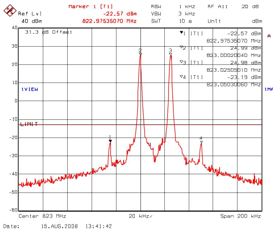
**Plot 5.5.4.2.5. Intermodulation with 3 RF signal inputs/outputs**
