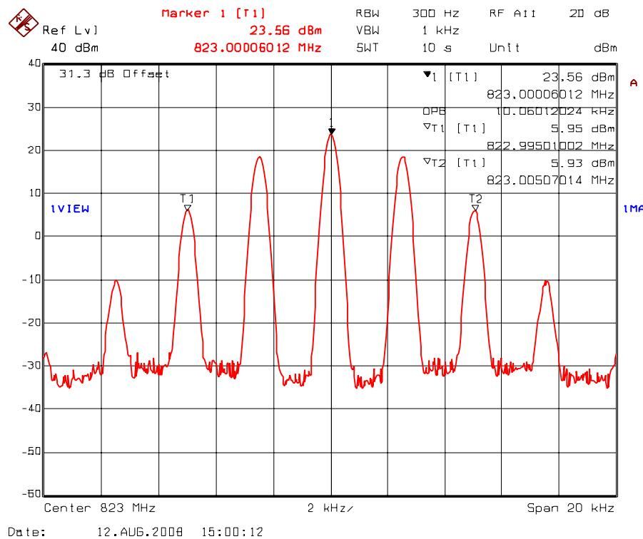
Plot 5.7.4.1.9. 99% Occupied Bandwidth – RF Input Signal
