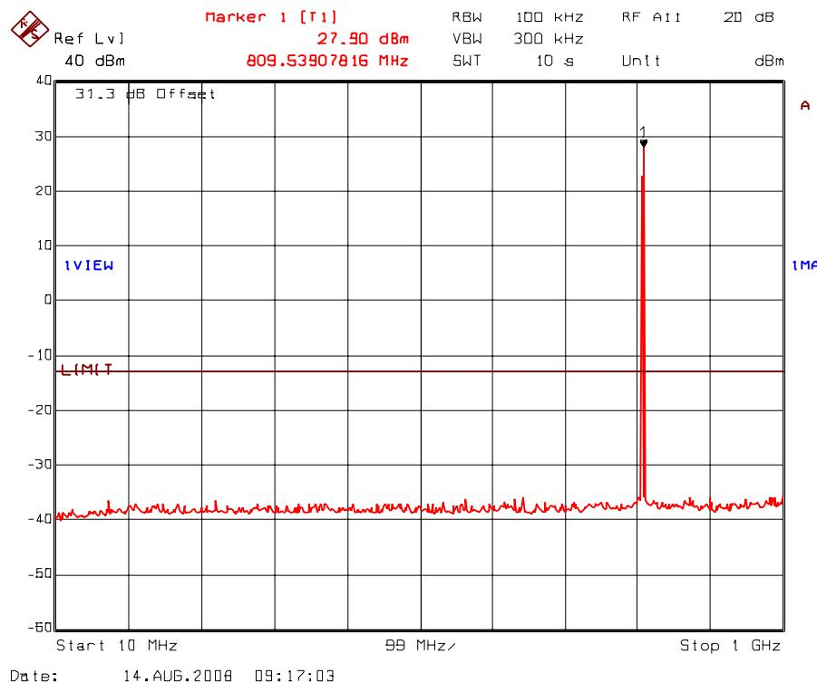
Plot 5.8.5.4. Transmitter antenna conducted RF spurious emissions at antenna port
