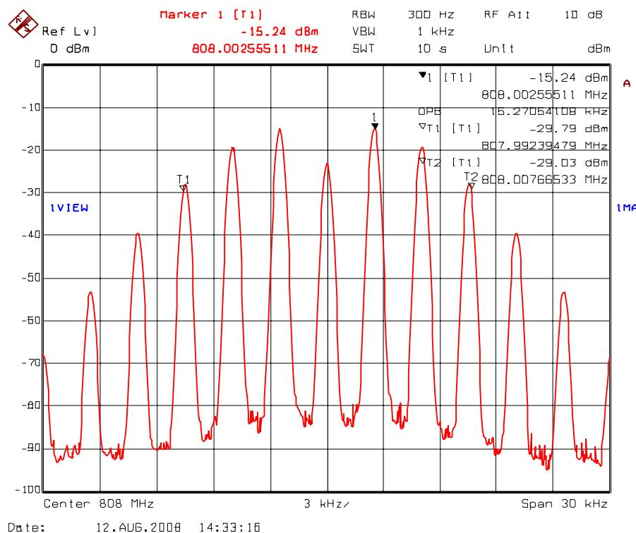
Plot 5.7.4.1.11. 99% Occupied Bandwidth – RF Input Signal
