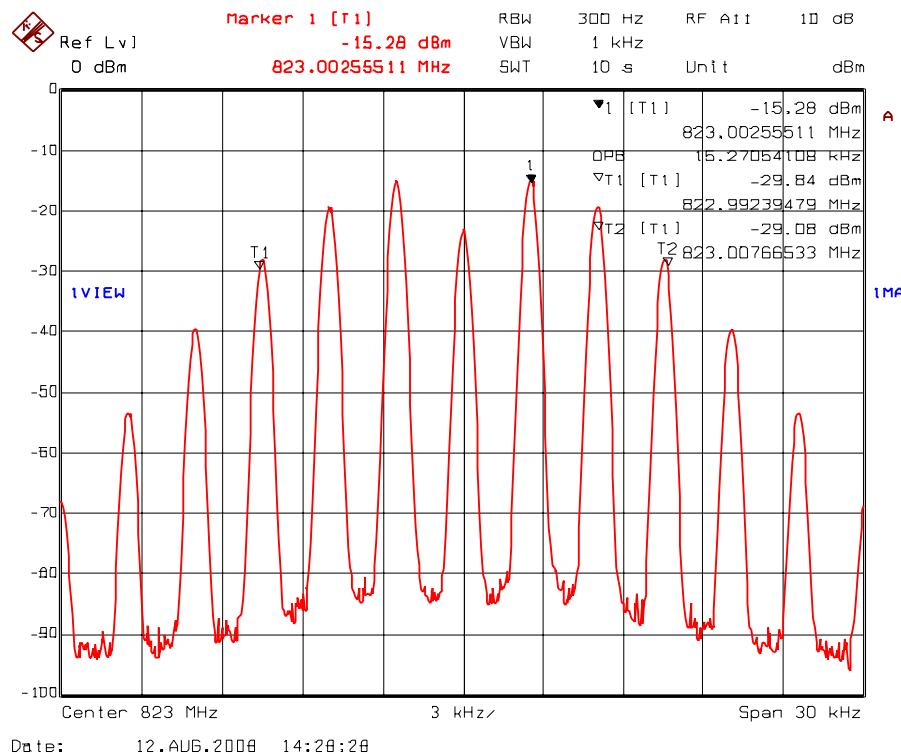
Plot 5.7.4.1.13. 99% Occupied Bandwidth – RF Output Signal
