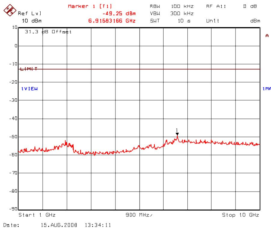
Plot 5.8.5.21. Transmitter antenna conducted RF spurious emissions at antenna port
