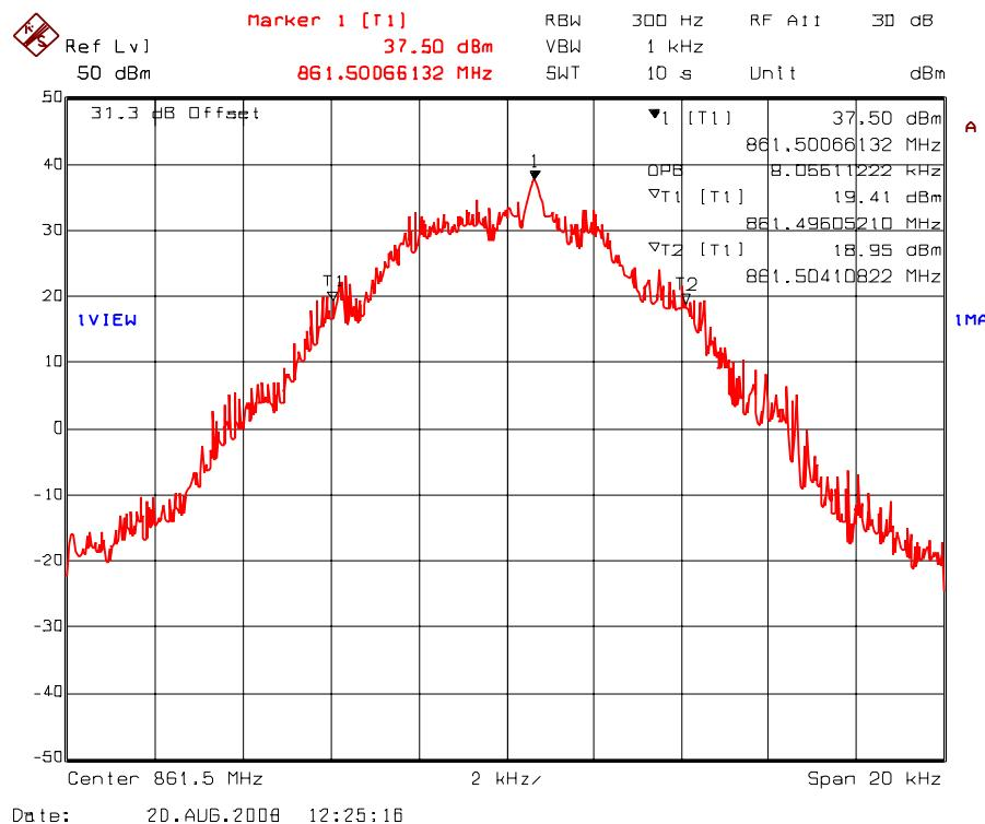
Plot 5.7.4.1.59. 99% Occupied Bandwidth – RF Input Signal
