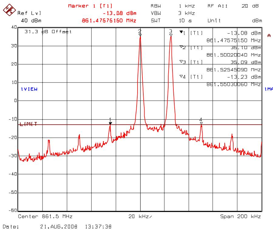
**Plot 5.5.4.2.12. Intermodulation with 3 RF signal inputs/outputs**
