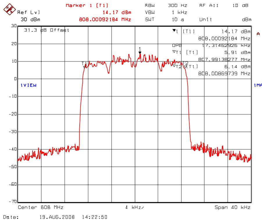
Plot 5.7.4.1.39. 99% Occupied Bandwidth – RF Output Signal
