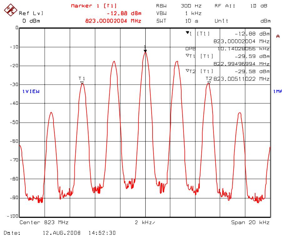
Plot 5.7.4.1.5. 99% Occupied Bandwidth – RF Output Signal
