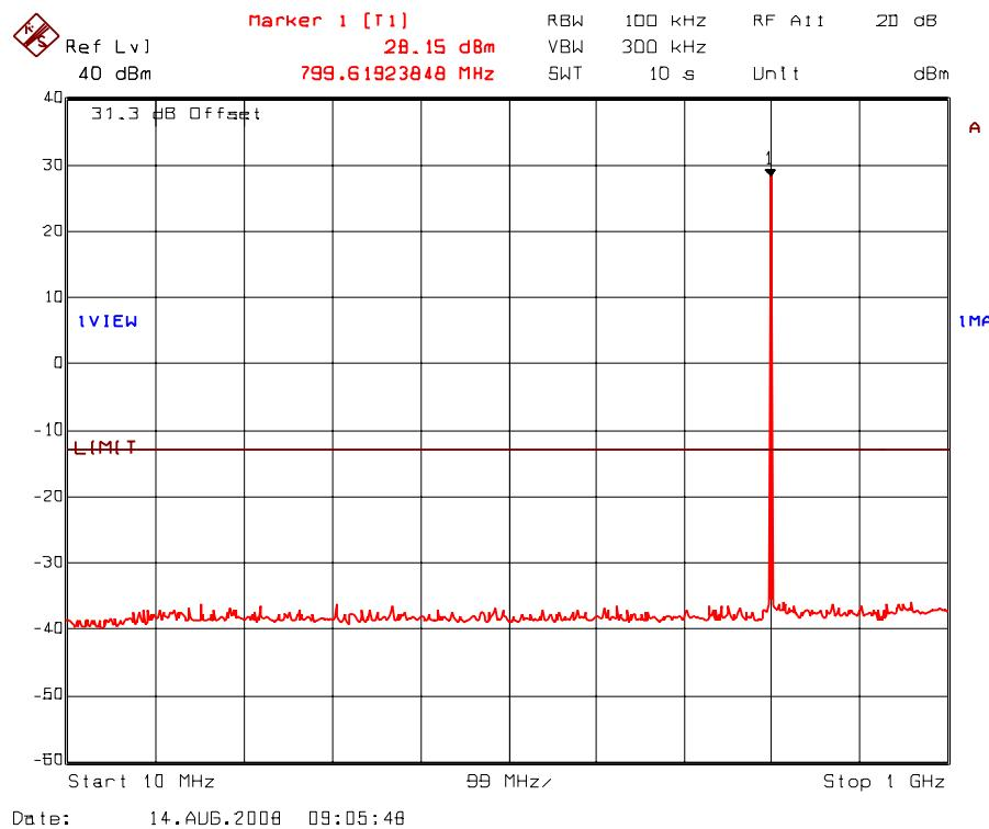
Plot 5.8.5.2. Transmitter antenna conducted RF spurious emissions at antenna port
