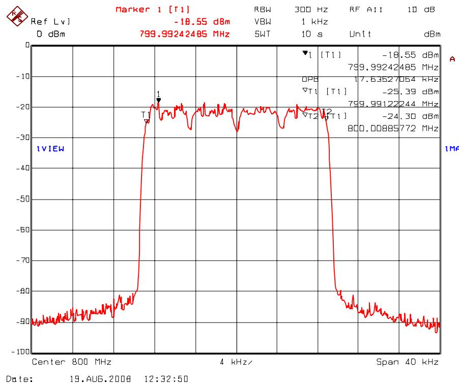
Plot 5.7.4.1.34. 99% Occupied Bandwidth – RF Input Signal
