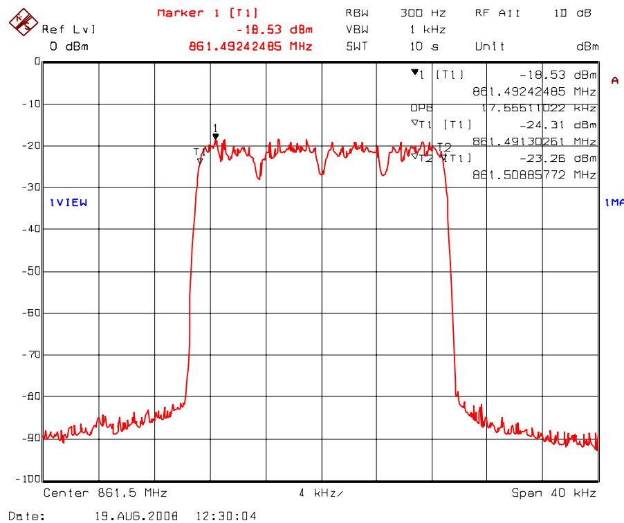
Plot 5.7.4.1.68. 99% Occupied Bandwidth – RF Output Signal
