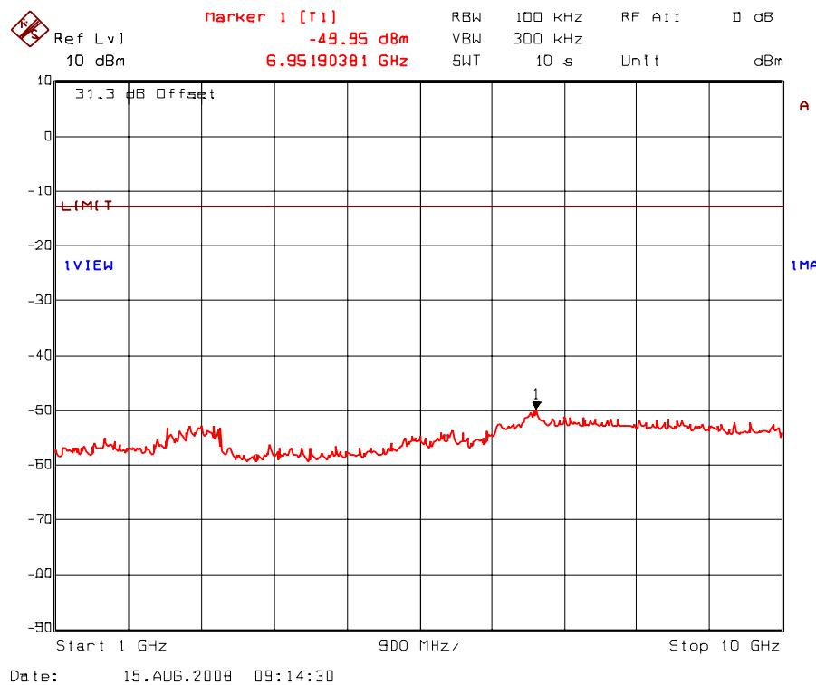
Plot 5.8.5.37. Transmitter antenna conducted RF spurious emissions at antenna port
