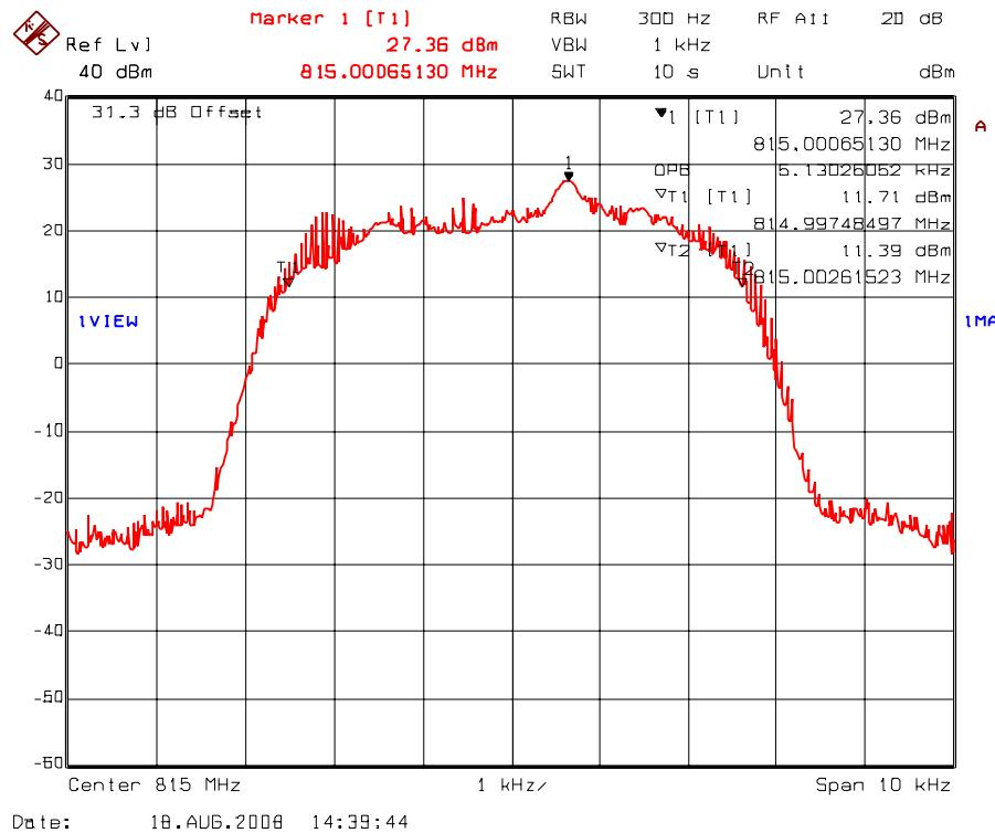
Plot 5.7.4.1.32. 99% Occupied Bandwidth – RF Output Signal
