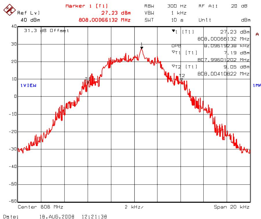
Plot 5.7.4.1.23. 99% Occupied Bandwidth – RF Output Signal
