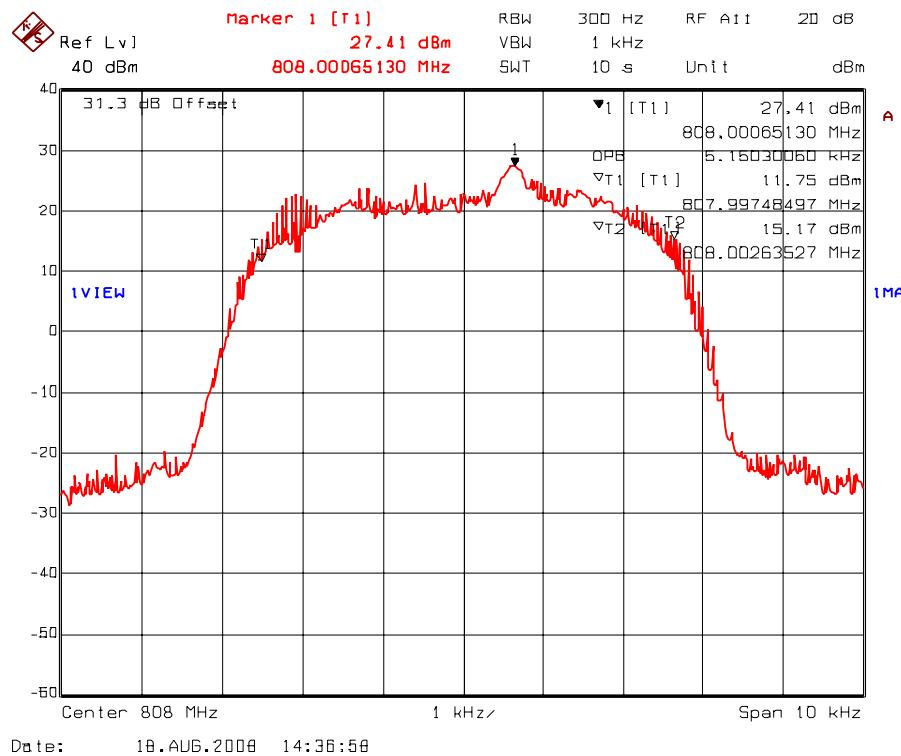
Plot 5.7.4.1.31. 99% Occupied Bandwidth – RF Output Signal
