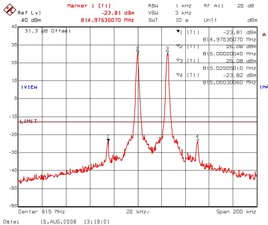
**Plot 5.5.4.2.4. Intermodulation with 2 RF signal inputs/outputs**
