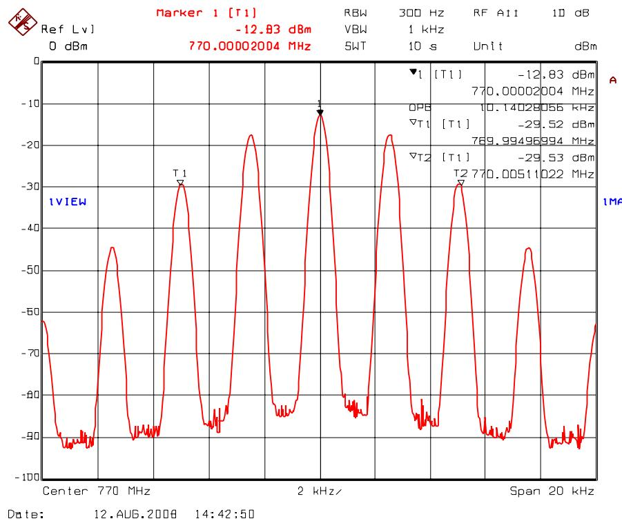
Plot 5.7.4.1.42. 99% Occupied Bandwidth – RF Input Signal
