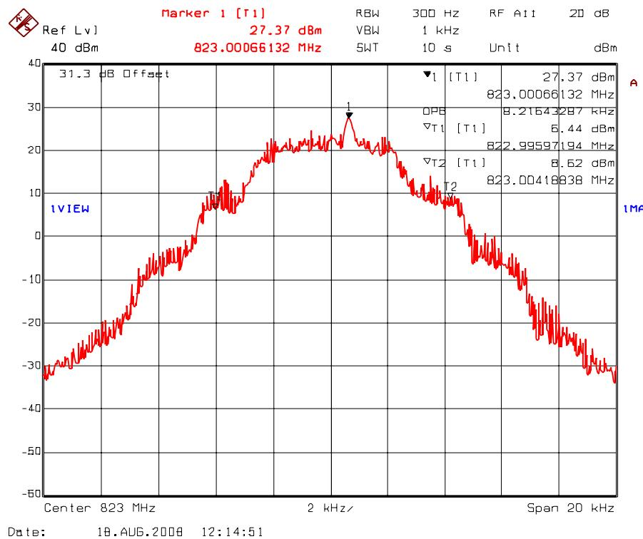
Plot 5.7.4.1.25. 99% Occupied Bandwidth – RF Input Signal
