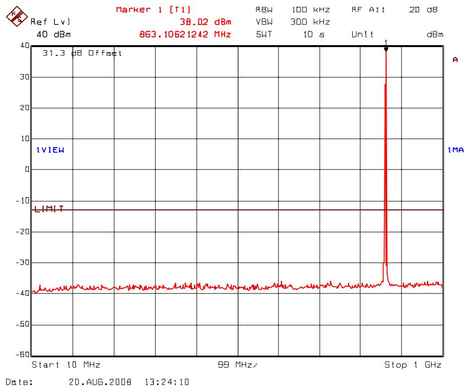
Plot 5.8.5.14. Transmitter antenna conducted RF spurious emissions at antenna port
