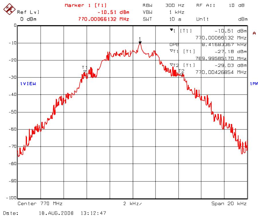
Plot 5.7.4.1.54. 99% Occupied Bandwidth – RF Input Signal
