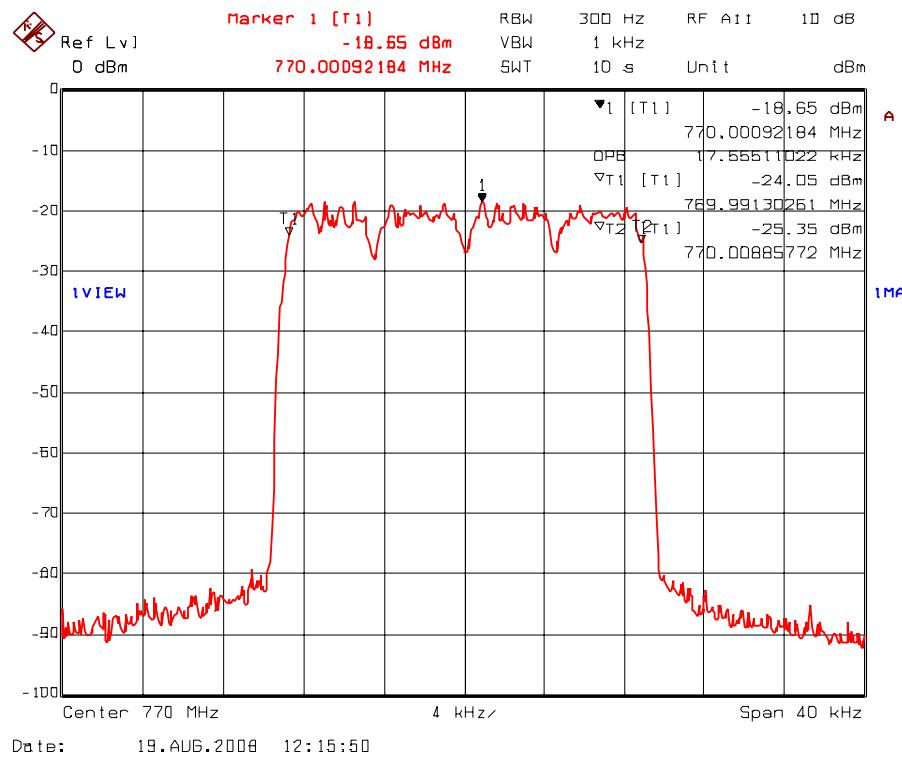
Plot 5.7.4.1.66. 99% Occupied Bandwidth – RF Input Signal
