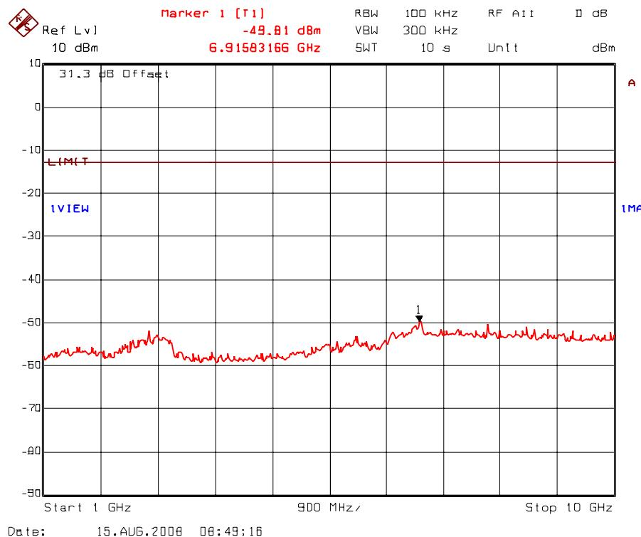
Plot 5.8.5.33. Transmitter antenna conducted RF spurious emissions at antenna port
