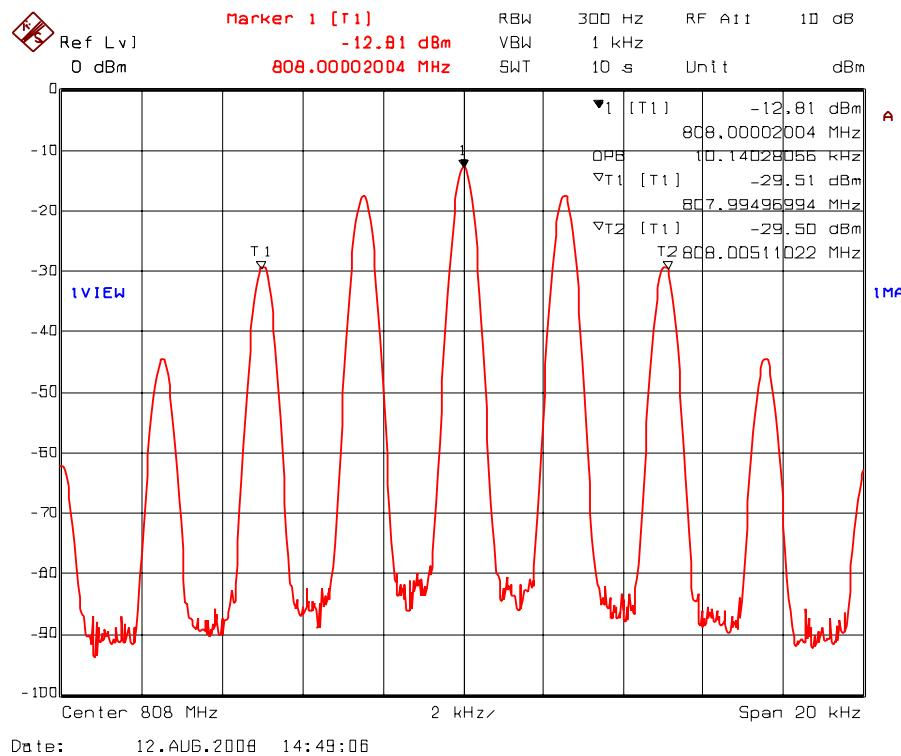
Plot 5.7.4.1.3. 99% Occupied Bandwidth – RF Input Signal
