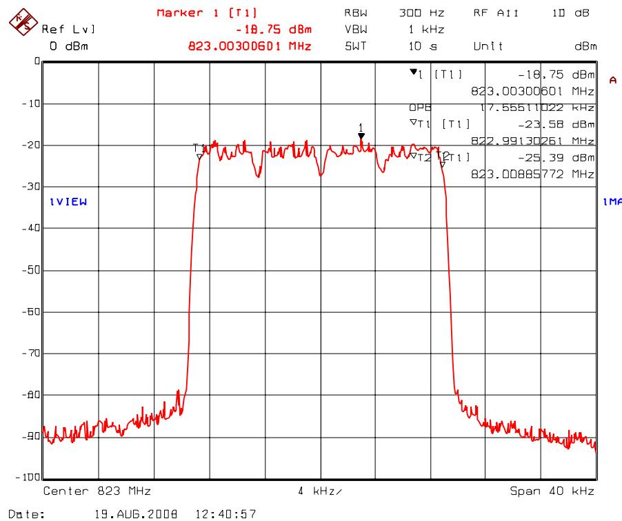
Plot 5.7.4.1.37. 99% Occupied Bandwidth – RF Output Signal
