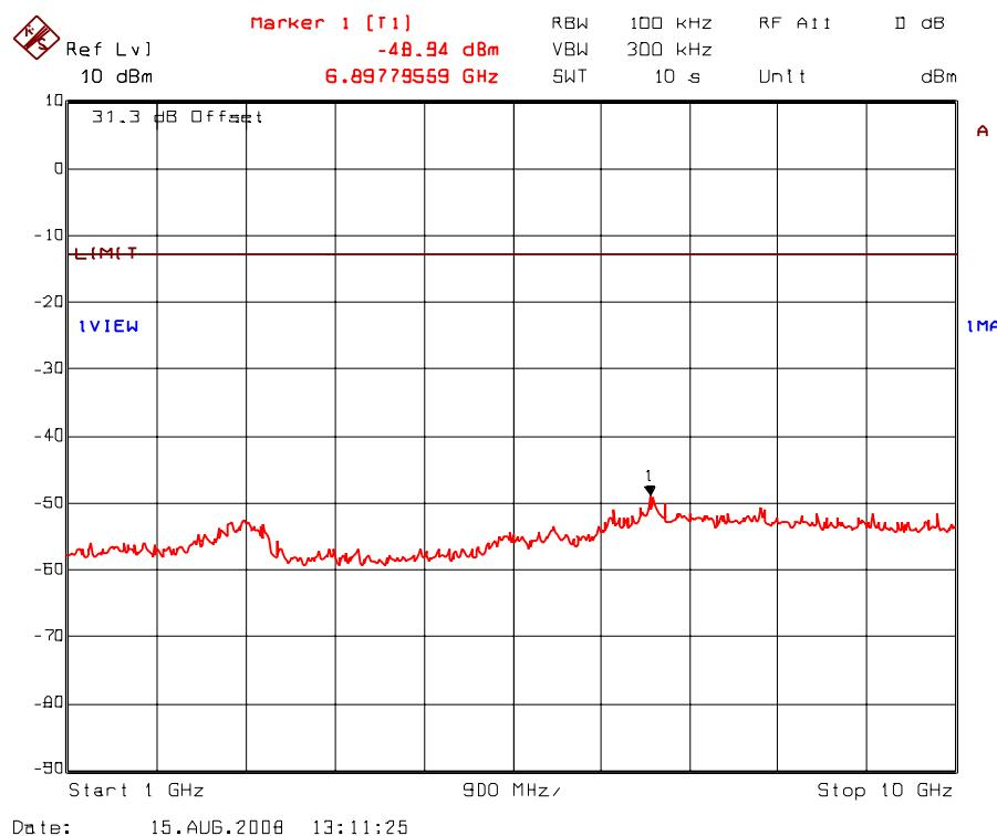
Plot 5.8.5.19. Transmitter antenna conducted RF spurious emissions at antenna port
