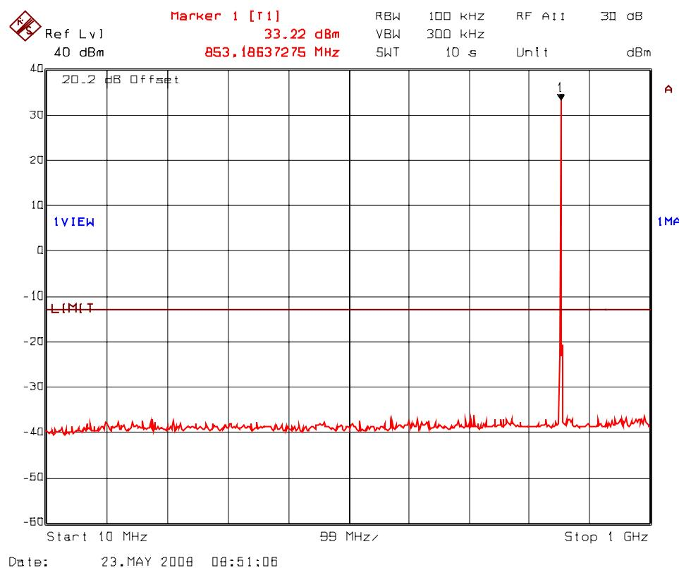
**PLOT # 40(b) Transmitter Antenna Conducted RF Spurious Emissions @ Antenna Port
