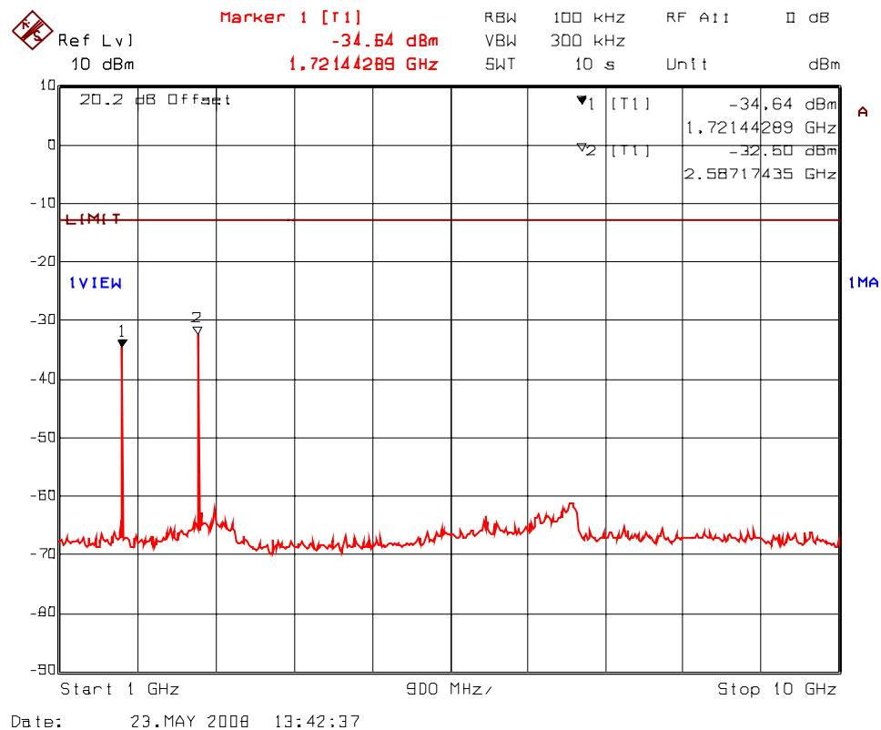
**PLOT # 45(a): Transmitter Antenna Conducted RF Spurious Emissions @ Antenna Port
