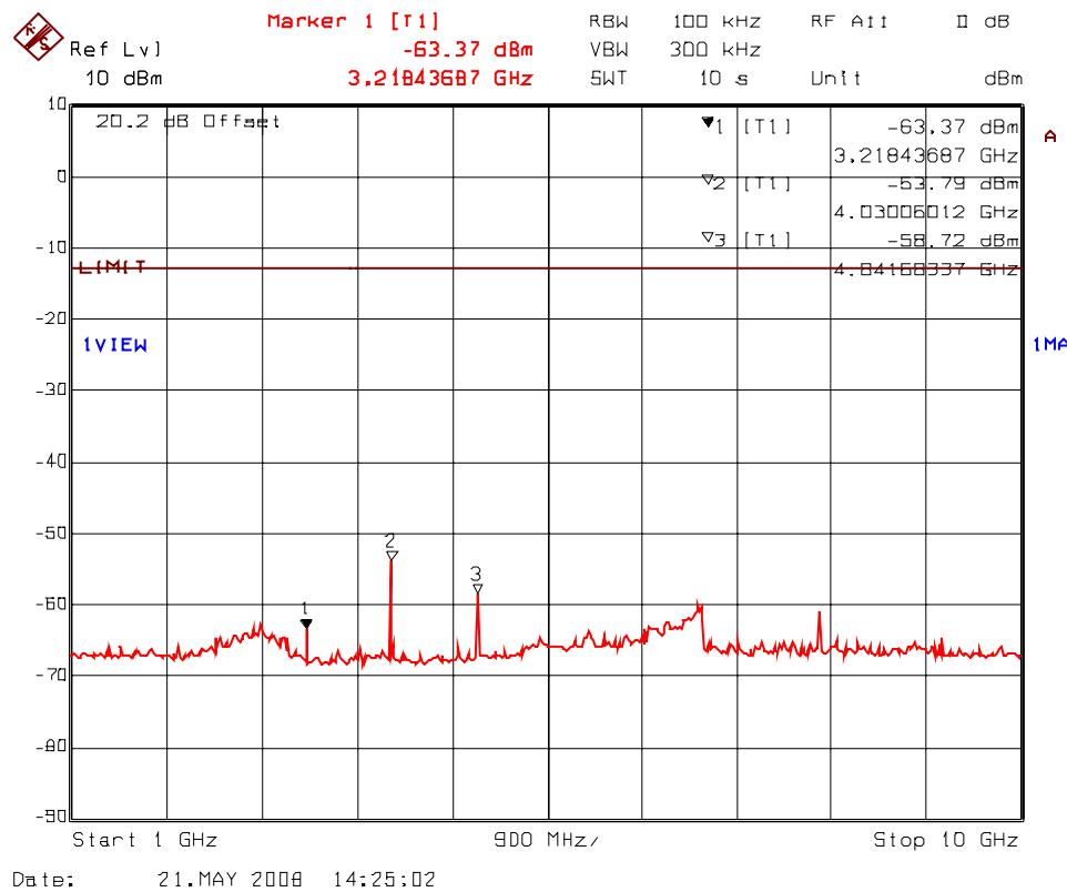
**PLOT # 47(a): Transmitter Antenna Conducted RF Spurious Emissions @ Antenna Port
