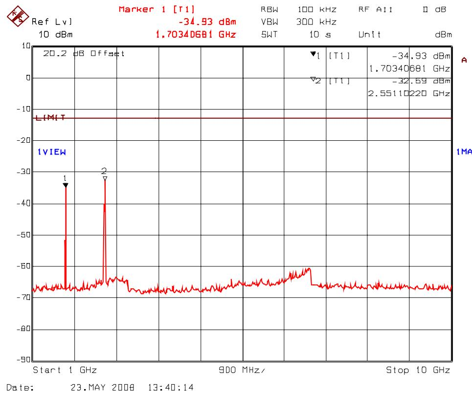
**PLOT # 44(a): Transmitter Antenna Conducted RF Spurious Emissions @ Antenna Port
