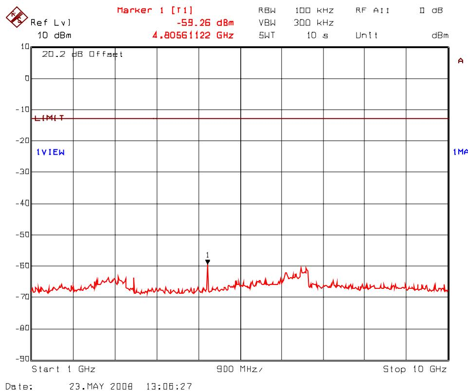
**PLOT # 54(a): Transmitter Antenna Conducted RF Spurious Emissions @ Antenna Port
