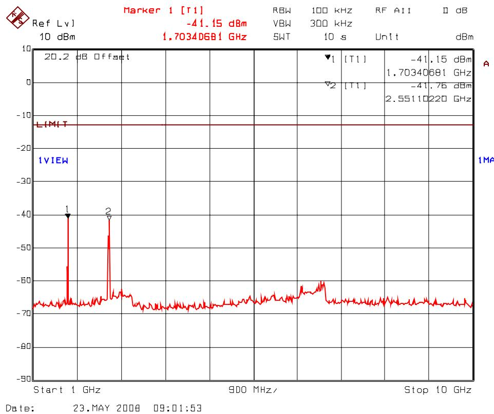
**PLOT # 41(a): Transmitter Antenna Conducted RF Spurious Emissions @ Antenna Port
