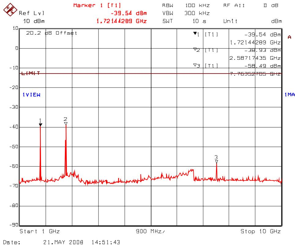
**PLOT # 39(a): Transmitter Antenna Conducted RF Spurious Emissions @ Antenna Port
