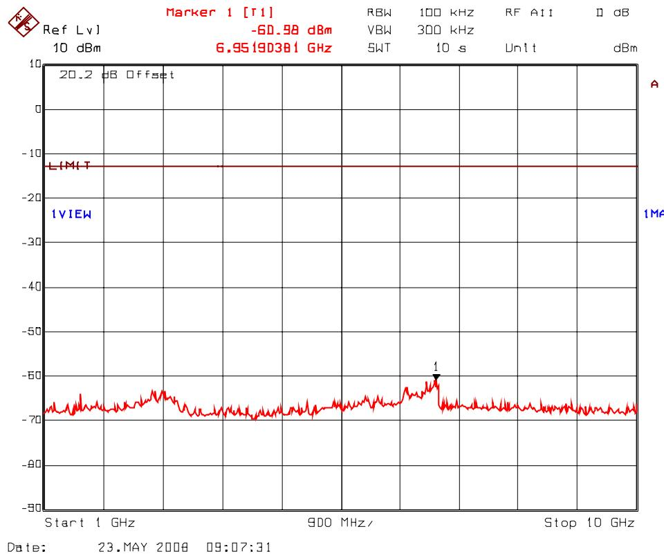
**PLOT # 40(a): Transmitter Antenna Conducted RF Spurious Emissions @ Antenna Port
