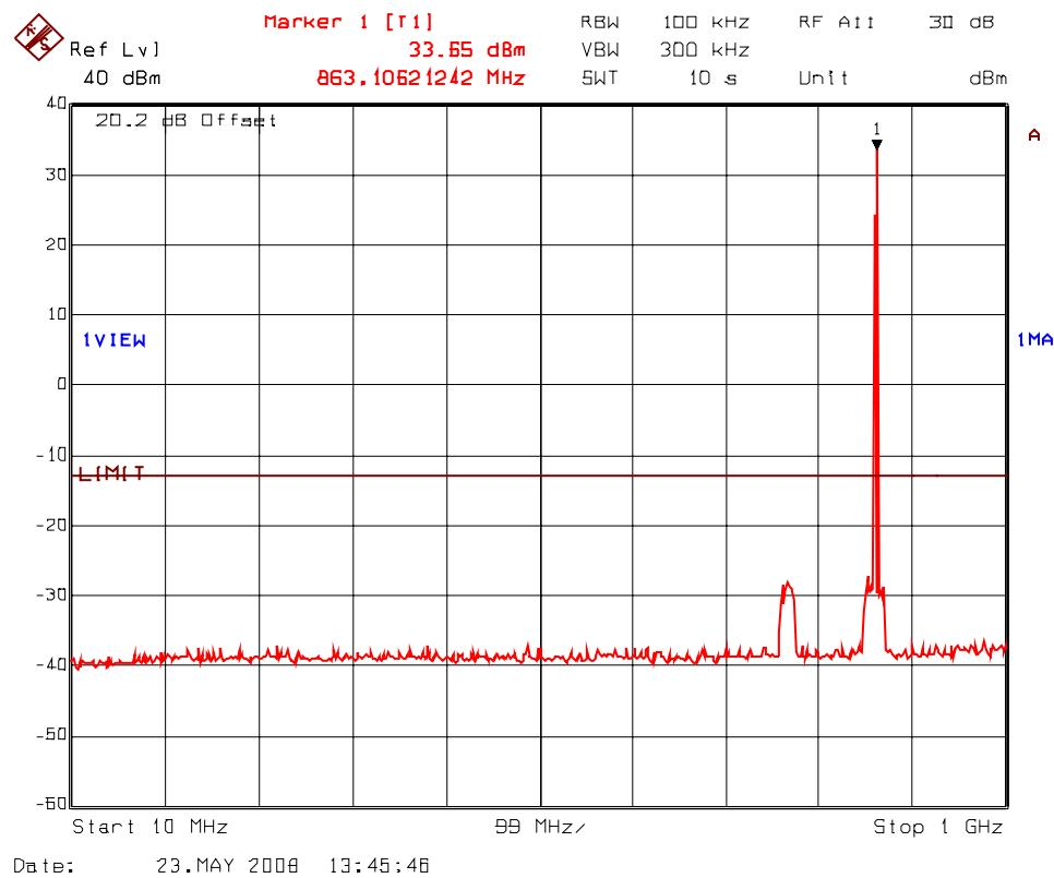
**PLOT # 44(b) Transmitter Antenna Conducted RF Spurious Emissions @ Antenna Port
