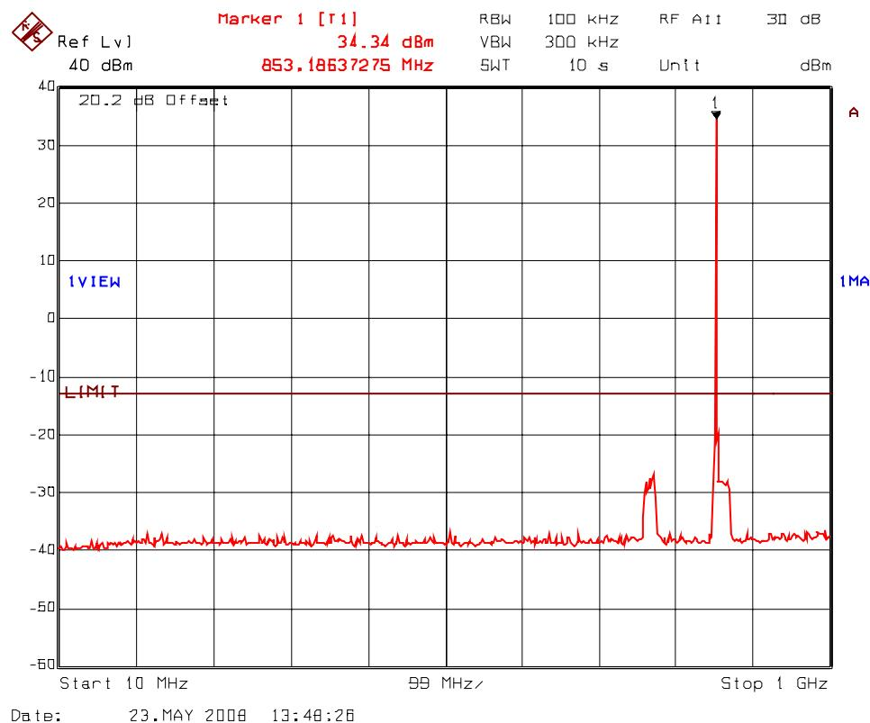
**PLOT # 43(b) Transmitter Antenna Conducted RF Spurious Emissions @ Antenna Port
