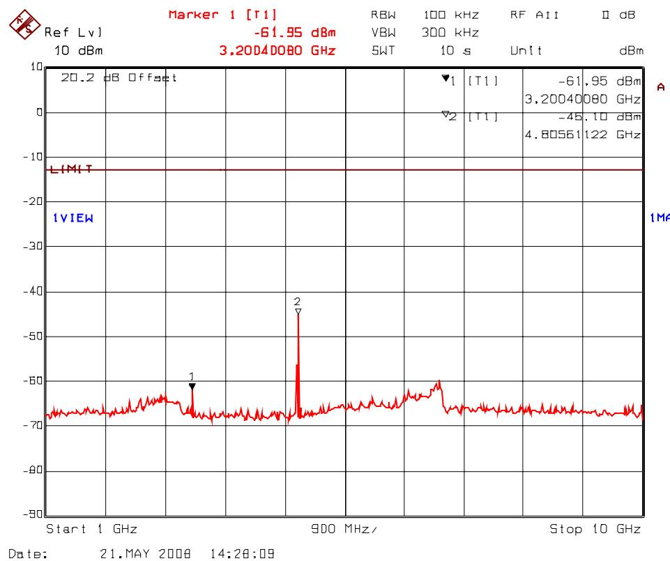
**PLOT # 46(a): Transmitter Antenna Conducted RF Spurious Emissions @ Antenna Port
