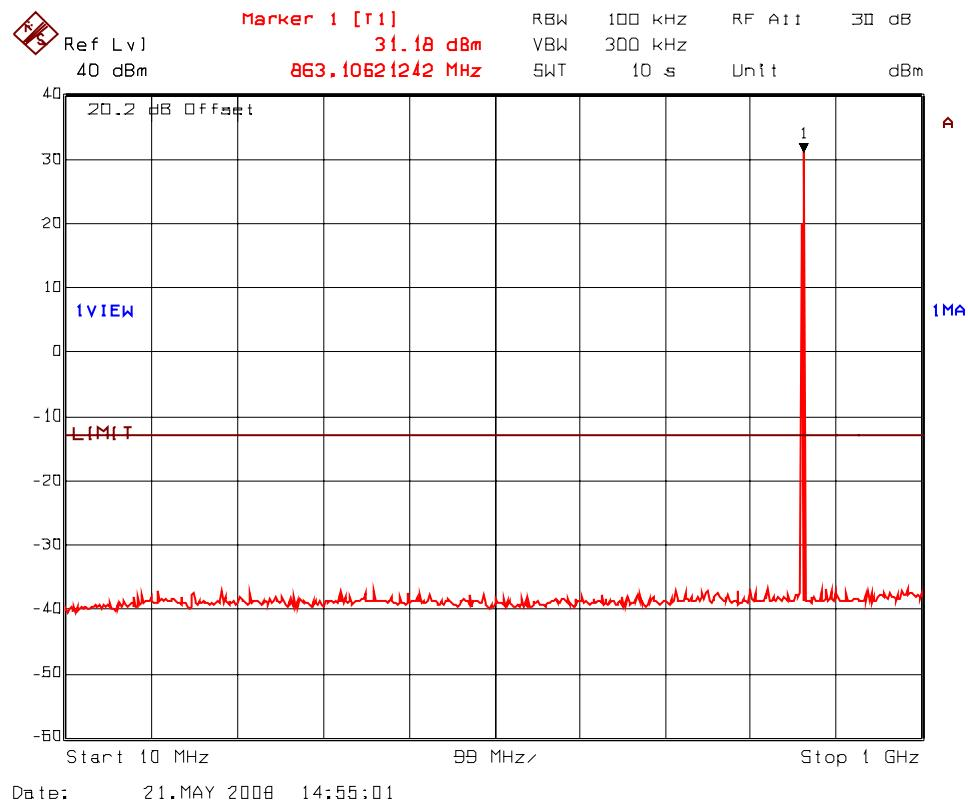
**PLOT # 38(b) Transmitter Antenna Conducted RF Spurious Emissions @ Antenna Port
