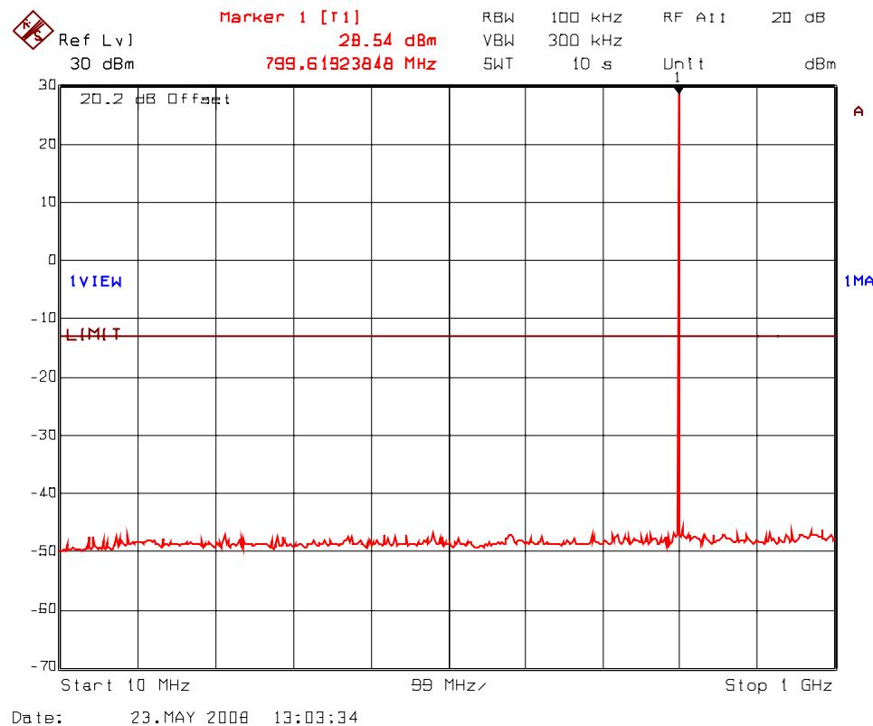
**PLOT # 53(b) Transmitter Antenna Conducted RF Spurious Emissions @ Antenna Port
