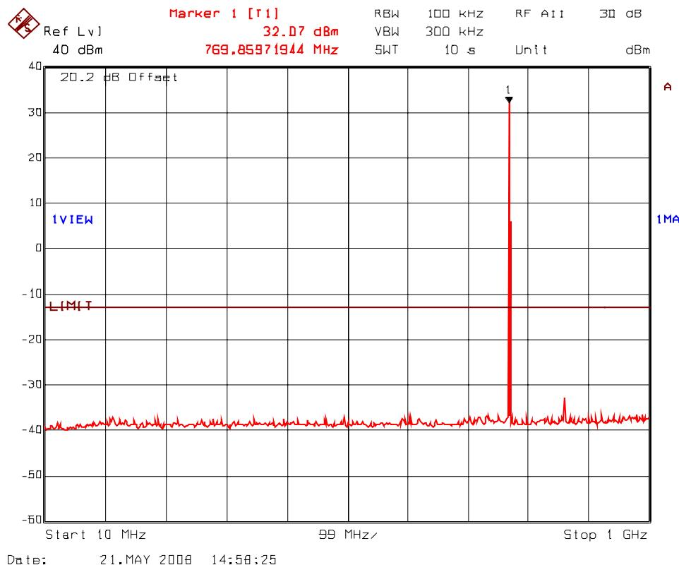
**PLOT # 36(b) Transmitter Antenna Conducted RF Spurious Emissions @ Antenna Port
