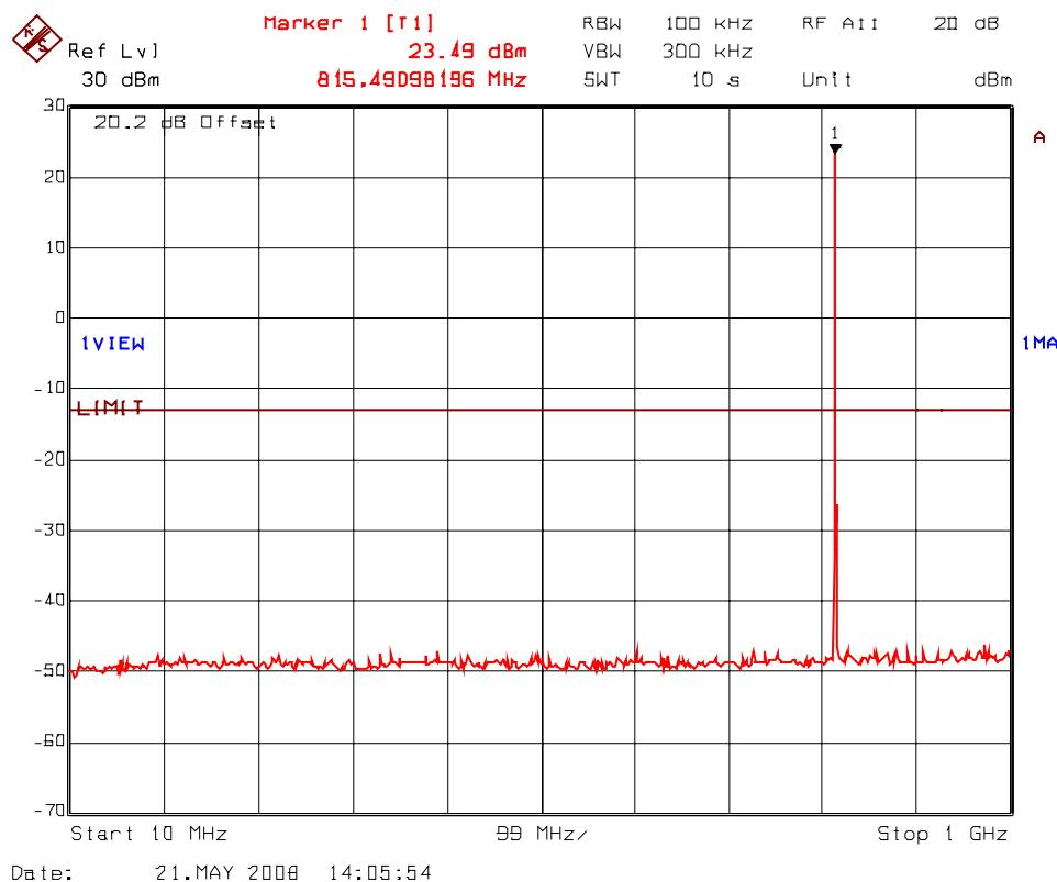
**PLOT # 47(b) Transmitter Antenna Conducted RF Spurious Emissions @ Antenna Port
