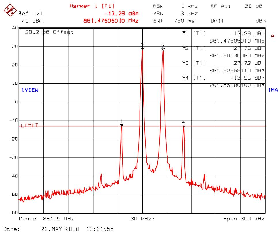
**PLOT#:** 4      **Intermodulation with 3 RF signal inputs/outputs**
