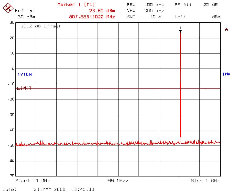
**PLOT # 46(b) Transmitter Antenna Conducted RF Spurious Emissions @ Antenna Port
