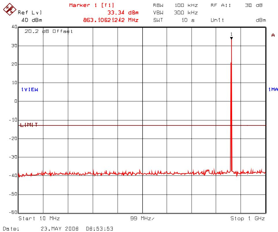
**PLOT # 41(b) Transmitter Antenna Conducted RF Spurious Emissions @ Antenna Port
