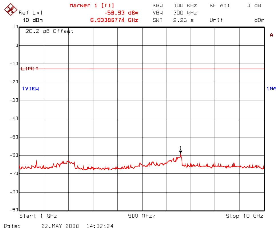
**PLOT # 53(a): Transmitter Antenna Conducted RF Spurious Emissions @ Antenna Port
