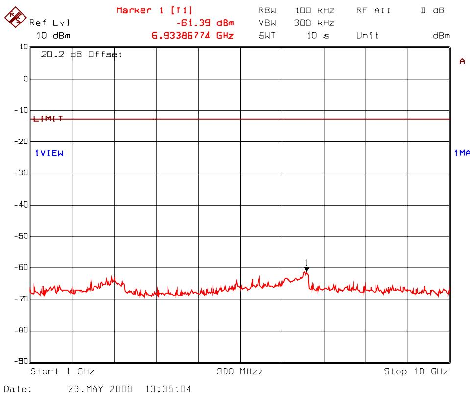
**PLOT # 43(a): Transmitter Antenna Conducted RF Spurious Emissions @ Antenna Port
