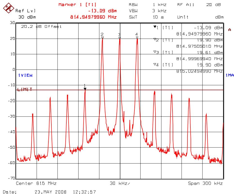
**PLOT#:** 14 **Intermodulation with 3 RF signal inputs/outputs**
