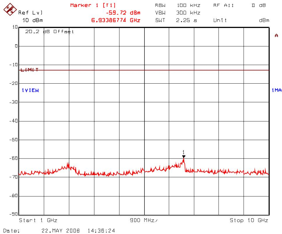
**PLOT # 52(a): Transmitter Antenna Conducted RF Spurious Emissions @ Antenna Port
