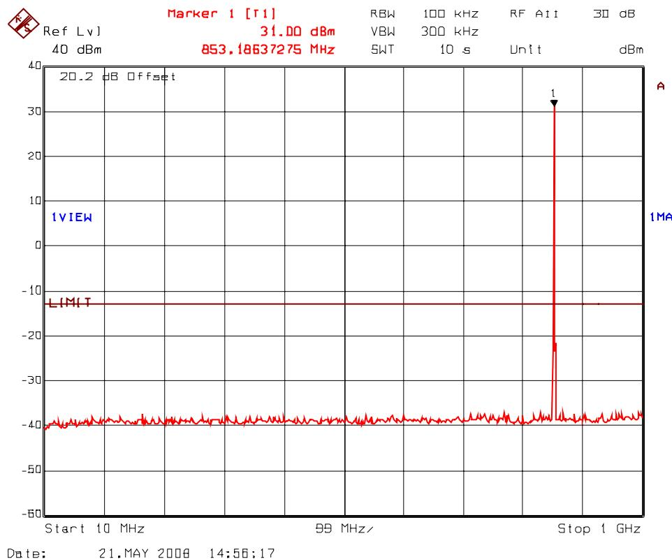
**PLOT # 37(b) Transmitter Antenna Conducted RF Spurious Emissions @ Antenna Port
