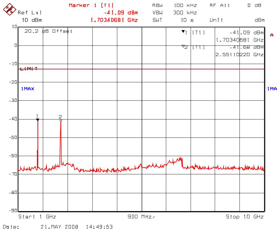
**PLOT # 38(a): Transmitter Antenna Conducted RF Spurious Emissions @ Antenna Port
