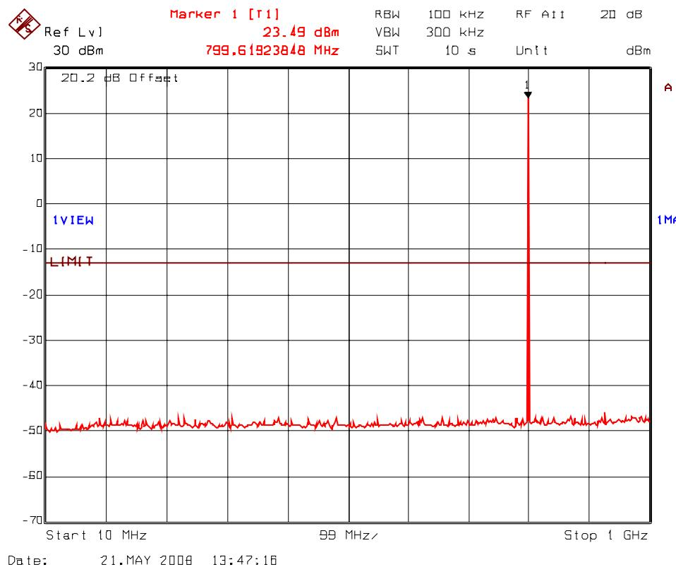
**PLOT # 45(b) Transmitter Antenna Conducted RF Spurious Emissions @ Antenna Port
