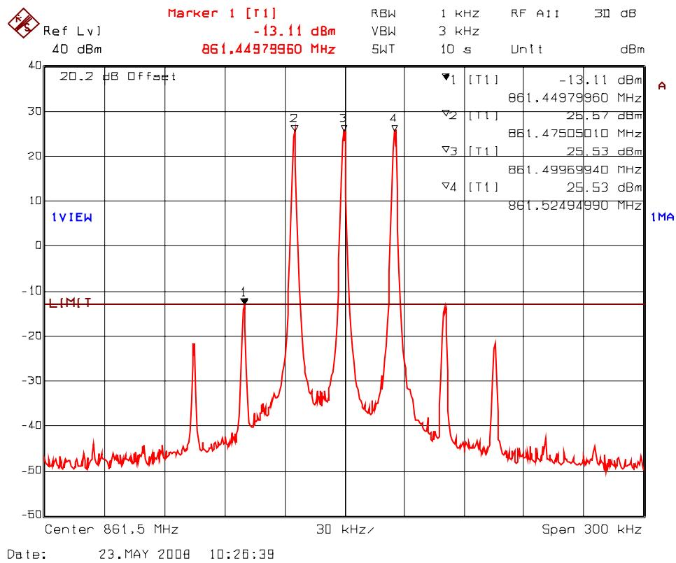
**PLOT#:** 7      **Intermodulation with 2 RF signal inputs/outputs**
