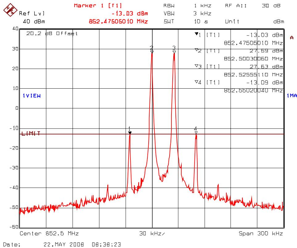
**PLOT#:** 3    **Intermodulation with 2 RF signal inputs/outputs**
