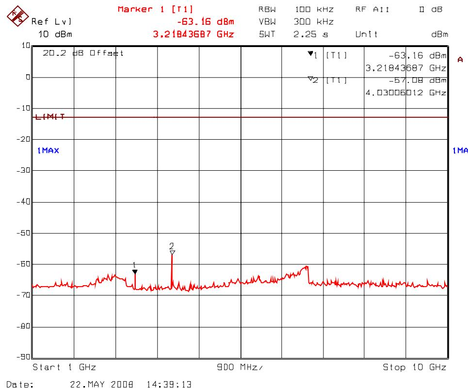
**PLOT # 51(a): Transmitter Antenna Conducted RF Spurious Emissions @ Antenna Port
