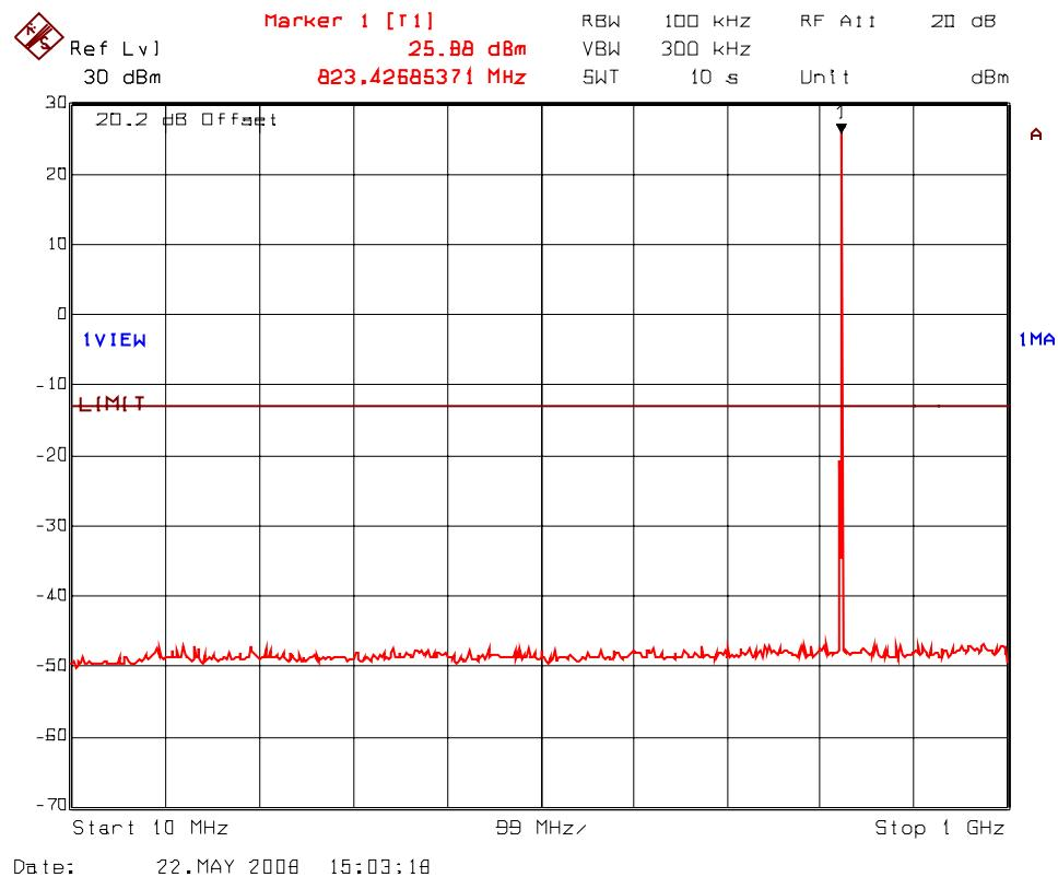
**PLOT # 52(b) Transmitter Antenna Conducted RF Spurious Emissions @ Antenna Port
