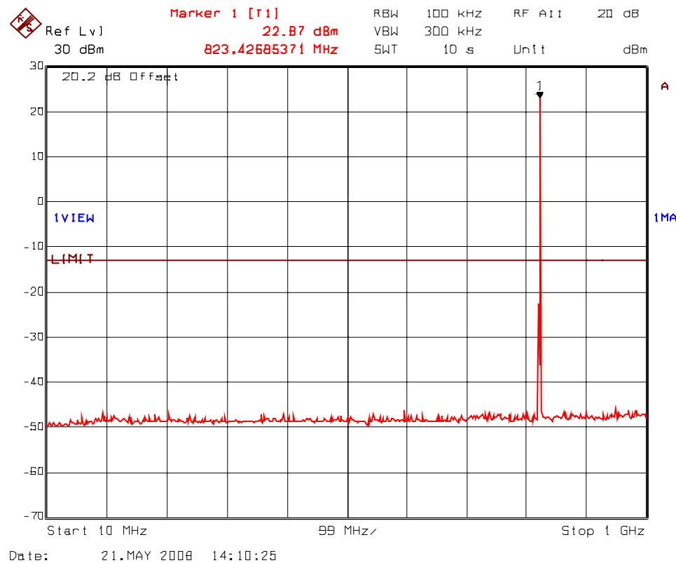
**PLOT # 48(b) Transmitter Antenna Conducted RF Spurious Emissions @ Antenna Port
