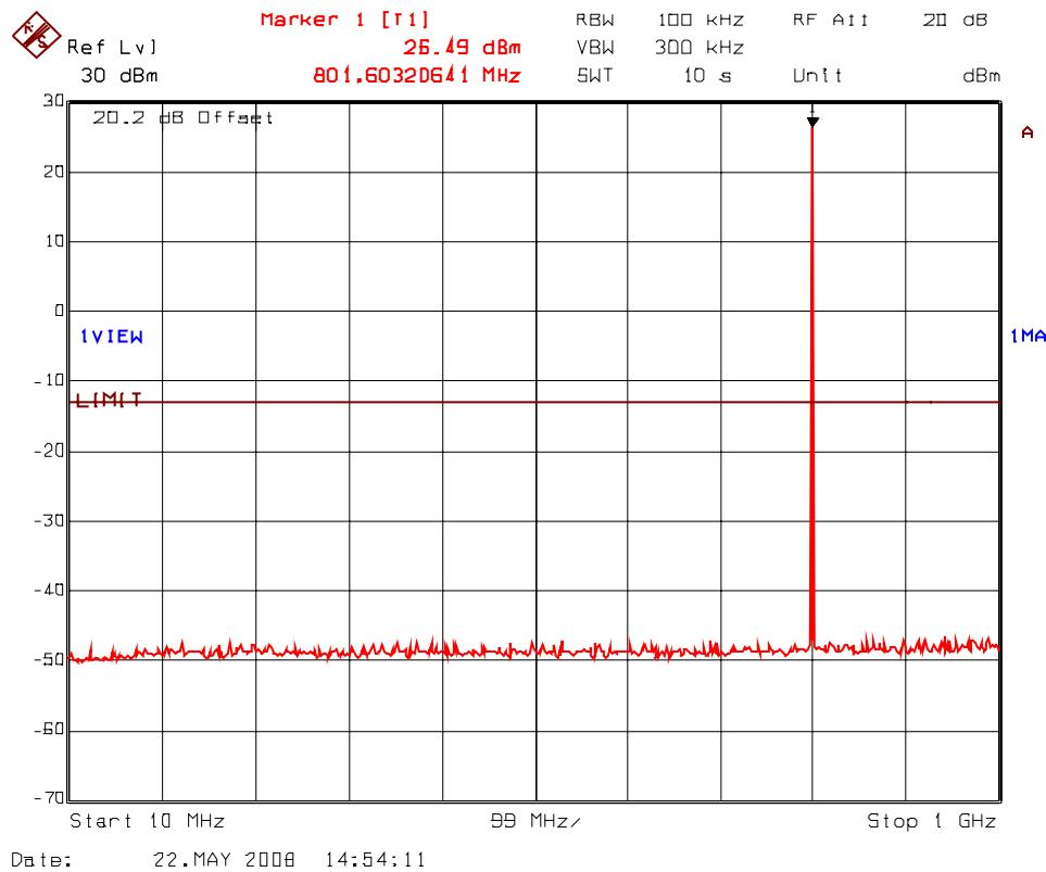
**PLOT # 49(b) Transmitter Antenna Conducted RF Spurious Emissions @ Antenna Port
