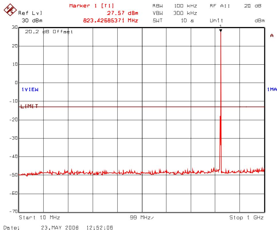
**PLOT # 56(b) Transmitter Antenna Conducted RF Spurious Emissions @ Antenna Port
