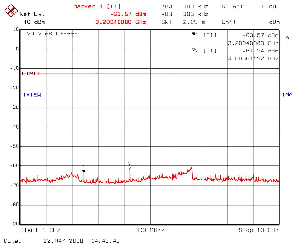
**PLOT # 50(a): Transmitter Antenna Conducted RF Spurious Emissions @ Antenna Port
