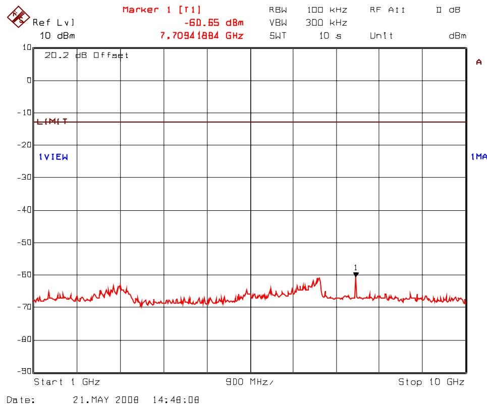
**PLOT # 37(a): Transmitter Antenna Conducted RF Spurious Emissions @ Antenna Port
