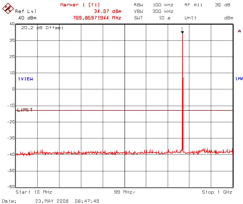
**PLOT # 39(b) Transmitter Antenna Conducted RF Spurious Emissions @ Antenna Port
