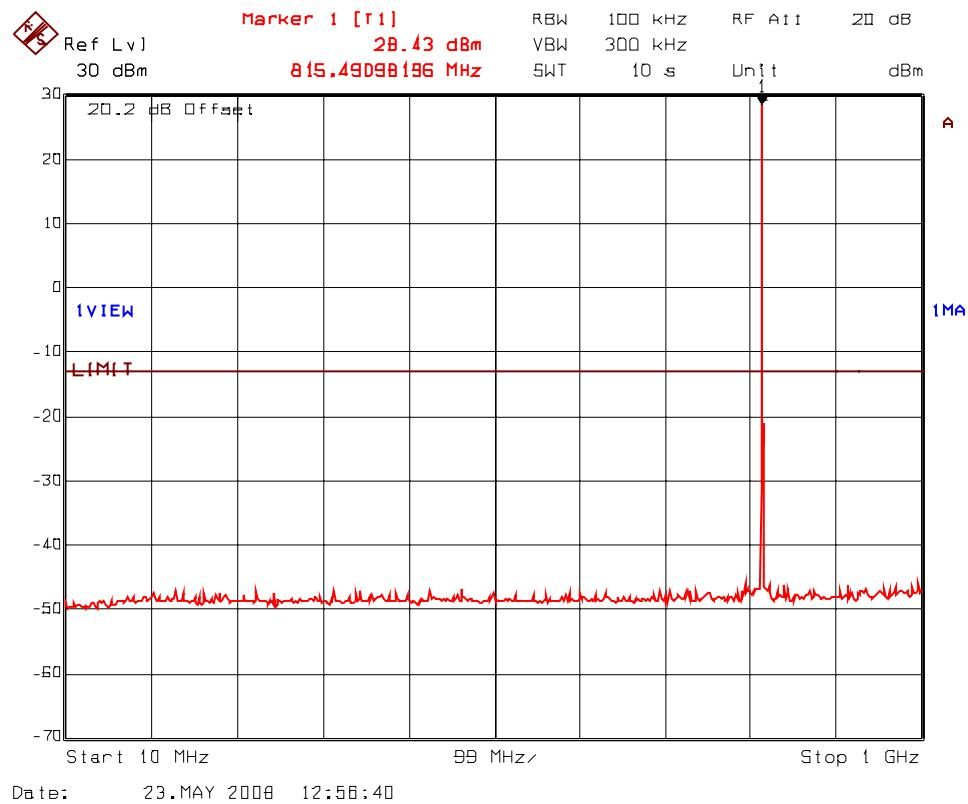
**PLOT # 55(b) Transmitter Antenna Conducted RF Spurious Emissions @ Antenna Port
