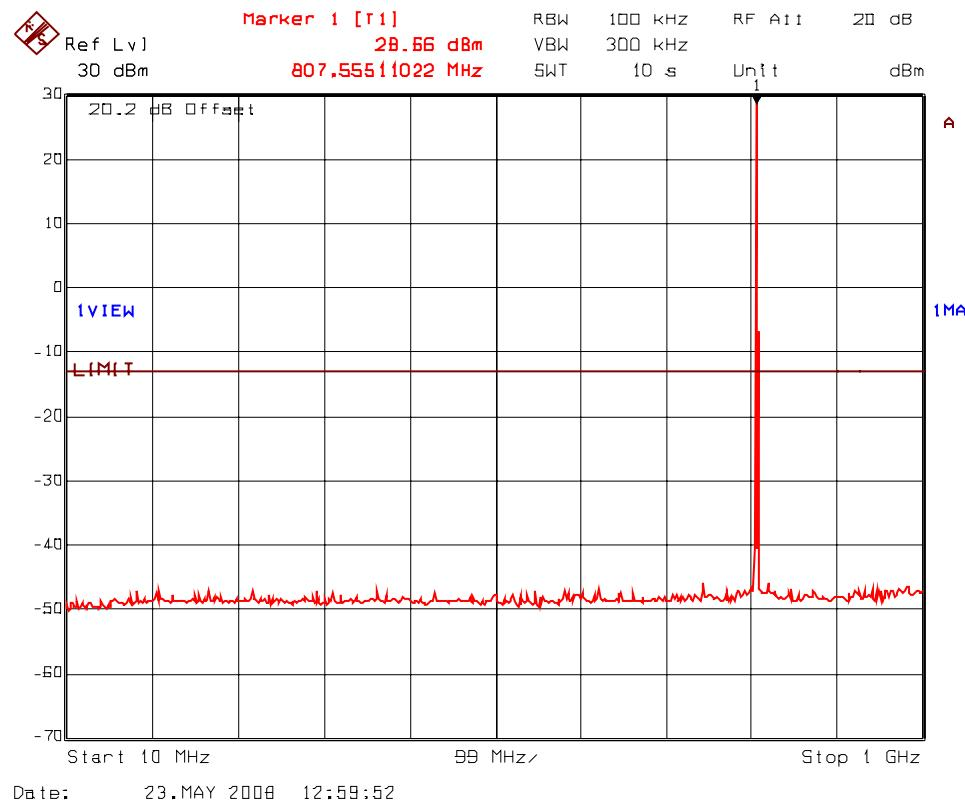
**PLOT # 54(b) Transmitter Antenna Conducted RF Spurious Emissions @ Antenna Port
