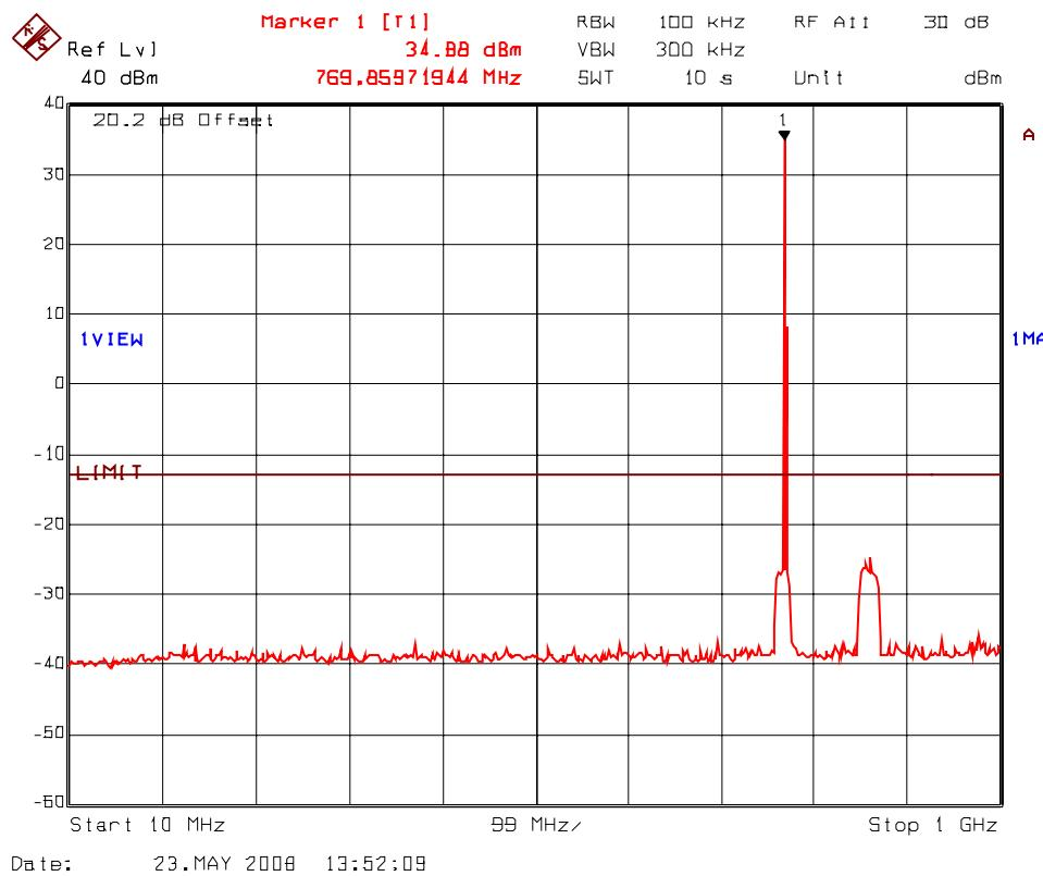
**PLOT # 42(b) Transmitter Antenna Conducted RF Spurious Emissions @ Antenna Port
