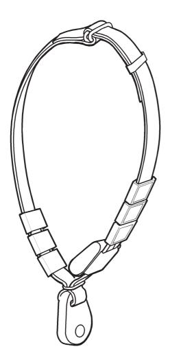
The Activity Tag shall be mounted on the "inside" of the neckband as the figure to the left shows. Note that the thickest part of the tag shall point downward.
