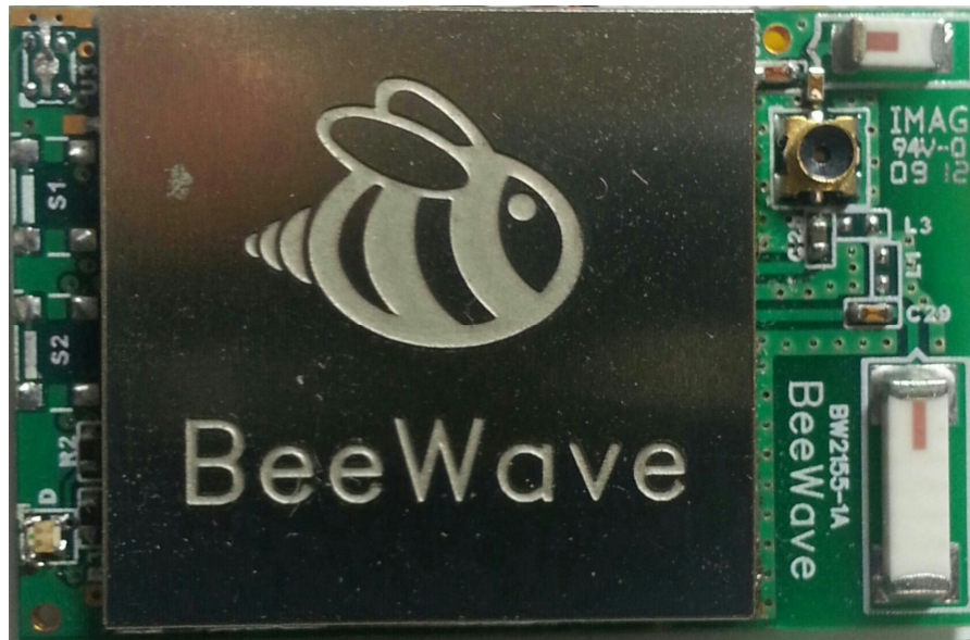
BW2155B Top View with Shield
