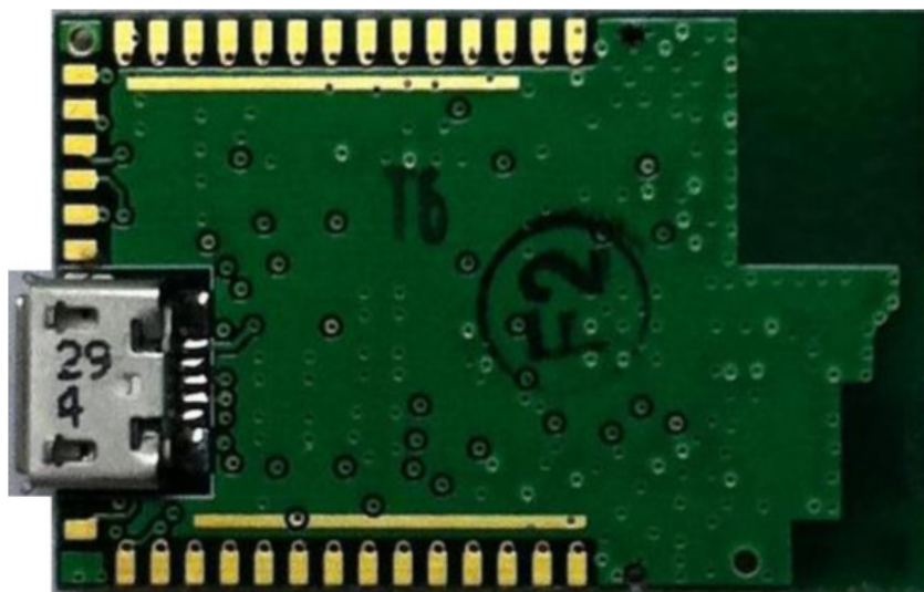
BW2155A Bottom View showing the \mu USB connector
