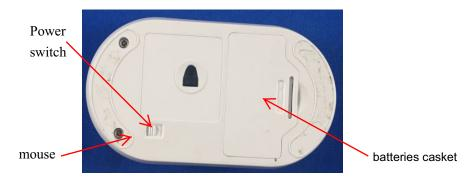
b. Put the batteries into the batteries casket, lock the cover.
