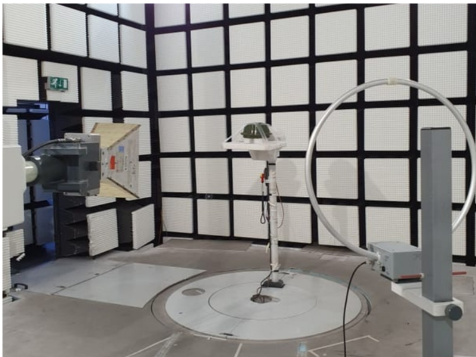
Photo 4: Setup Shielded fully anechoic chamber
