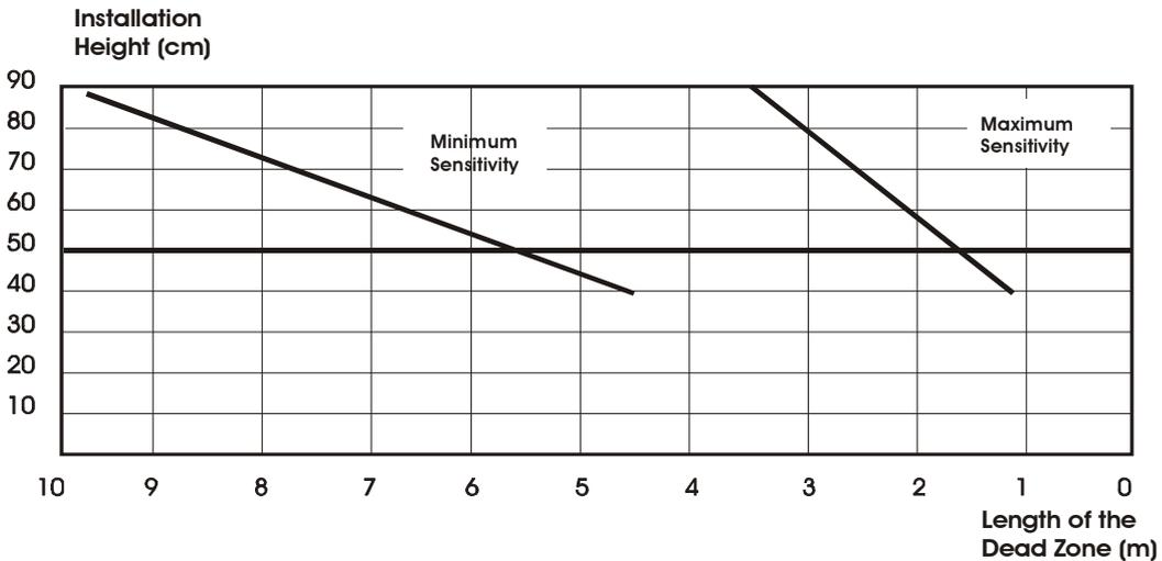
Figure 6 ERMOx 482. 80-120-200: Dead zone length near the equipment versus installation height.
