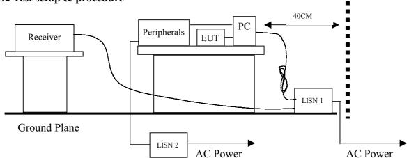
The EUT are connected to the main power through a line impedance stabilization network (LISN). This provides a 50 ohm/50uH coupling impedance for the measuring equipment. The peripheral devices are also connected to the main power through a LISN that provides a 50ohm/50uH coupling impedance with 50ohm termination.
