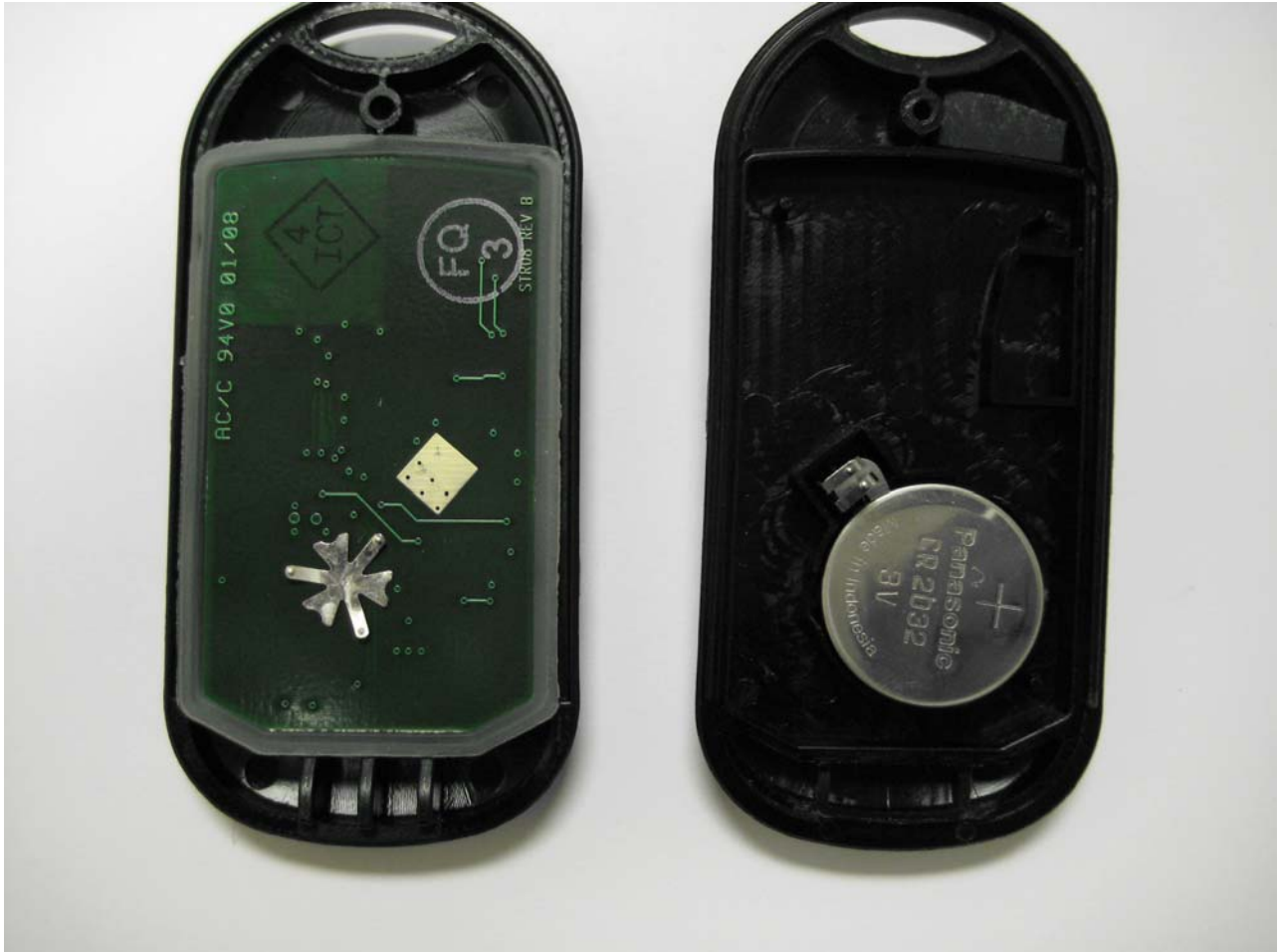
View #3 – Open for Inspection, showing backside of RF Section and Battery Compartment
