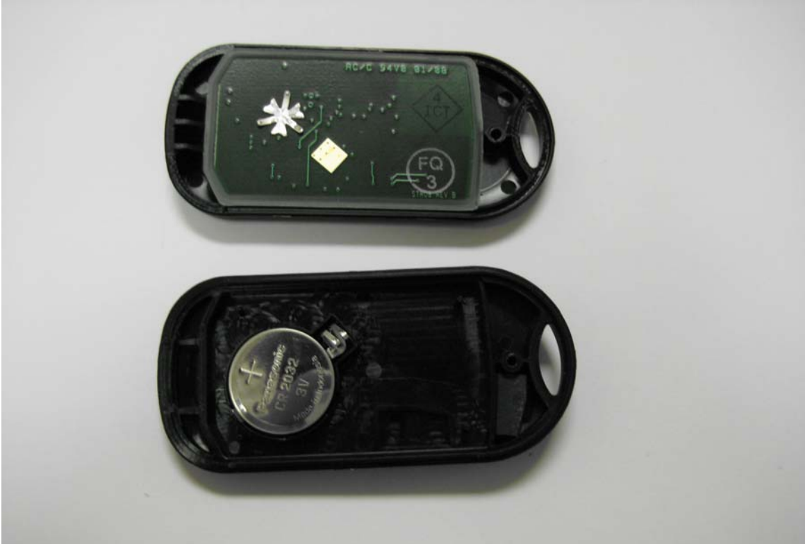
View #4 – Open for Inspection, showing backside of RF Section and Battery Compartment
