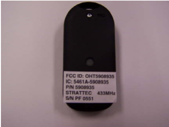
Picture 1: Back of Passive Key Fob
