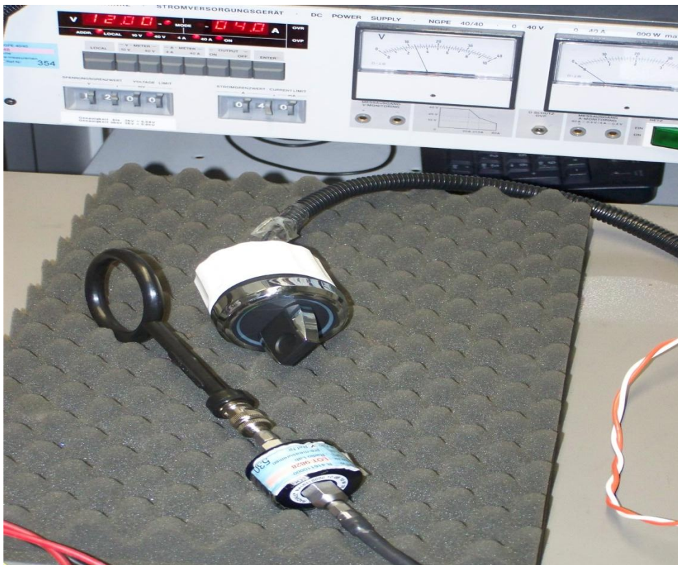
Set-up: Occupied bandwidth measurement
