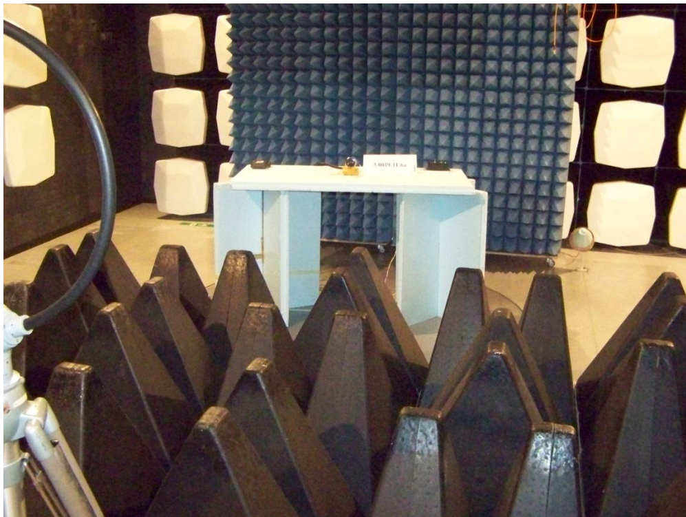
EMI radiated measurements up to 30 MHz (anechoic-room with mobile-floor absorbers)
