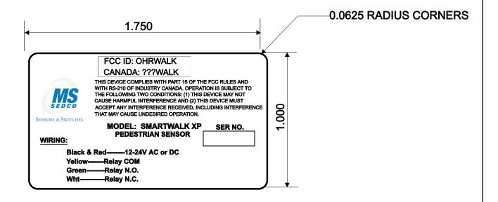
MATERIAL IS 0.003 THICK KIMDURA WITH SELF ADHESIVE BACKING (WITH NO LAMINATION)
