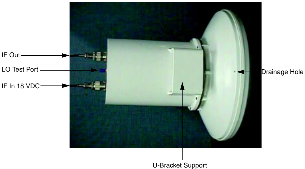
Figure 1-12 CTR 38 GHz Bottom View with Bracket
