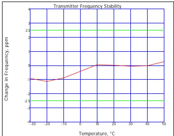
Temperature Stability for 12.50kHz Modulation
