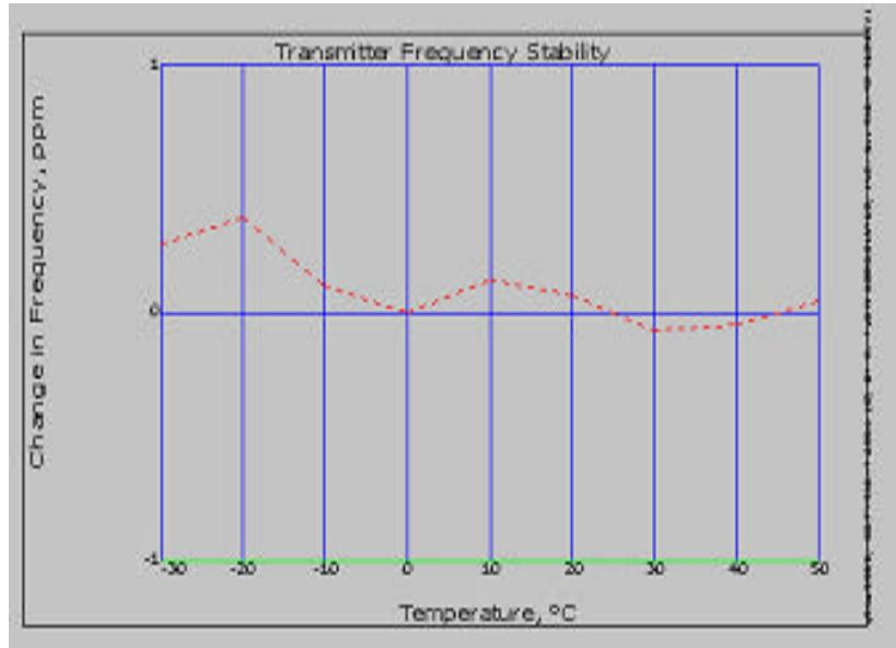
Temperature Stability for 6.25kHz Modulation
