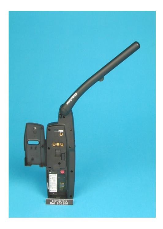
Photograph Three: Rear view of Ericsson Jekyll submitted for testing with antenna in deployed position and connector blanking panel removed.
