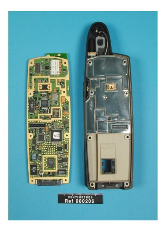
Photograph Five: Underside of main pcb of Ericsson Jekyll showing SIM interface and RF sections.
