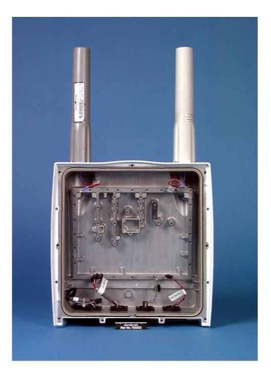
Figure Four: Rear view of Ericsson FAU200 SAT with back panel and PCB removed showing inside of case.
