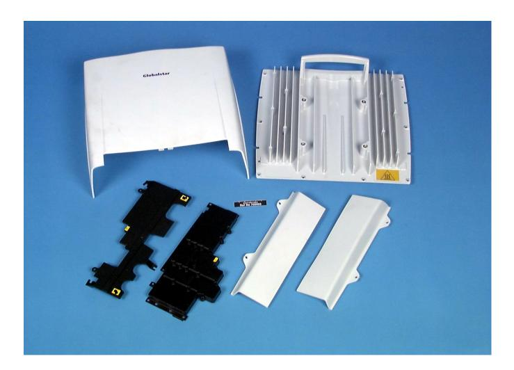
Figure Eight: Ericsson FAU200 SAT external and internal casings (Side 1).
