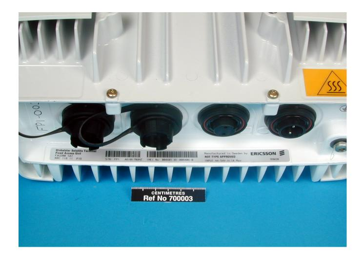
Figure Three: Underside of Ericsson FAU200 SAT showing connectors and labelling.
