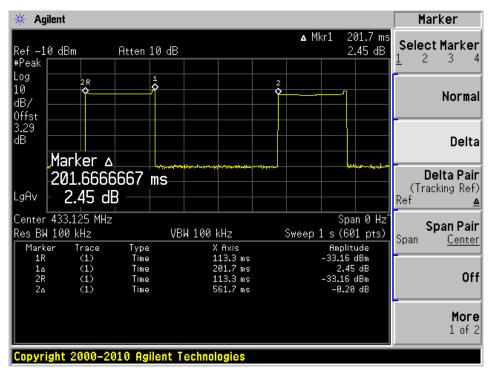
Duty Cycle Correction Factor =  $20*\log(\text{Ton/Tp}) = 20*\log(201.7/561.7) = -8.9$
