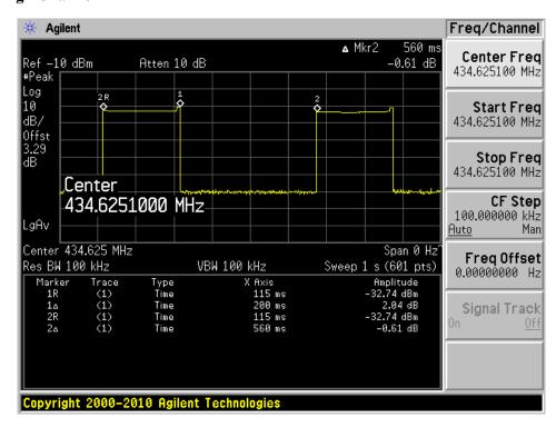
Duty Cycle Correction Factor =  $20*\log(\text{Ton/Tp}) = 20*\log(200/560) = -8.9$
