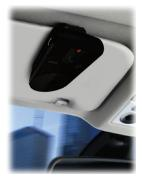
When installed, the Power button must be facing toward you as shown.
