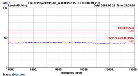
: 03CH06-HY Site FCC CLASS-B 3m HF-HORN AH-118 HORIZONTAL Condition
