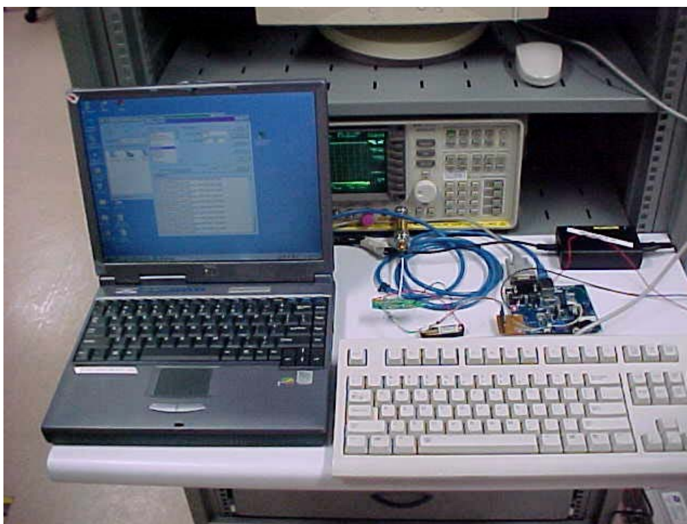
Maximum Peak Power Measurement Test Setup
