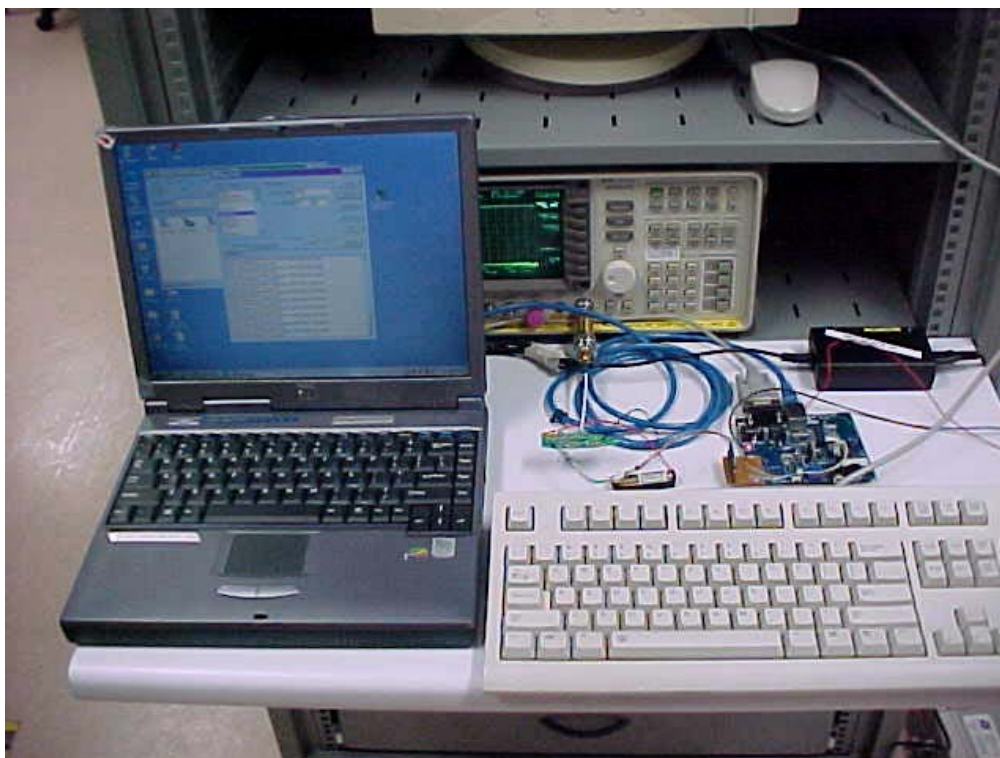
Carrier Frequency Separation Measurement Test Setup
