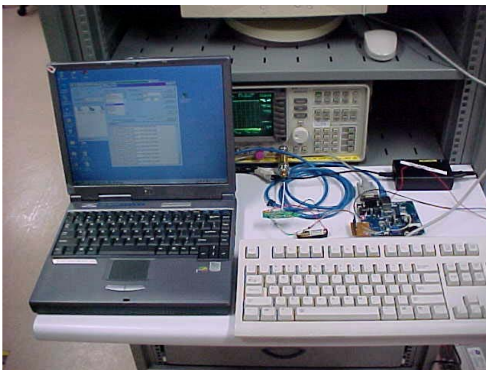
RF Conducted Spurious & Band Edge Measurement Test Setup
