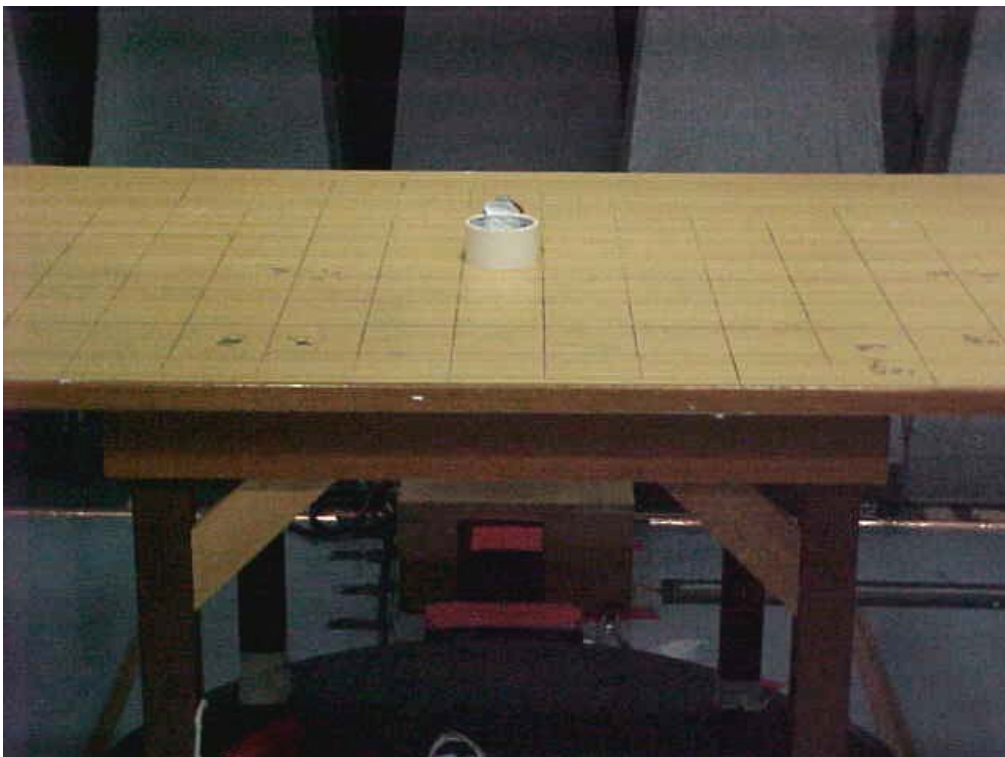
Radiated Emissions Setup (Rear View)
