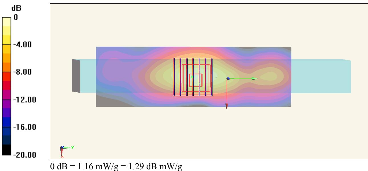
**#05\_WLAN2.4G\_802.11b 1Mbps\_Curved suface of Edge 2\_0cm\_Ch6****DUT: 340236**
