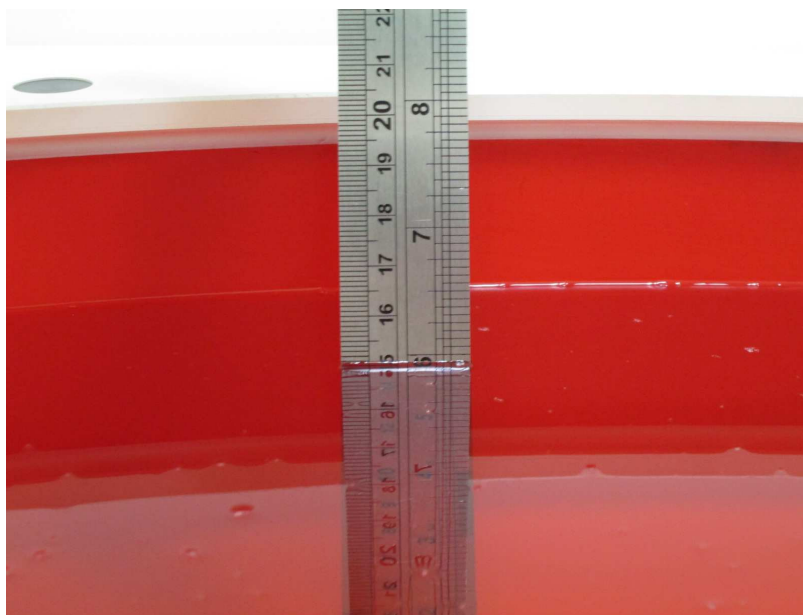
Fig 8.2 Photo of Liquid Height for Body Frequency 1900MHz
