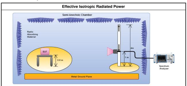
Electric field tests shall be performed in the frequency range of 30 MHz to 1000 MHz using a calibrated bi-log antenna and the frequency range of 1 GHz to 40 GHz using a calibrated horn antenna.
