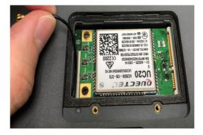
6. Attach the antenna cable to the MAIN connector of the LTE module
