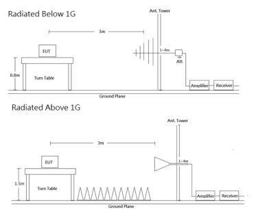
Radiated emission tests were performed in the 3 meters chamber test site, using the setup accordance with the ANSI C63.10-2013. The specification used was the FCC Part 15.209 and FCC 15.247 Limits.
