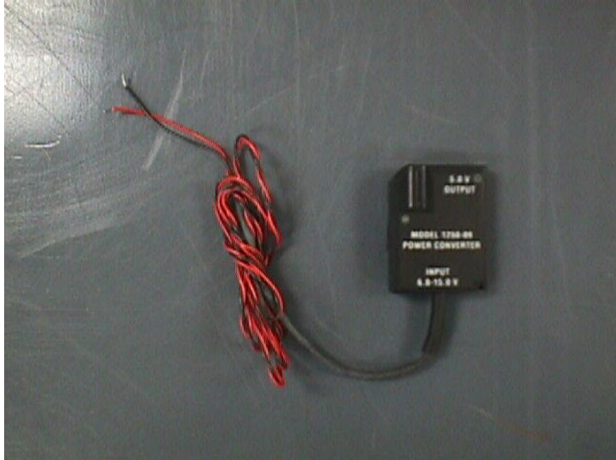
Figure 20: Power Converter M/N 1250-09 top view
