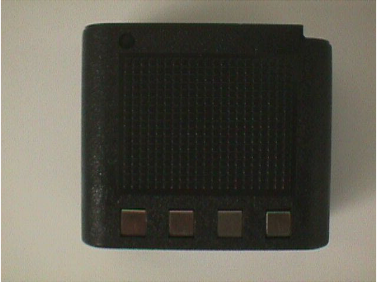
D27: BATTERY CONNECTIONS FOR EXTERNAL CHARGER
