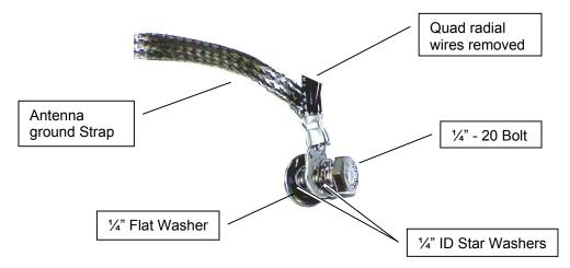
6. Put a 1/4" inside diameter (ID) star washer, and then a 1/4" ID flat washer on one of the 1/4" - 20 x 1" bolts. On the other bolt, place a 1/4" ID star washer, and then the QRT terminal. Place the bolts through the antenna base mount and thread the bolts into the rivnuts. Do Not tighten the bolts until you have attached the upper support bracket and aligned the antenna base mount with the upper support bracket.
