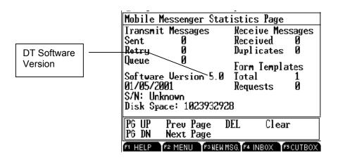
Next, determine the ITU software version. Press the **F2** key and then the **7** key, and the *ITU* Statistics Page – Transmitter page appears. Press the **YELLOW + PAGE DOWN** keys and the *ITU Statistics Page – Receiver* page appears. The ITU software version is listed in the lower left corner of the message box.
