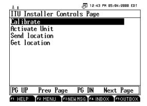
A calibration box appears with the **CALIBRATE** button highlighted. Wait until the question mark is replaced with an initial calibration value, and then press the **ENTER** key. The system begins the calibration process and continues until complete. This may take several minutes for ITUs versions 7.2 or higher, and 5-6 minutes for versions below 7.2. The user is unable to perform any other DT actions while the system calibrates.
