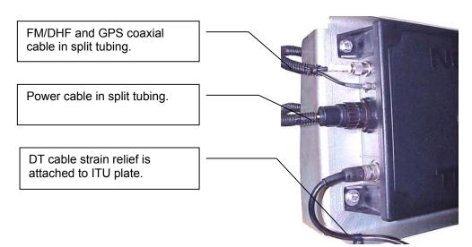
6. Attach strain relief. Place a strain relief on the DT cable and screw it directly to the ITU pedestal.
