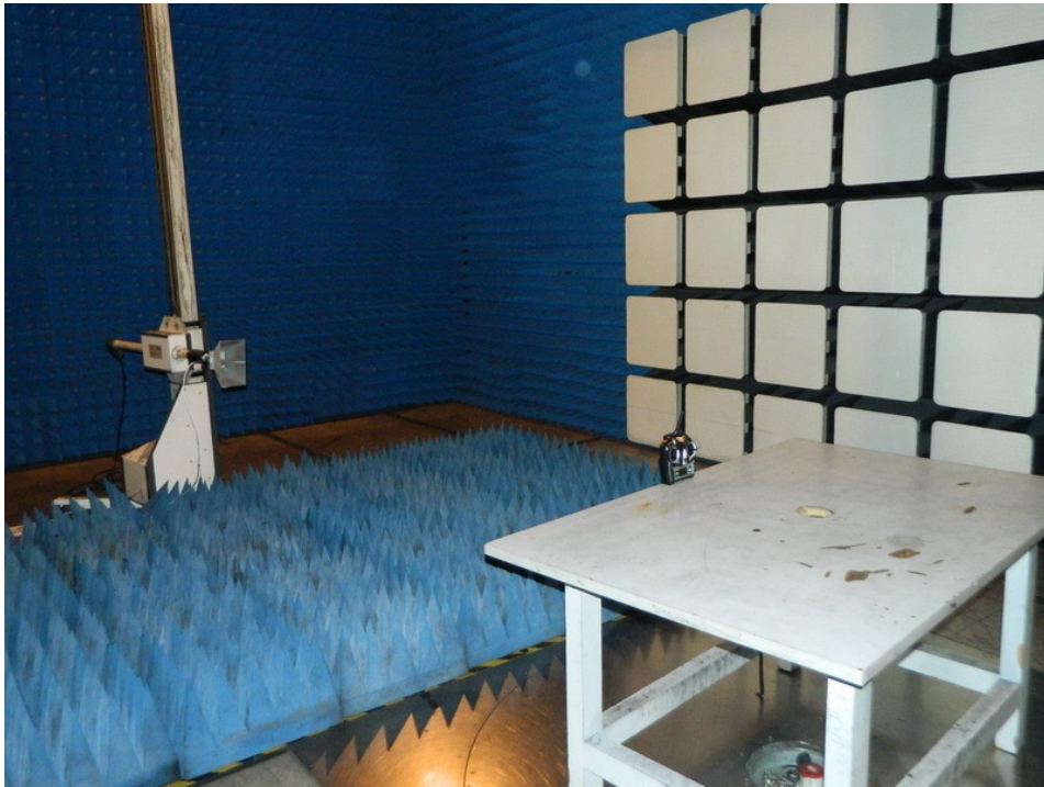
Setup for radiated emission
